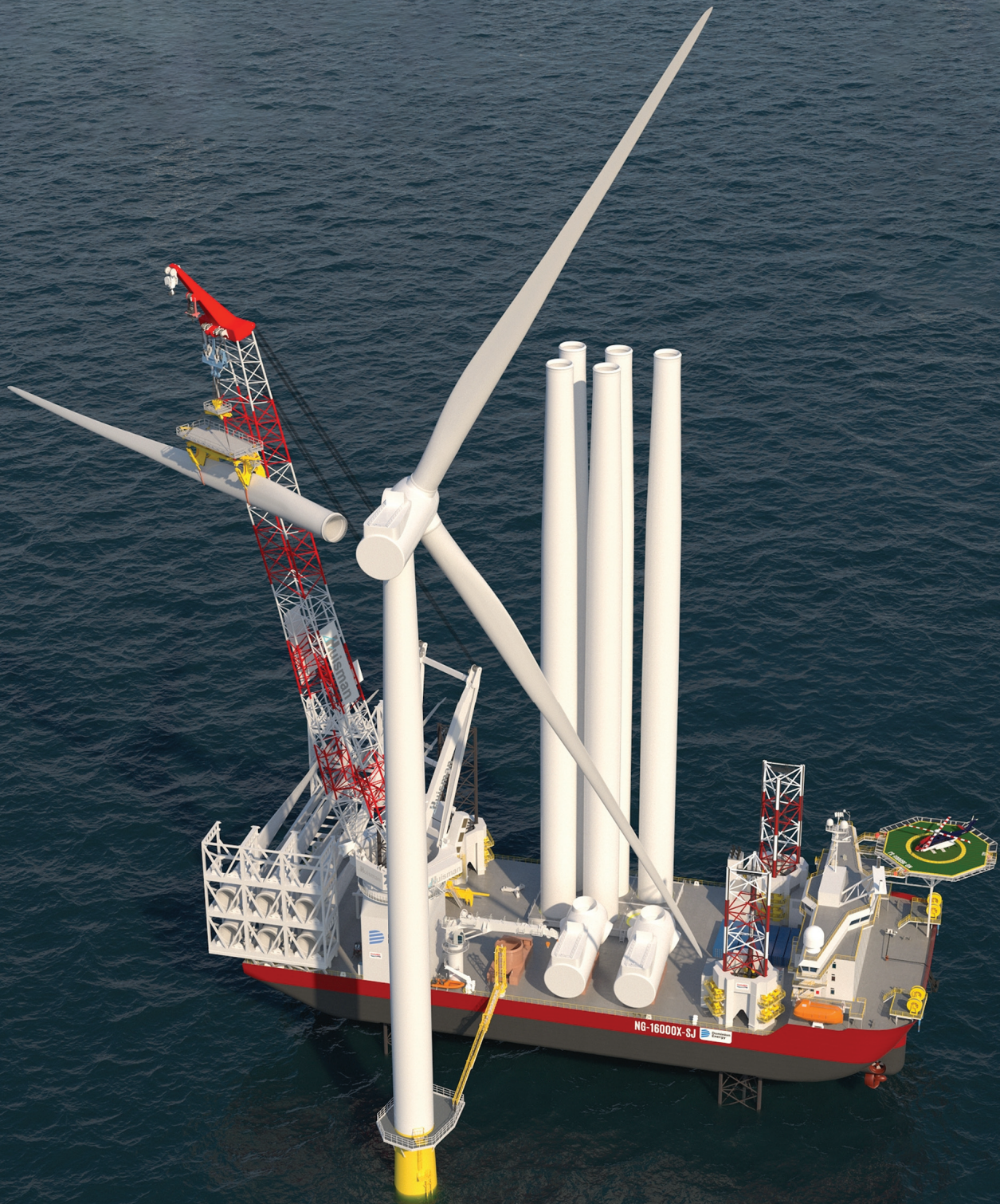
↑ Rendering of the first American-made offshore wind turbine installation vessel
