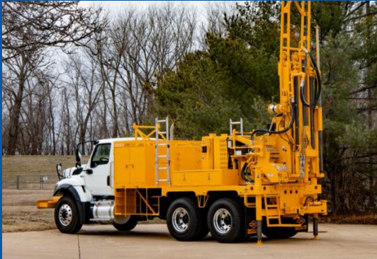
TRUCK-MOUNTED DRILL RIG
