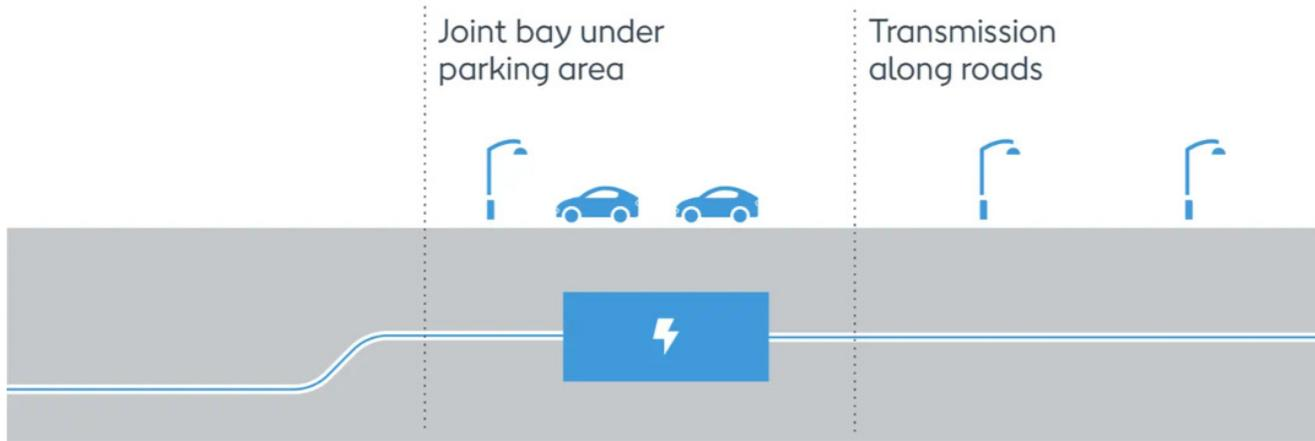
The site of the drilling pit becomes the home of the transition joint bay. This is an underground concrete box where the cable from under the beach joins a cable leading to the onshore substation further inland.
