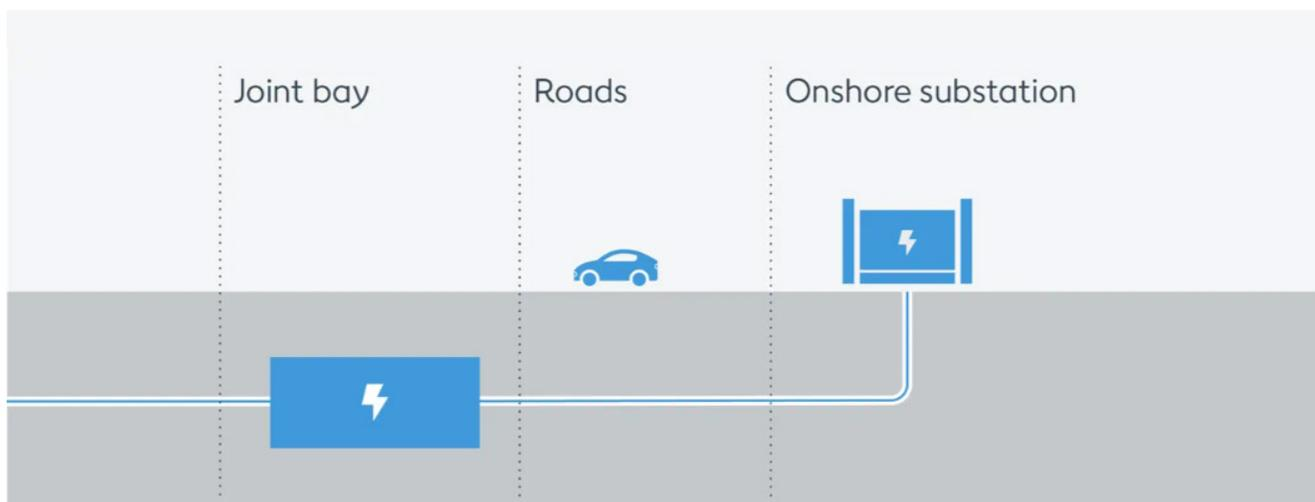
From the transition joint bay, a cable runs underground to a substation. Depending on the location of the substation, the underground transmission line could be several miles long. Like other utility pipes and cables, it tends to run lengthways underneath a road.
