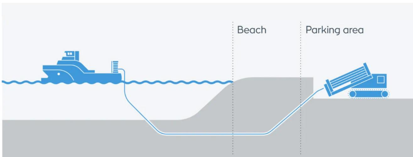
The first stage of making landfall is for a cable to run from the seafloor to a location a short distance inland. To put this cable in place, a hole is drilled using a technique called horizontal directional drilling.
