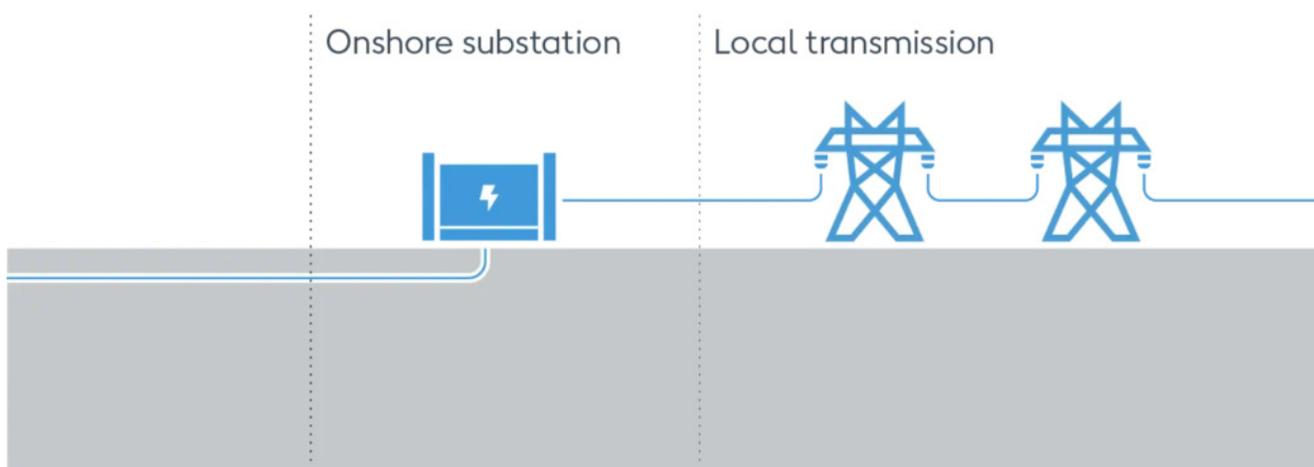
The final stage in getting renewable power from the offshore wind farm to the distribution grid is the substation. This is where the physical connection is located, and where the current is converted to the right voltage and frequency to be fed into the grid.
