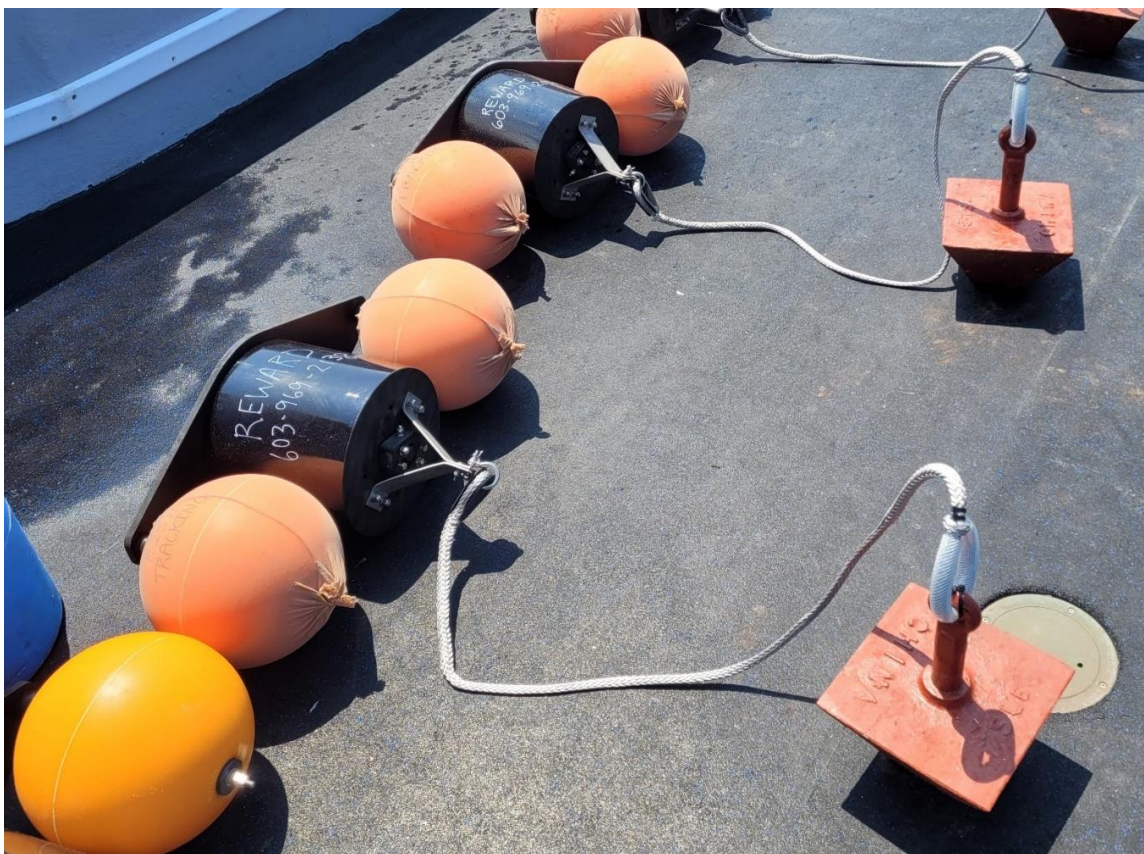
Figure 2 – Mooring configuration used to deploy VEMCO VR2AR acoustic receivers.
