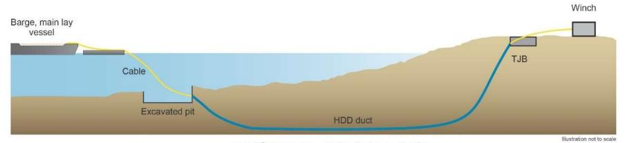
HDD Schematic - with Barge and TJB
