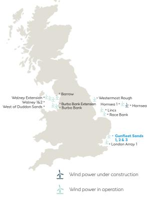
The Gunfleet Sands Offshore Wind Farm is located approximately 7 km (4.3 miles) south-east of Clacton-on-Sea, Essex. The project consists of three phases: Gunfleet Sands 1, with 30 3.6 MW turbines; Gunfleet Sands 2, with 18 3.6 MW turbines; and Gunfleet Sands 3 Demonstration Project which consists of 2 6 MW turbines.
