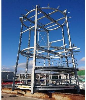
Figure 10 - Internal platform structures for Hornsea 2's offshore wind transition pieces
