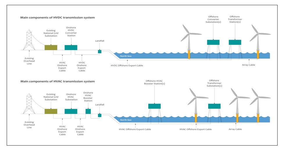
Figure 1.2 Main components of High Voltage Direct Current (HVDC) and High Voltage Alternating Current (HVAC) transmission options for Hornsea Three.
