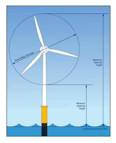
Figure 3.1 Schematic of an offshore wind turbine.
