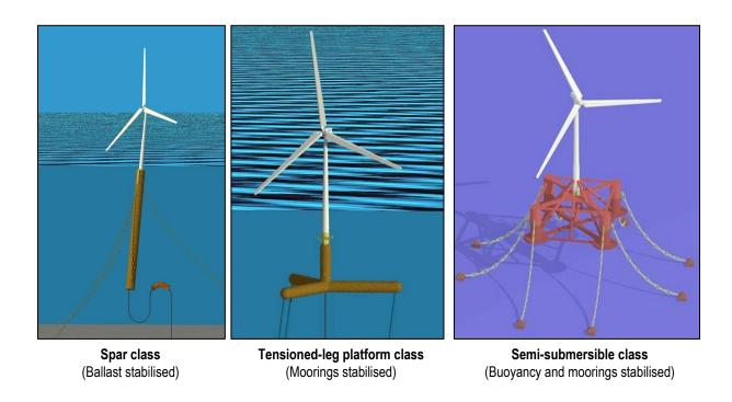
Figure 3.6 Examples of floating foundations.
