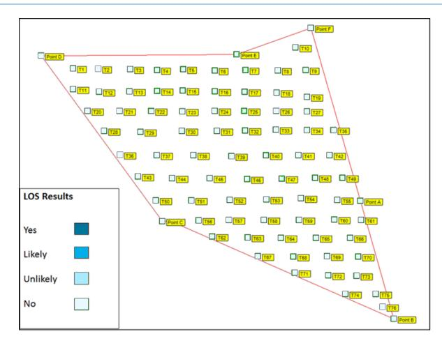
Figure 5.1: LOS Results from NATS Claxby PSR at a turbine tip height of 325 m.
