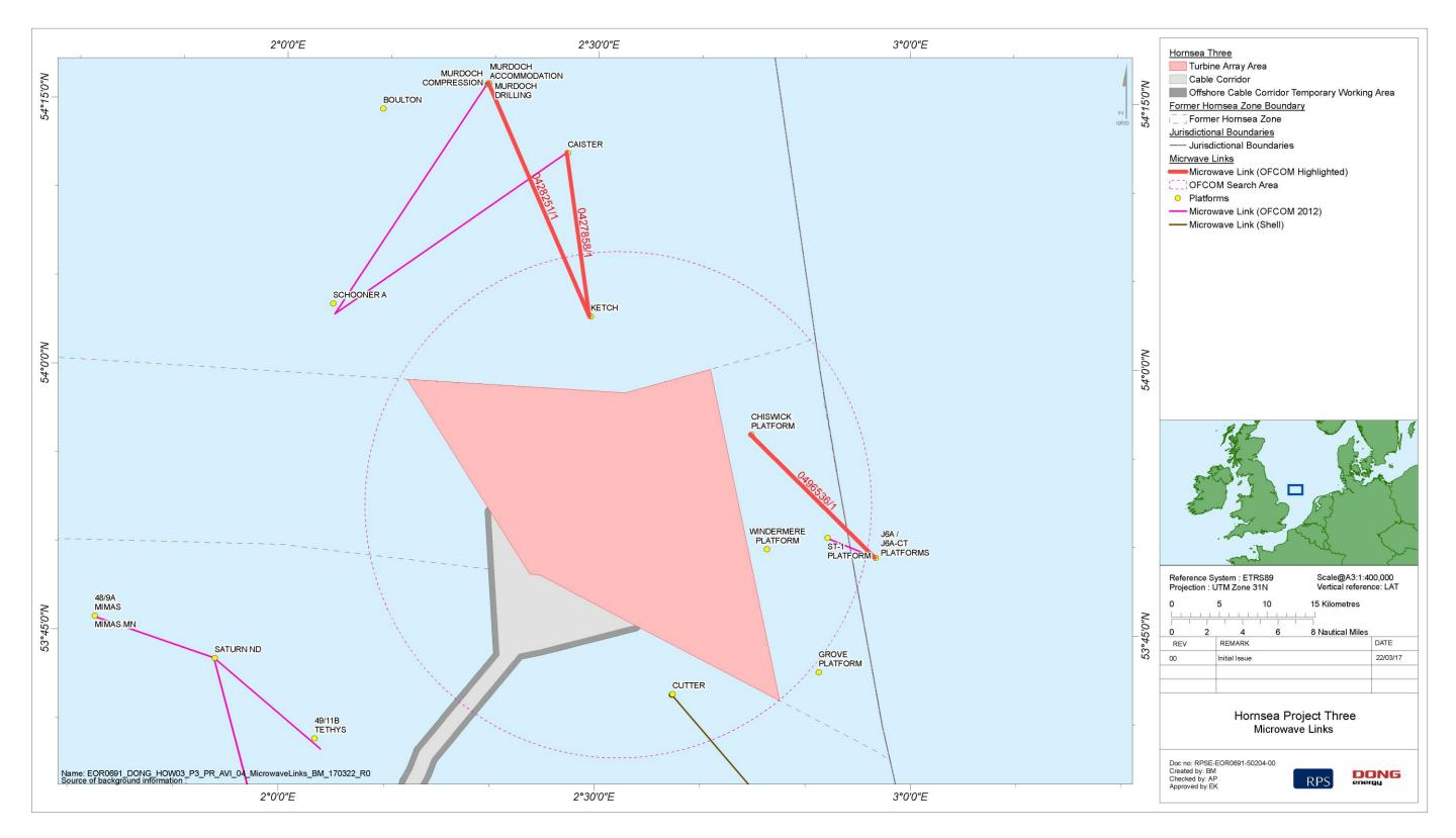
Figure 8.1: Microwave fixed links within 26.5 km of the centre of the Hornsea Three array area.
