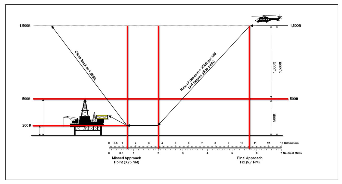
Figure 7.4: Indicative instrument approach procedure without turbines present.
