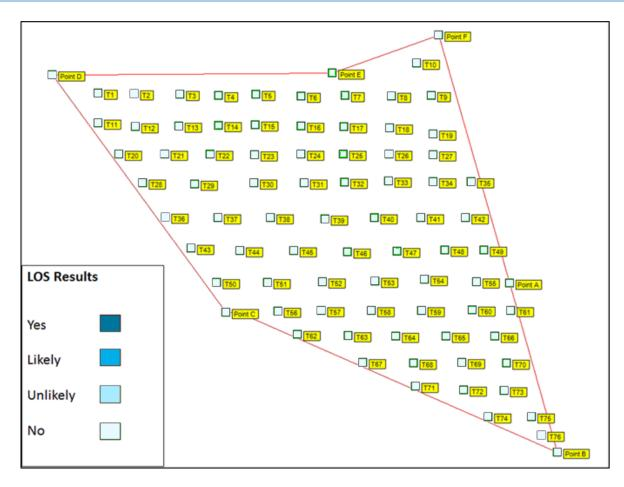
Figure 6.1: LOS results from MOD Staxton Wold ADR at a turbine tip height of 325 m.
