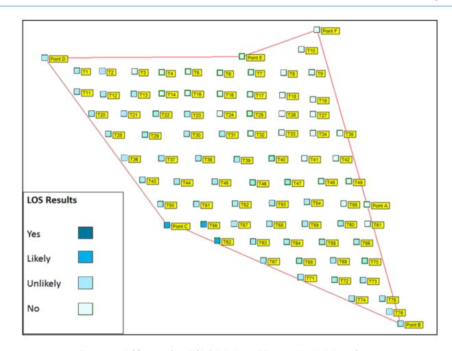
Figure 6.2: LOS results from MOD Trimingham ADR at a turbine tip height of 325 m.
