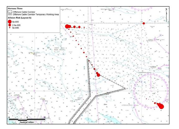
Figure 18.8: Annual powered vessel to structure allision frequency by structure.
