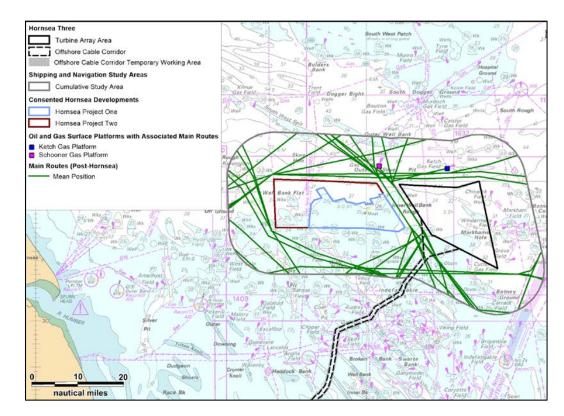
Figure 18.12: Post-Hornsea Three, Hornsea Project One and Hornsea Project Two main routes within the Hornsea Three cumulative shipping and navigation study area.
