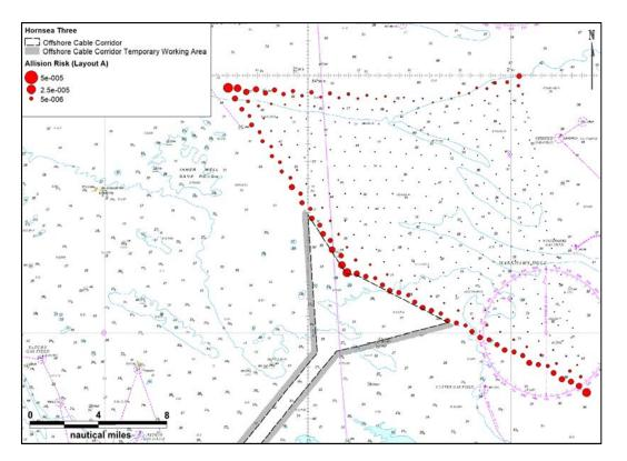
Figure 18.9: Annual NUC vessel to structure allision frequency.
