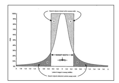
Figure C.5: Sweep width versus probability of detection.
