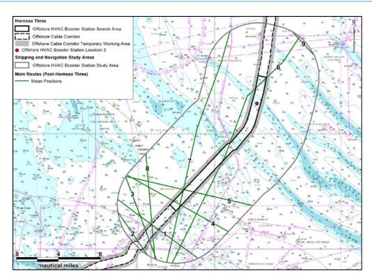
Figure 18.17: Post-Hornsea Three main routes within offshore HVAC booster station shipping and navigation study area for Location 3.
