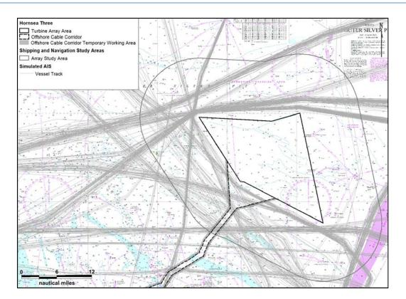
Figure 18.7: Simulated AIS following installation of Hornsea Three array area (40 days).
