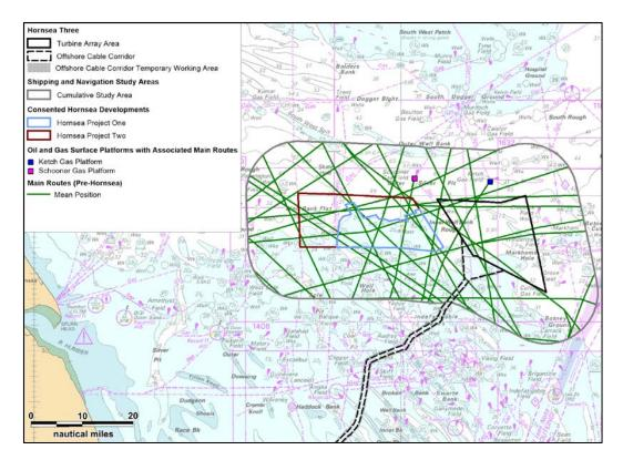
Figure 18.11: Pre-Hornsea Three, Hornsea Project One and Hornsea Project Two main routes within the Hornsea Three cumulative shipping and navigation study area.
