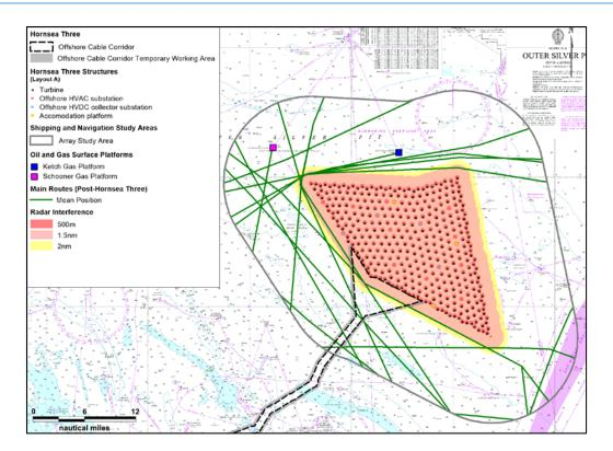
Figure 19.1: Hornsea Three array area (Layout A) Radar interference and post-Hornsea Three routeing.
