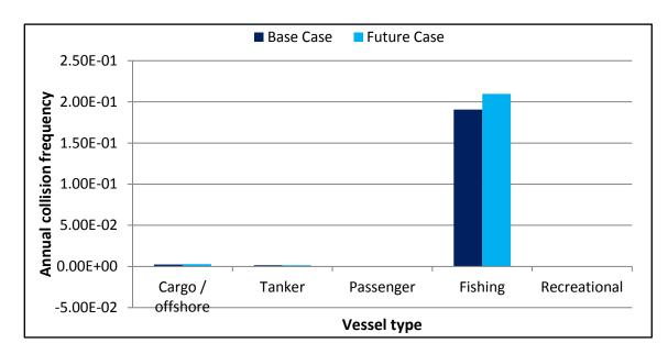
Figure A.16: Change in annual collision frequency by vessel type.
