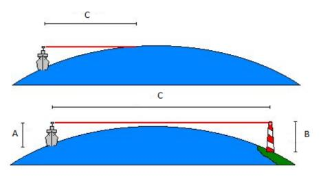
Figure 19.3: Determining Radar range.
