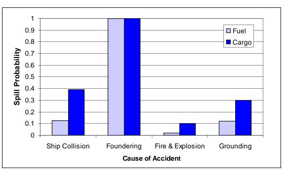
Figure A.22: Probability of an oil spill resulting from an accident.
