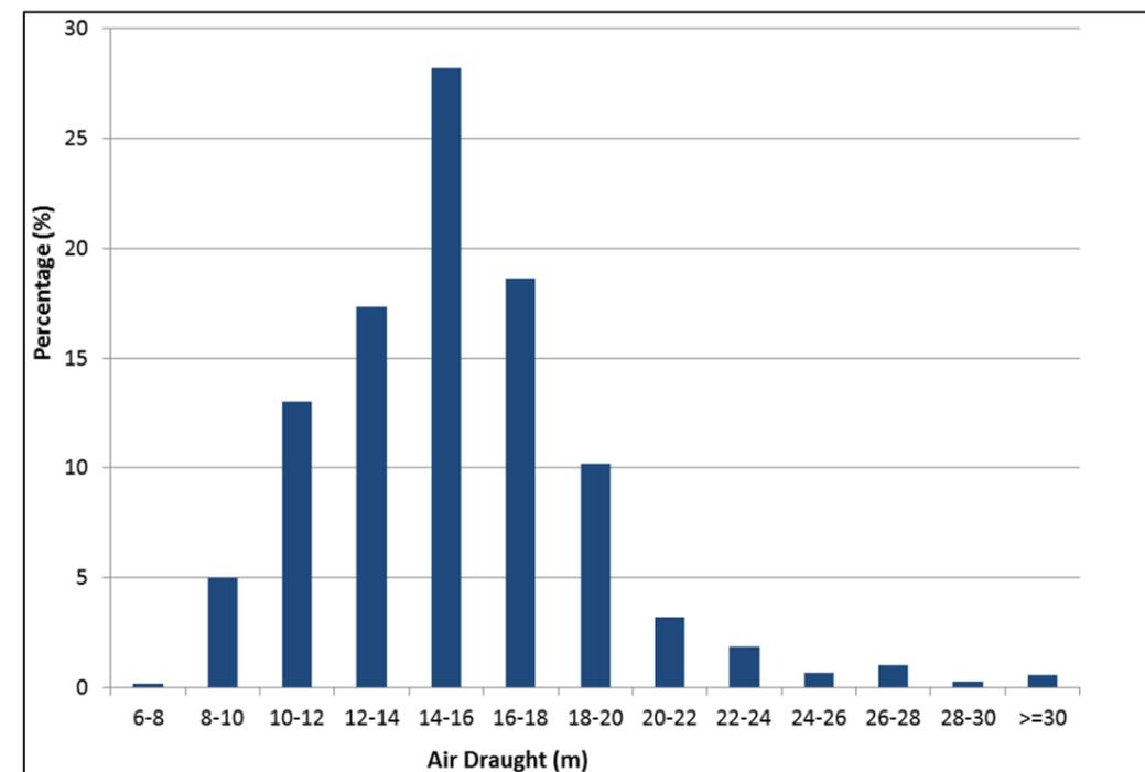
Figure 18.10: Air draught data for IRC fleet (collected 2009 to 2011) (RYA, 2015).
