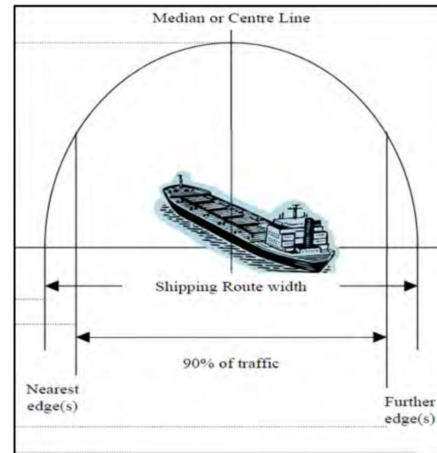
Figure 15.17: Illustration of main route calculation.
