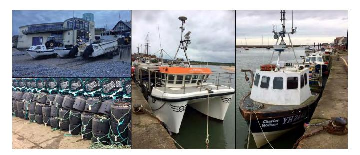
Figure 2.8: Typical inshore potting vessels: top left: beach launched vessels in Cromer; bottom left: plastic whelk pots and crab and lobster pots; centre: catamaran and right: potting vessel moored at Wells-Next-the-Sea (Source: Poseidon).
