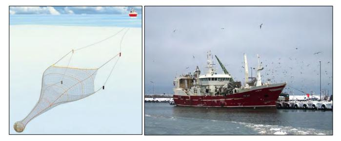
Figure 2.10: Typical pelagic trawl gear (Source: Galbraith *et al.*, 2004) and vessel (Source: Poseidon).
