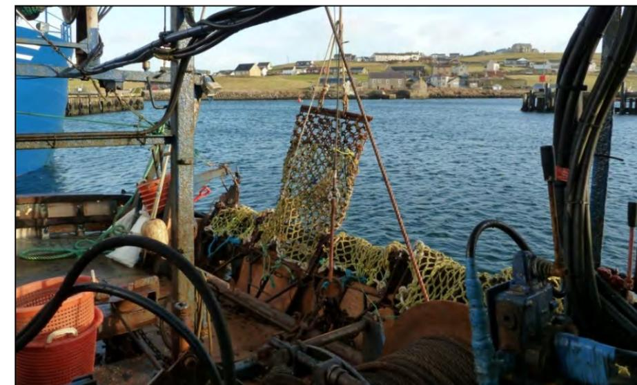
Figure 2.9: Typical scallop dredging vessel (Source: Poseidon).
