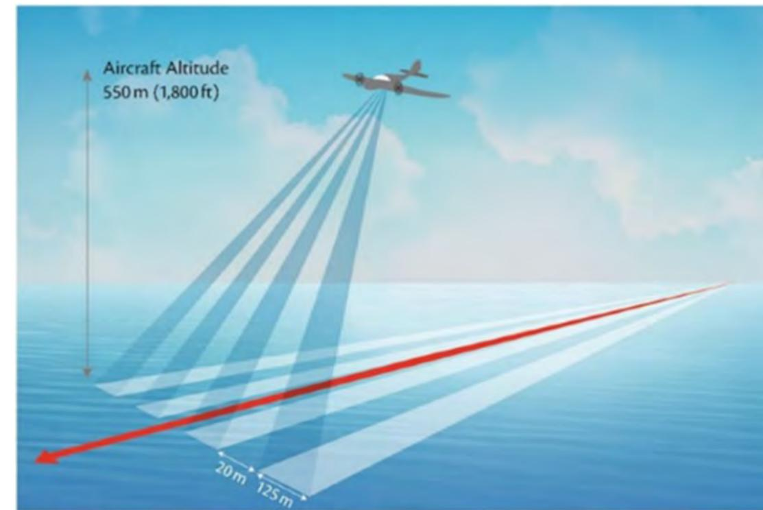
Figure 2.2: Illustration of the survey swathe for HiDef's Gen II camera rig.
