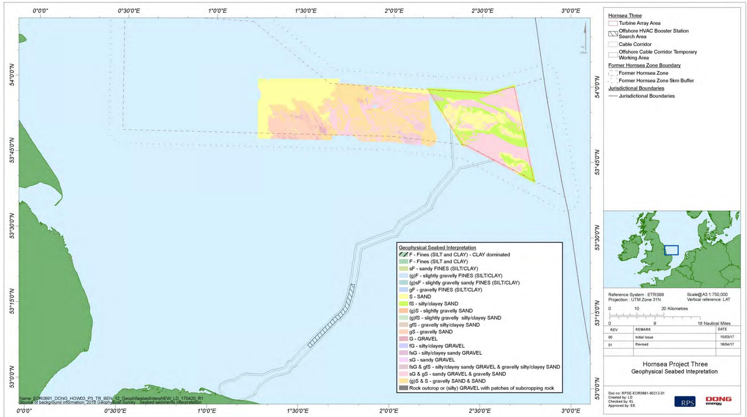
Figure 2.6: Geophysical survey seabed interpretation for the Hornsea Three benthic ecology study area.
