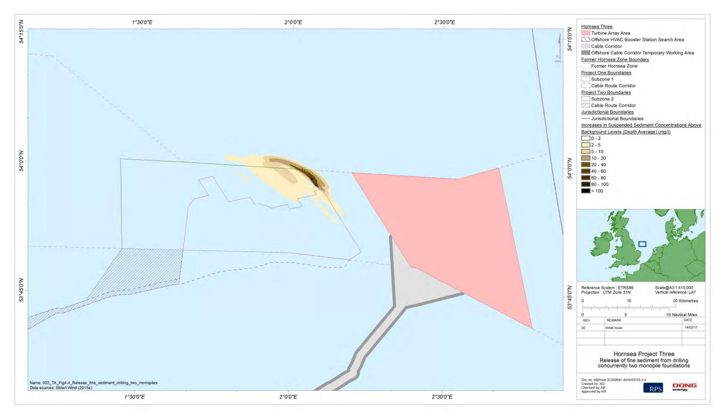
Figure 4.4: Release of fine sediment from drilling concurrently two monopile foundations (reproduced from SMart Wind, 2015a).
