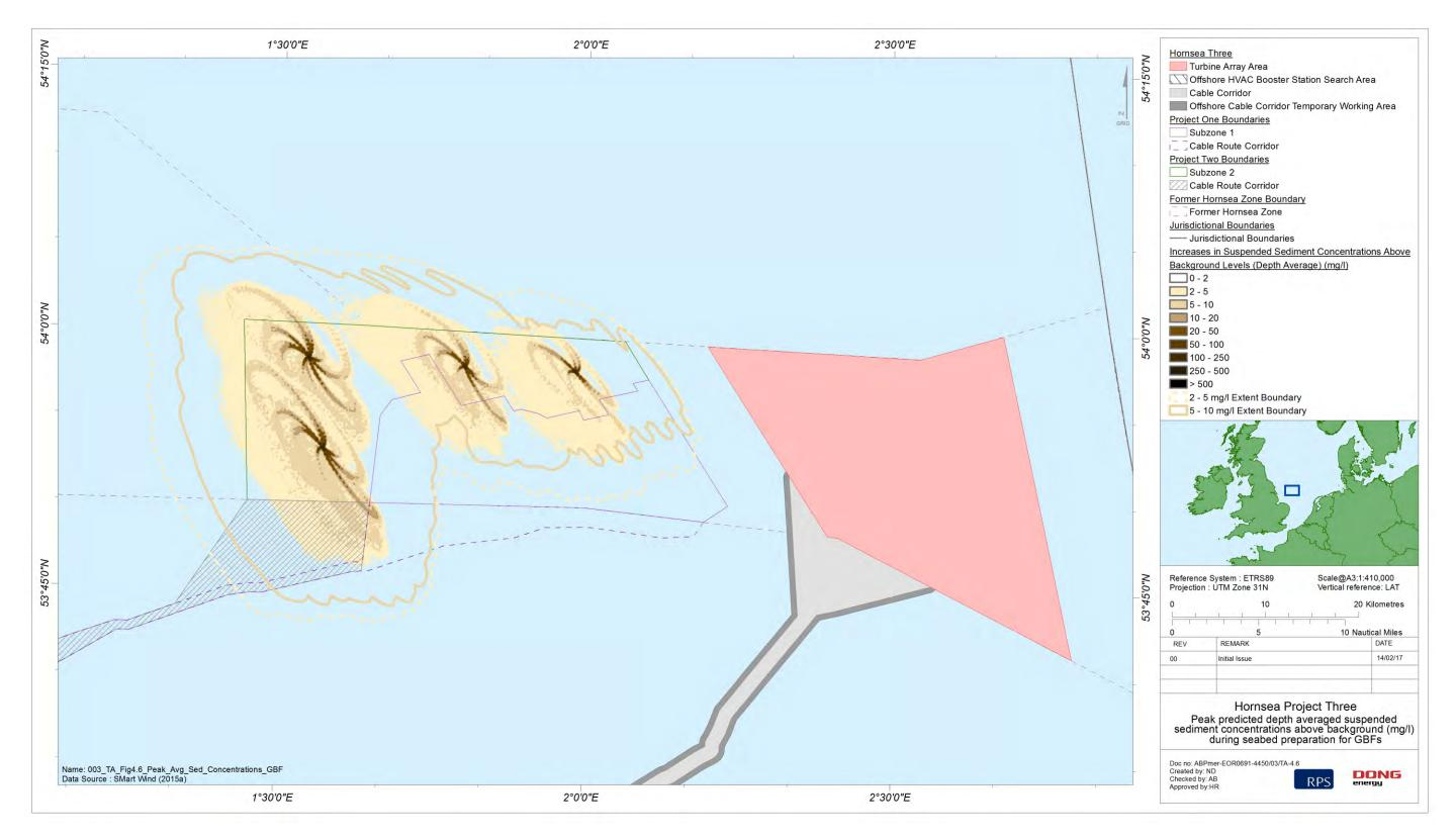
Figure 4.6: Peak predicted depth averaged suspended sediment concentrations above background (mg/l) during seabed preparation for gravity base foundations (reproduced from SMart Wind, 2015a).
