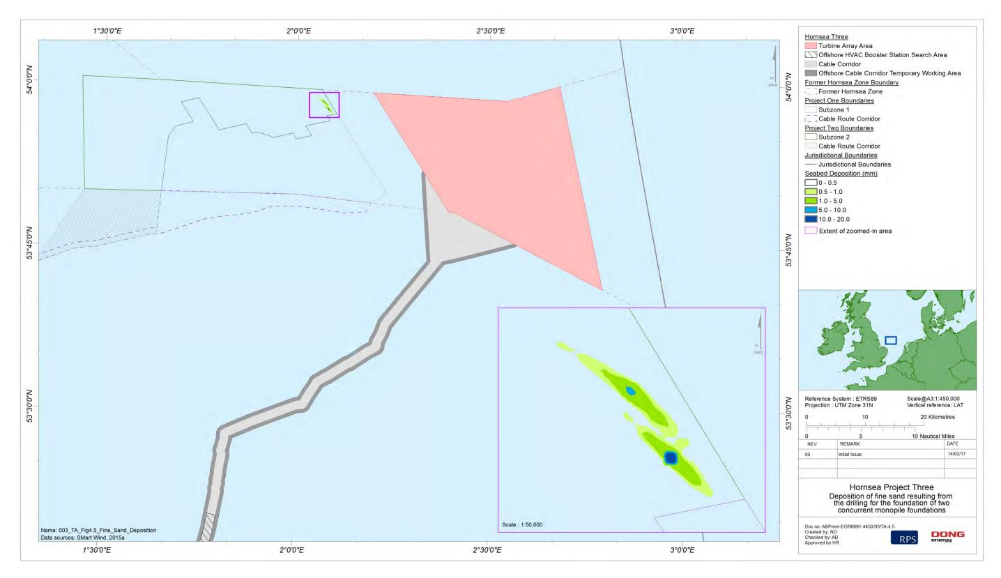
Figure 4.5: Deposition of fine sand resulting from the drilling for the foundation of two concurrent monopile foundations (reproduced from SMart Wind, 2015a).
