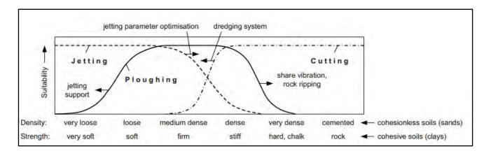
Figure 4.9: Indicative burial tool suitability in different ground conditions (DNV, 2014).
