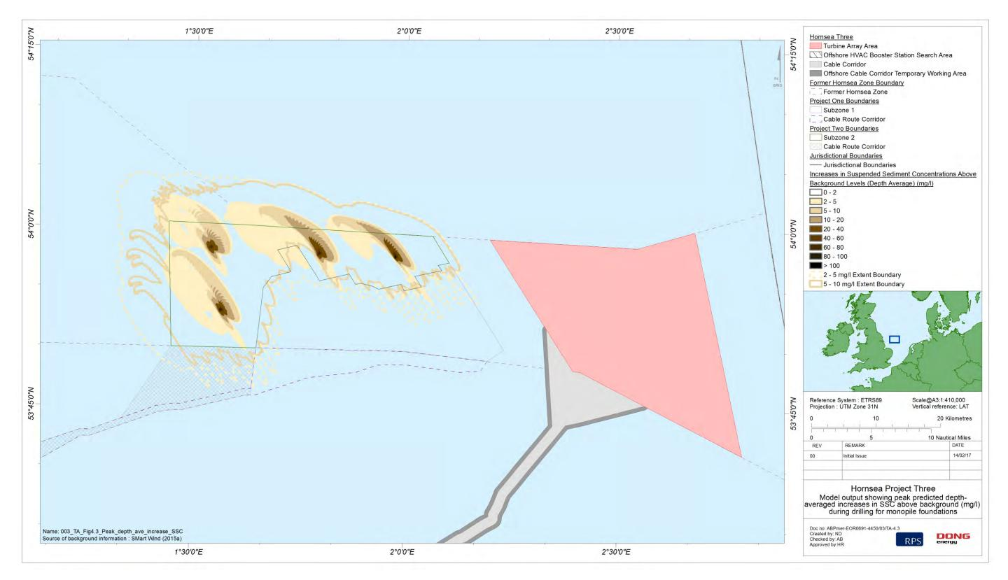
Figure 4.3: Model output showing peak predicted depth-averaged increases in SSC above background (mg/l) during drilling for monopile foundations (reproduced from SMart Wind, 2015a).
