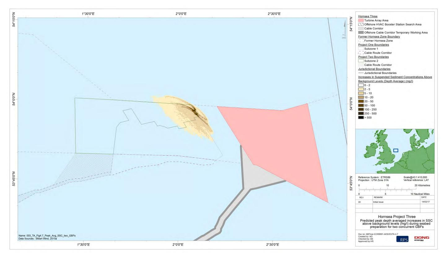
Figure 4.7: Predicted peak depth averaged increases in SSC above background levels (mg/l) during seabed preparation for two concurrent gravity base foundations (reproduced from SMart Wind, 2015a).
