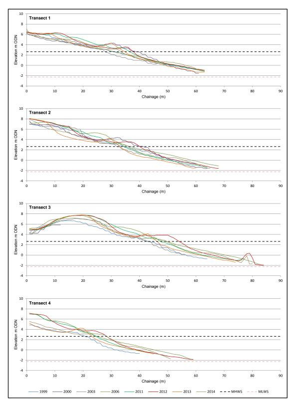
Figure 6.6: Topography (m ODN) along profile transects 1 to 4 during the period 1999 to 2014, based on LiDAR data.
