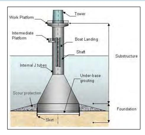
Figure B.3: Outline design of a gravity base foundation (reproduced from SMart Wind, 2015d).
