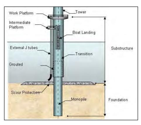
Figure B.1: Outline design of a typical steel monopile foundation (with scour protection) (reproduced from SMart Wind, 2015d).
