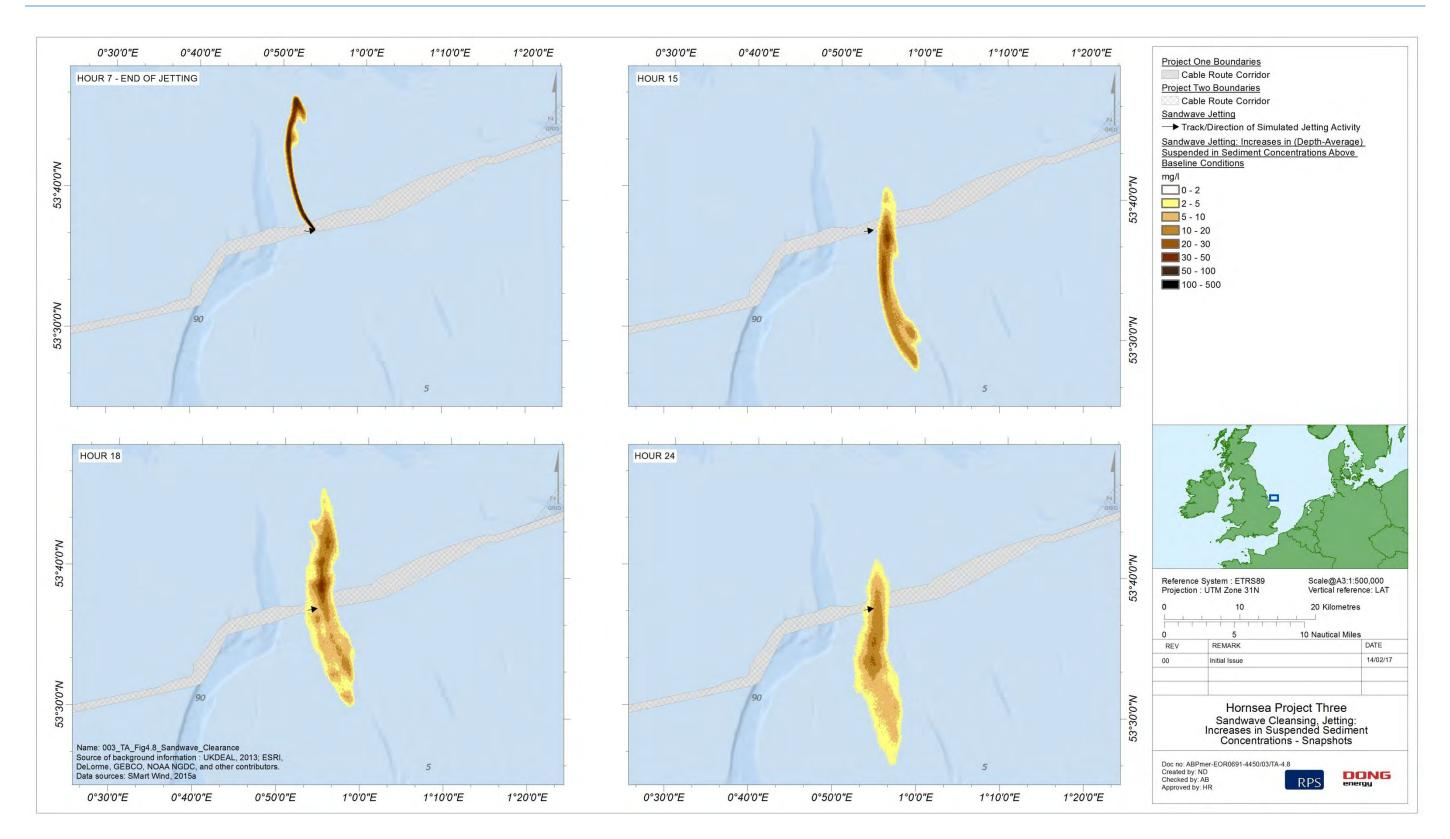
Figure 4.8: Sandwave clearance via mass excavator tool - predicted maximum increases in depth-averaged SSC above background conditions (reproduced from SMart Wind, 2015a).
