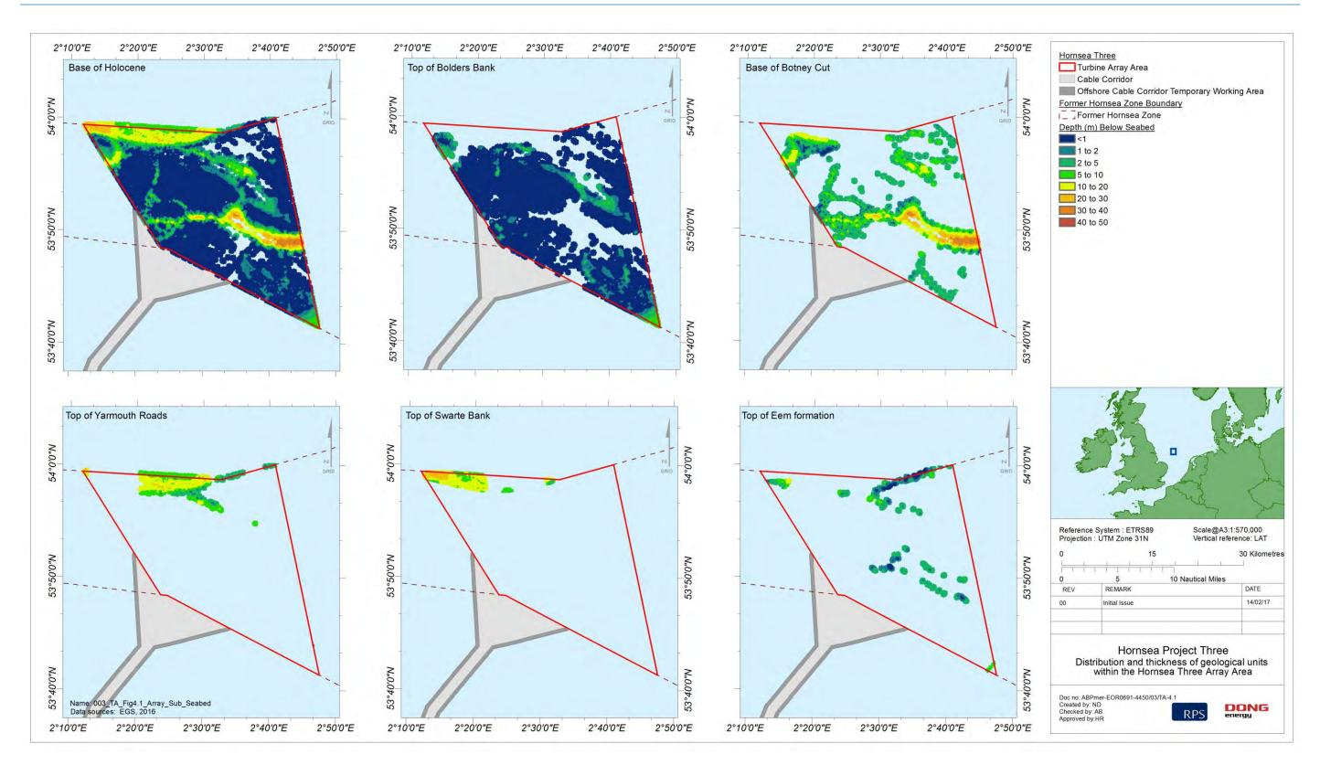
Figure 4.1: Distribution and thickness of geological units within the Hornsea Three array area.
