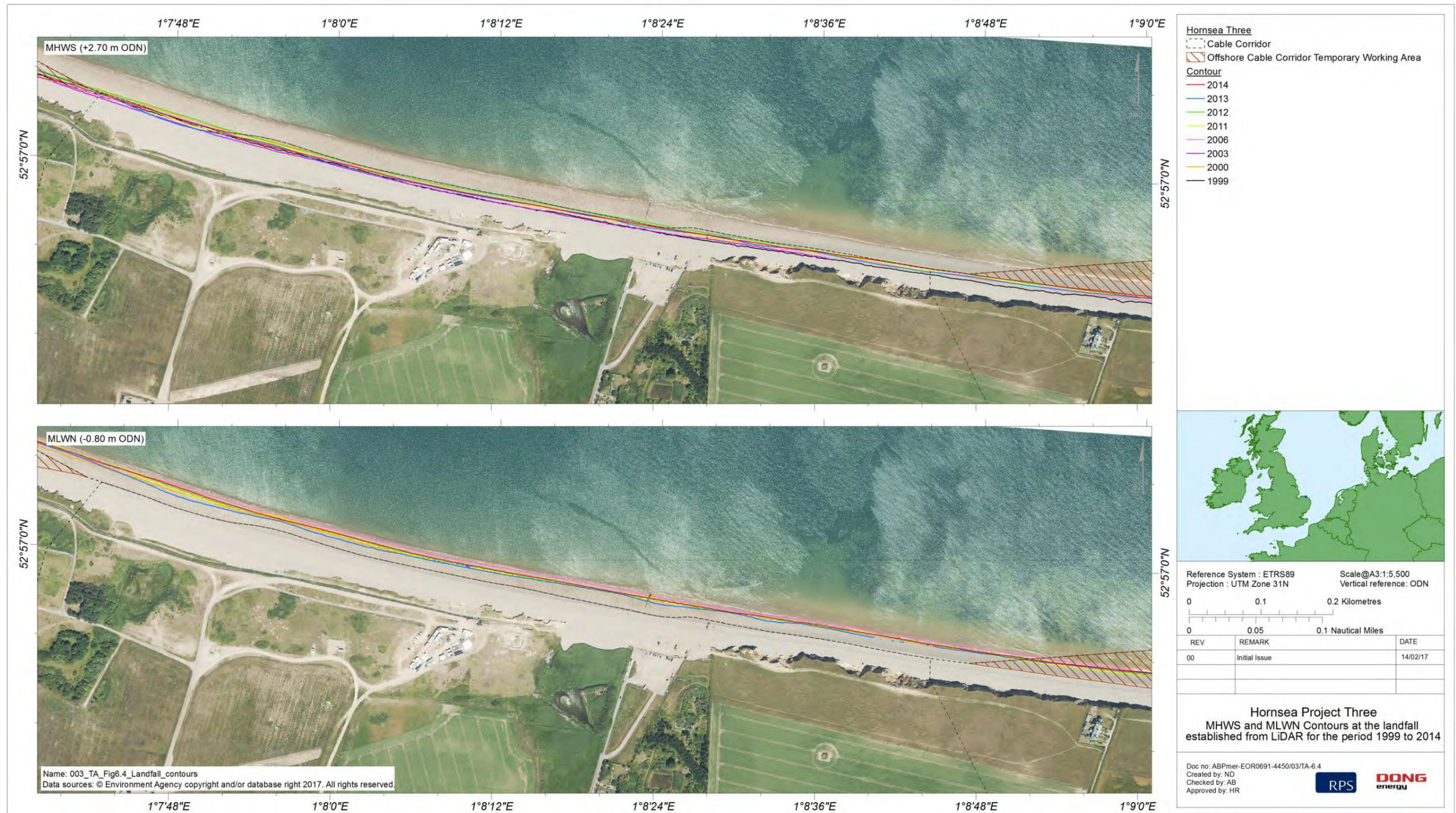
Figure 6.4: MHWS and MLWN contours at the landfall established from LiDAR for the period 1999 to 2014.
