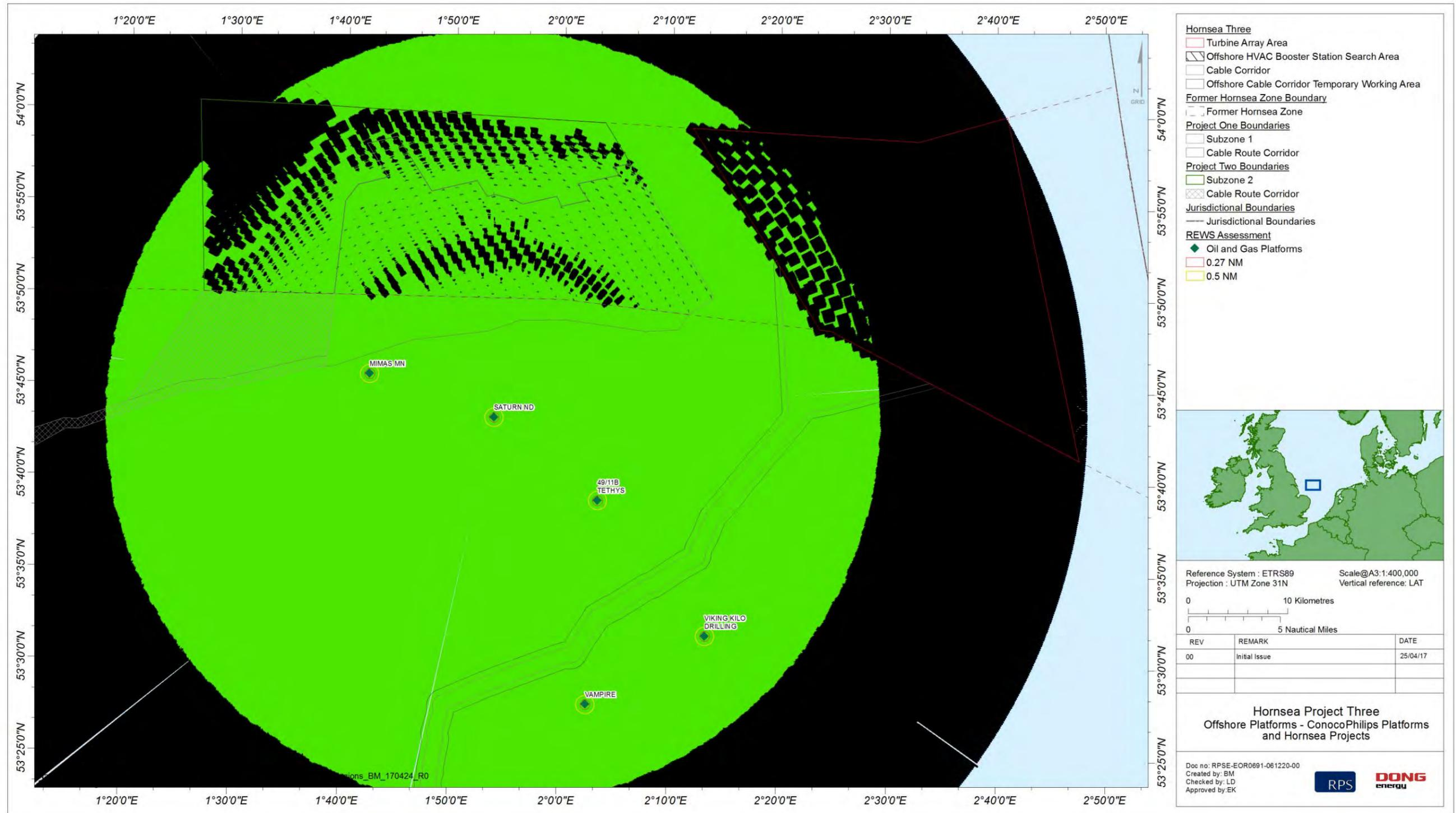
Figure 5.15: Saturn platform REWS detection plot showing loss regions for a large 1,000 m<sup>2</sup> target over the combined Hornsea Project One, Hornsea Project Two and Hornsea Three.
