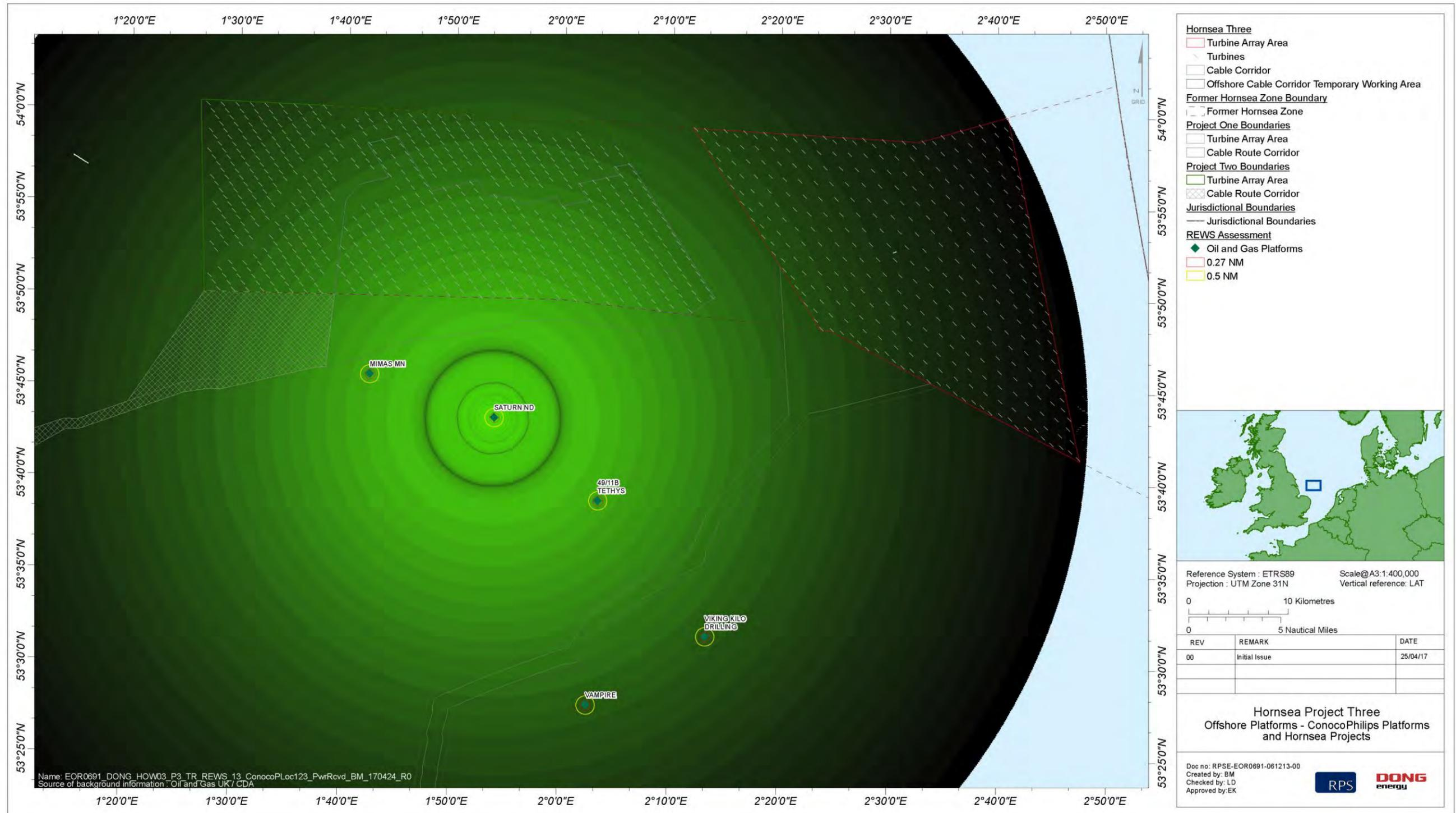
Figure 5.10: Modelled power received from 100 m² target (coverage).
