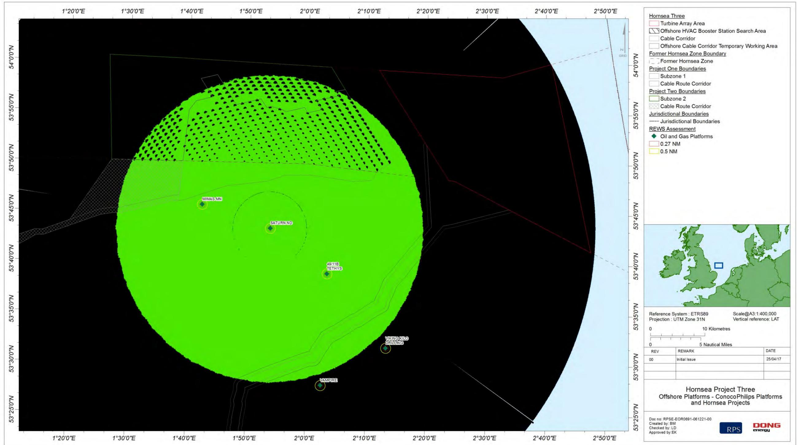
Figure 6.2: Saturn platform REWS detection plot using standard modified CFAR thresholding.
