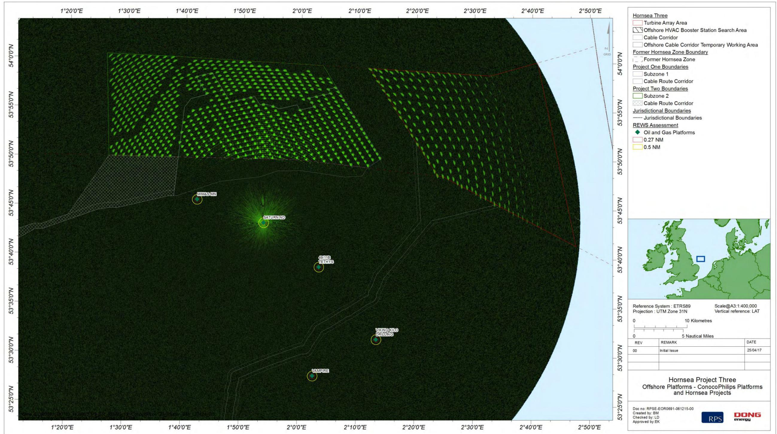
Figure 5.8: Saturn platform REWS clutter map showing returns from the combined Hornsea Project One, Hornsea Project Two and Hornsea Three and sea clutter.
