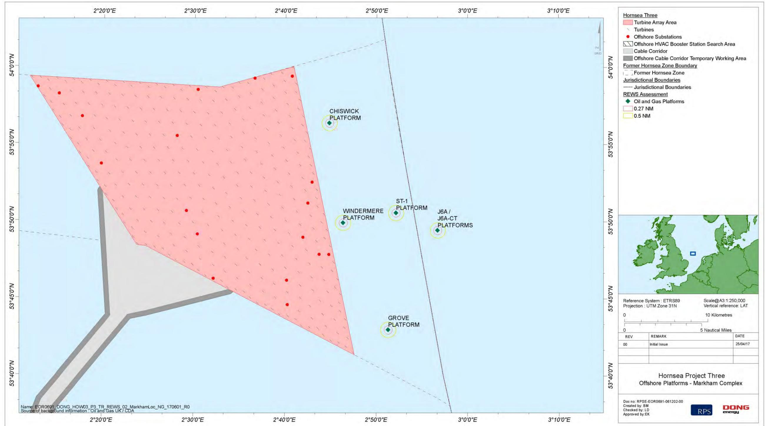
Figure 4.1: Modelled layout of the wind farm with respect to Centrica operated Markham complex of platforms.
