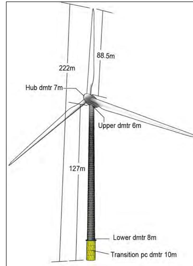
Figure 3.1: Modelled turbine geometry
