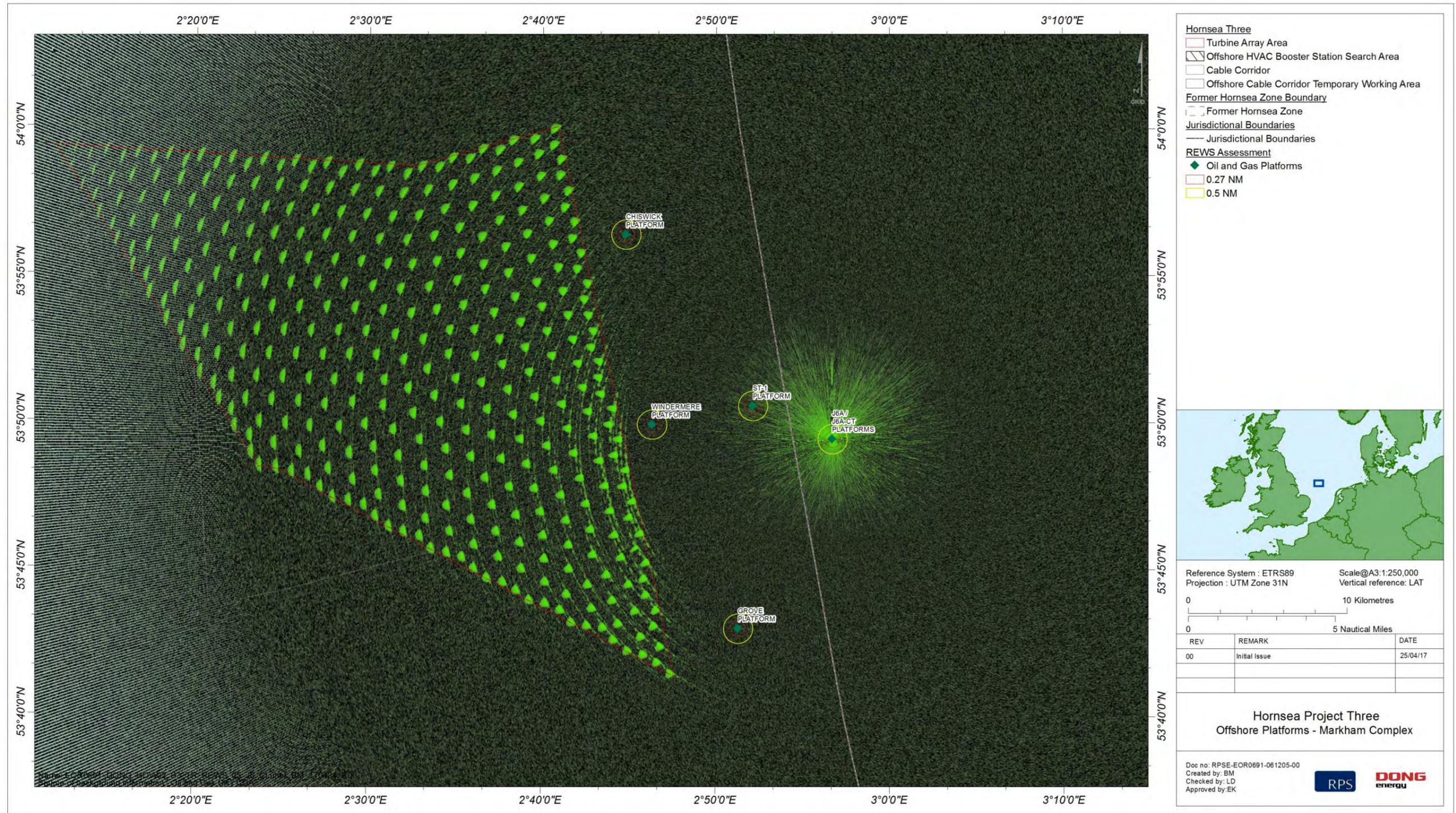
Figure 4.2: J6A platform REWS clutter map showing returns from the turbines and sea clutter.
