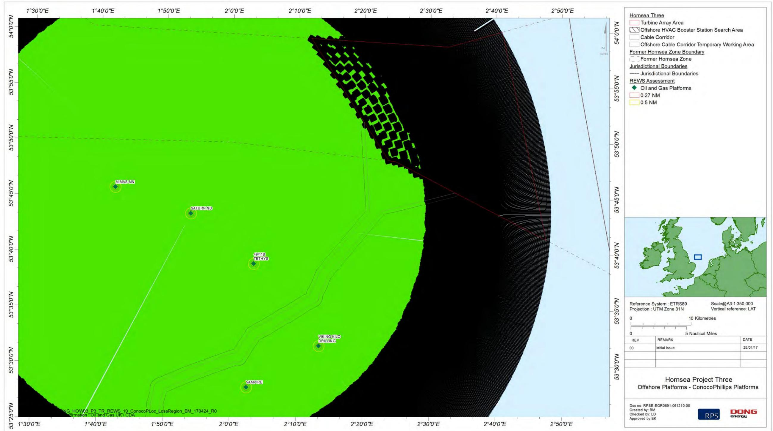
Figure 5.5: Saturn platform REWS detection plot showing loss regions for a large 1000 m² RCS target over the Hornsea Three array area.
