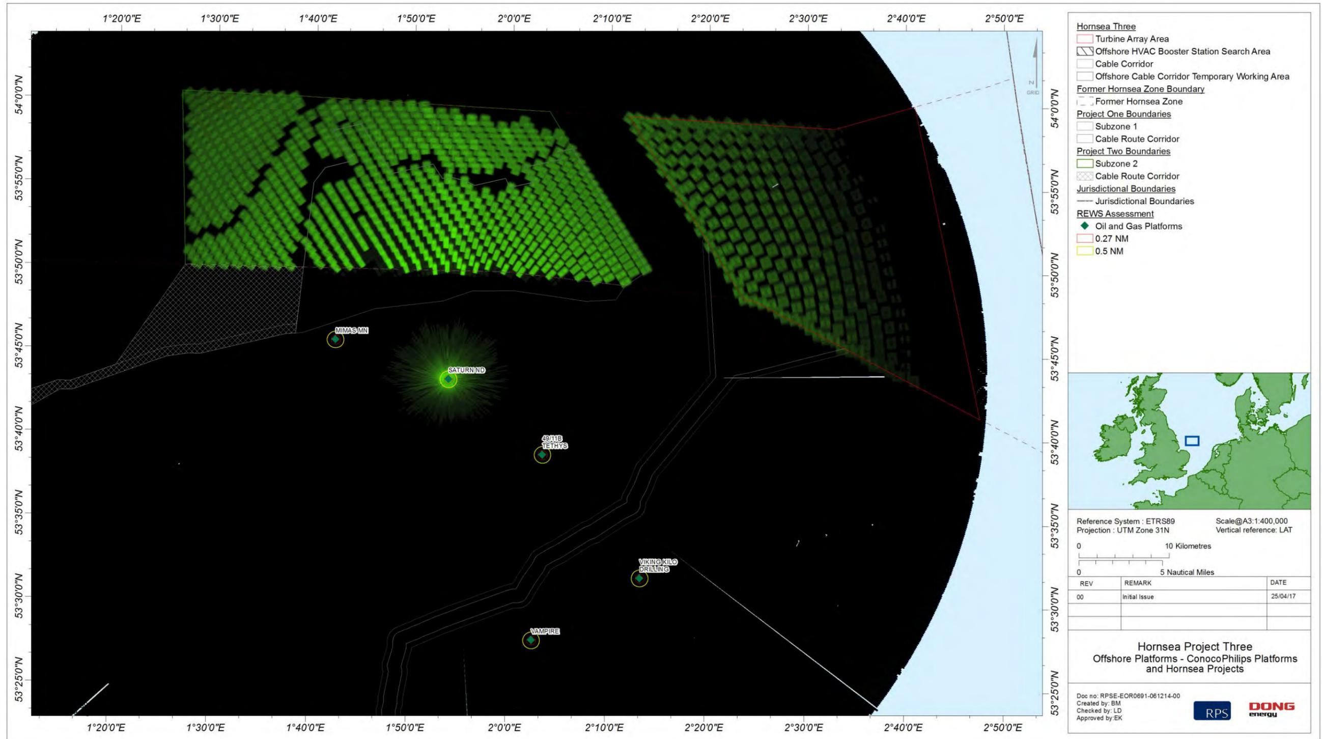
Figure 5.9: Saturn platform REWS detection threshold over the combined Hornsea Project One, Hornsea Project Two and Hornsea Three.
