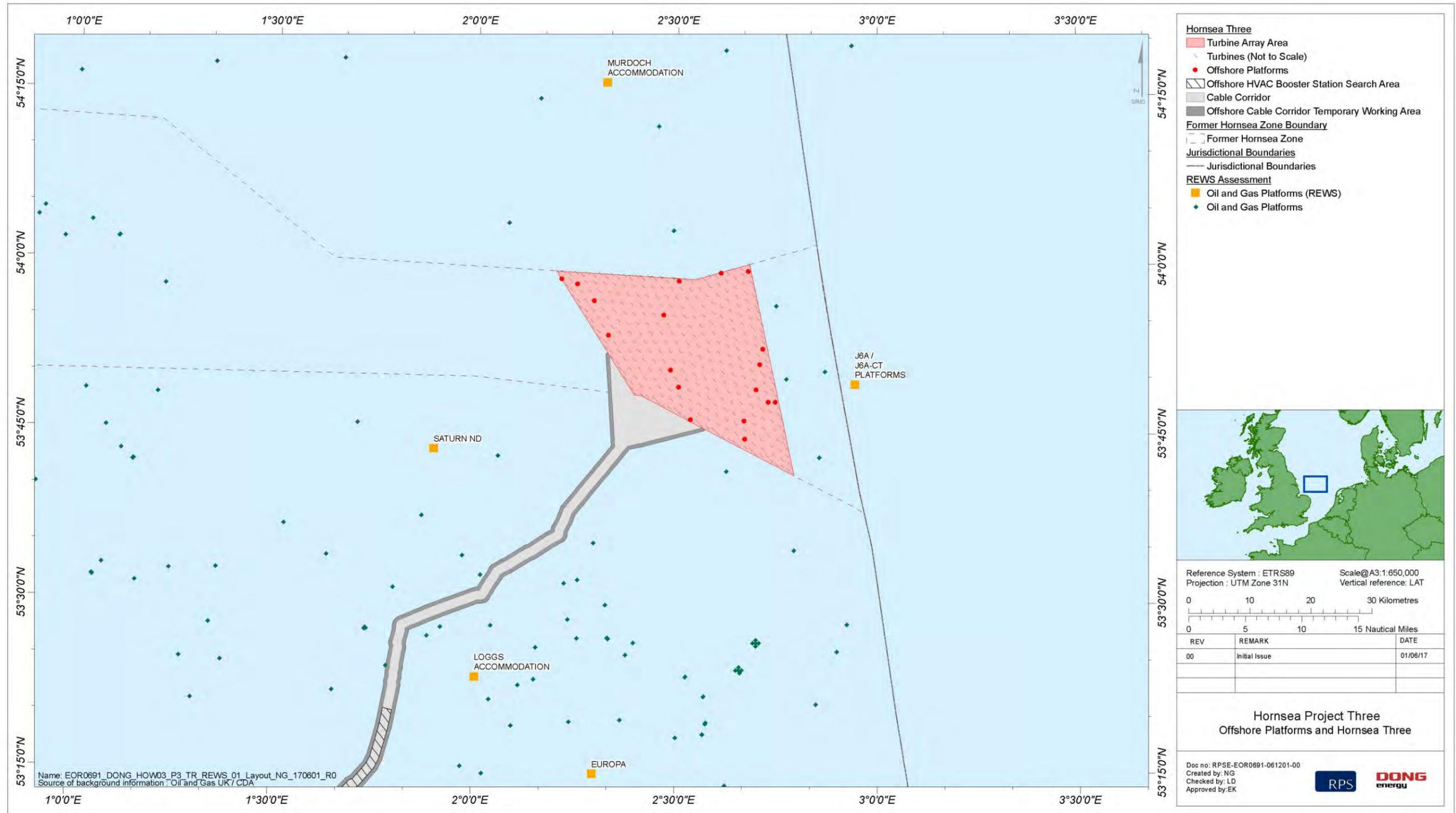
Figure 3.4: Indicative Hornsea Three layout with nearby offshore platforms with REWS.
