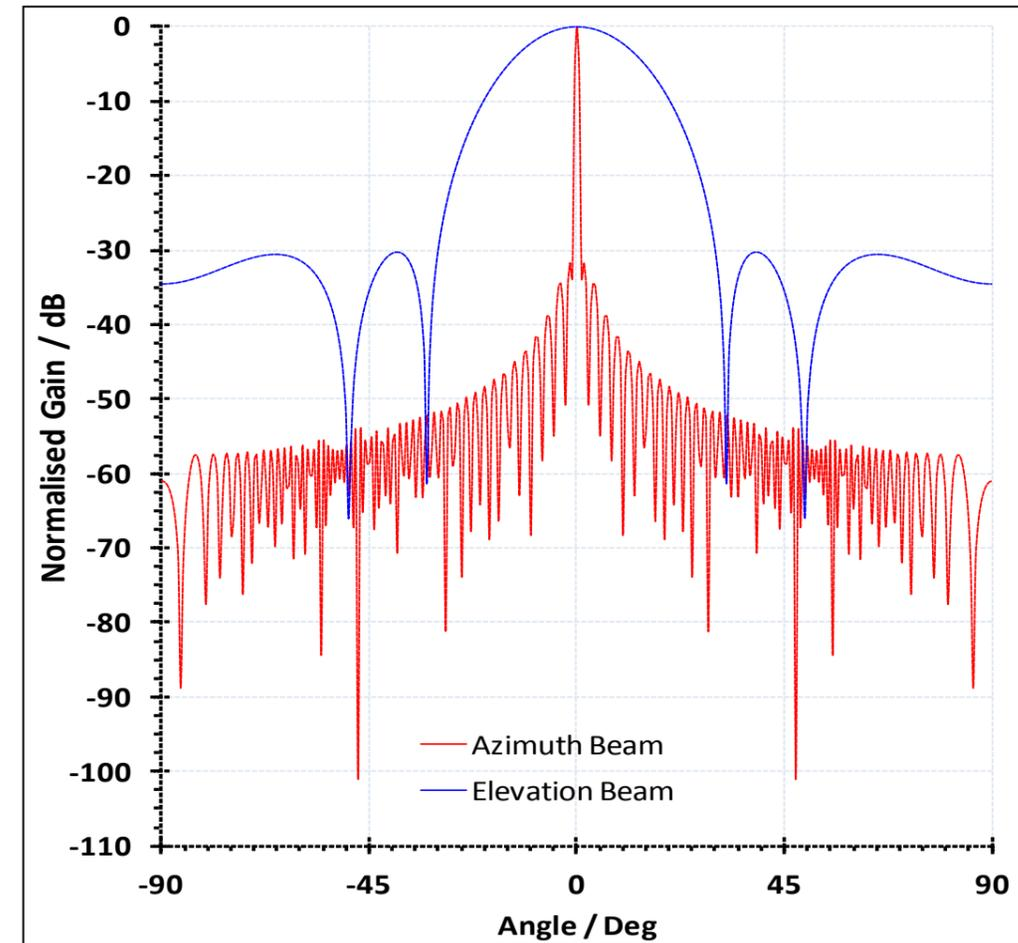
Figure 3.2: The radar antenna elevation and azimuth patterns.
