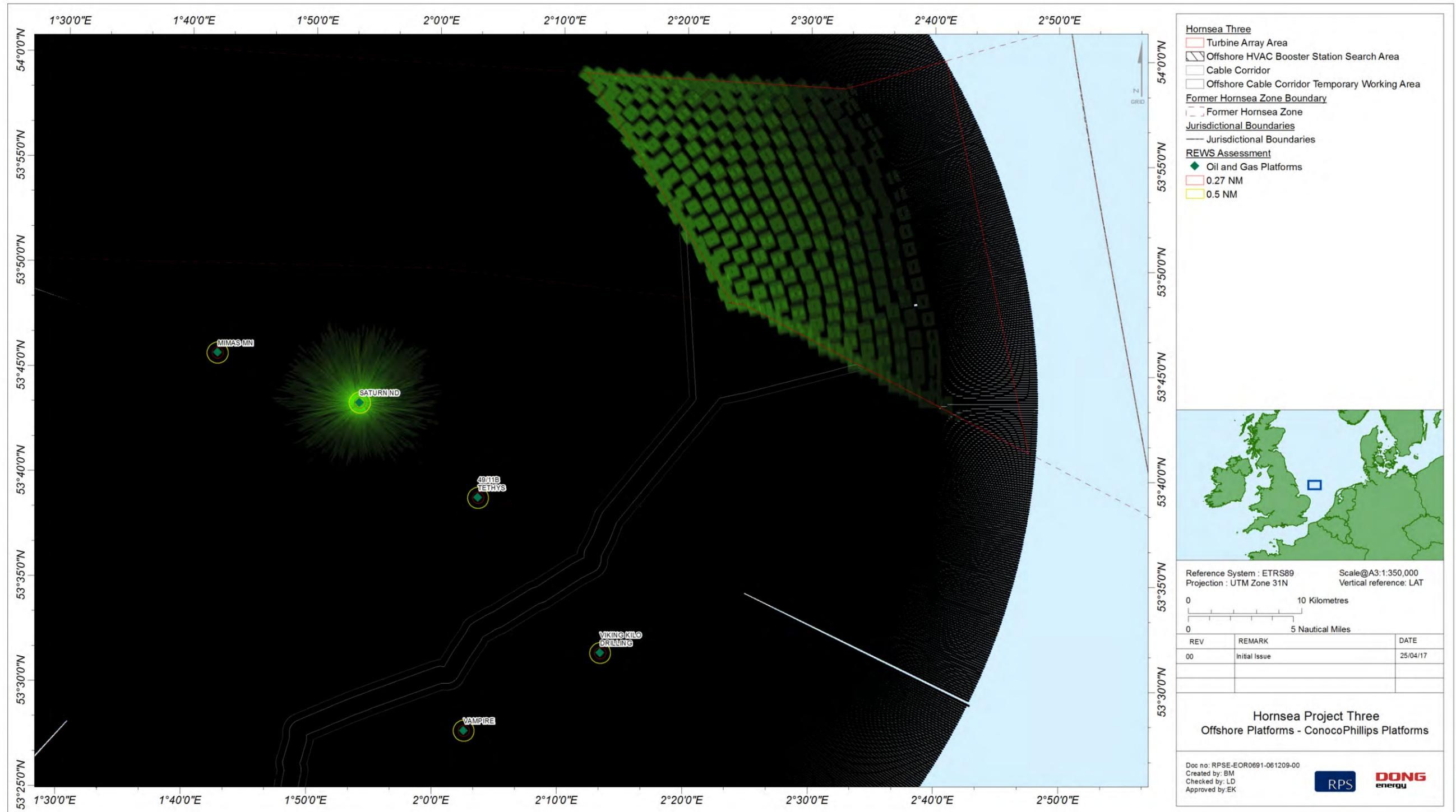
Figure 5.3: Saturn platform REWS detection threshold over the Hornsea Three array area.
