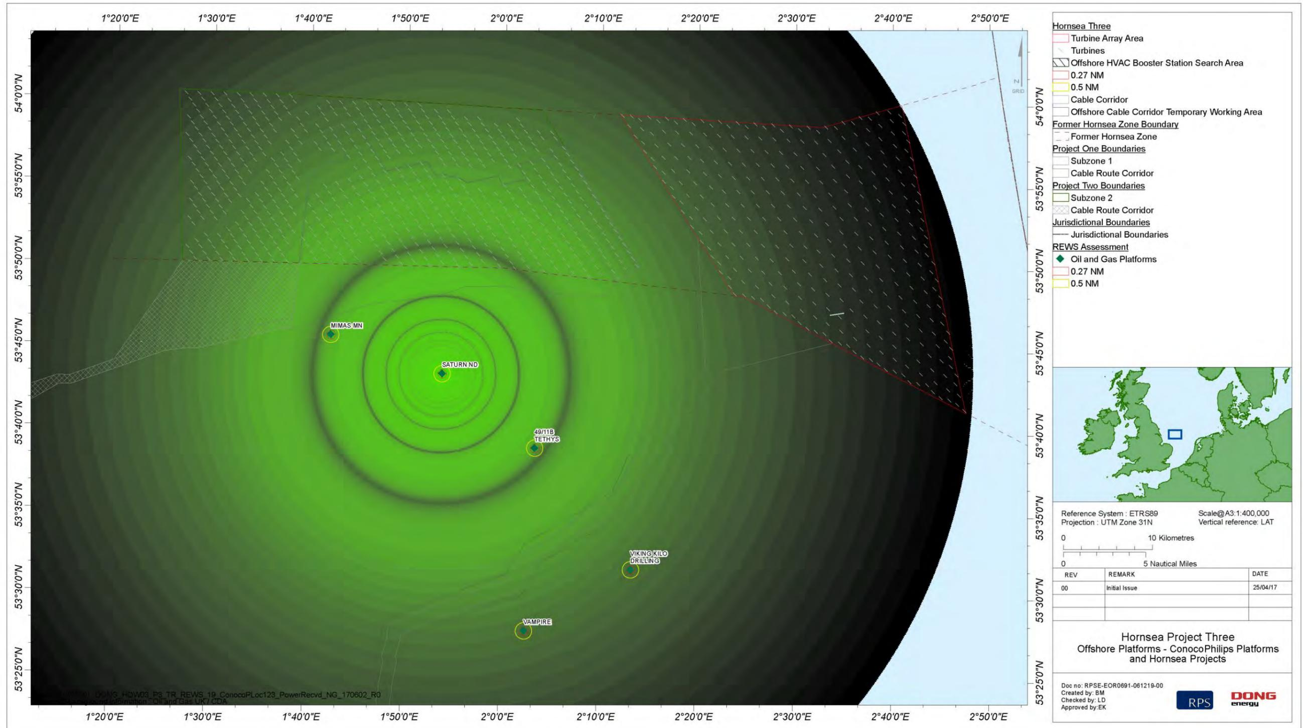
Figure 5.14: Modelled power received from the large 1,000 m² target (coverage).
