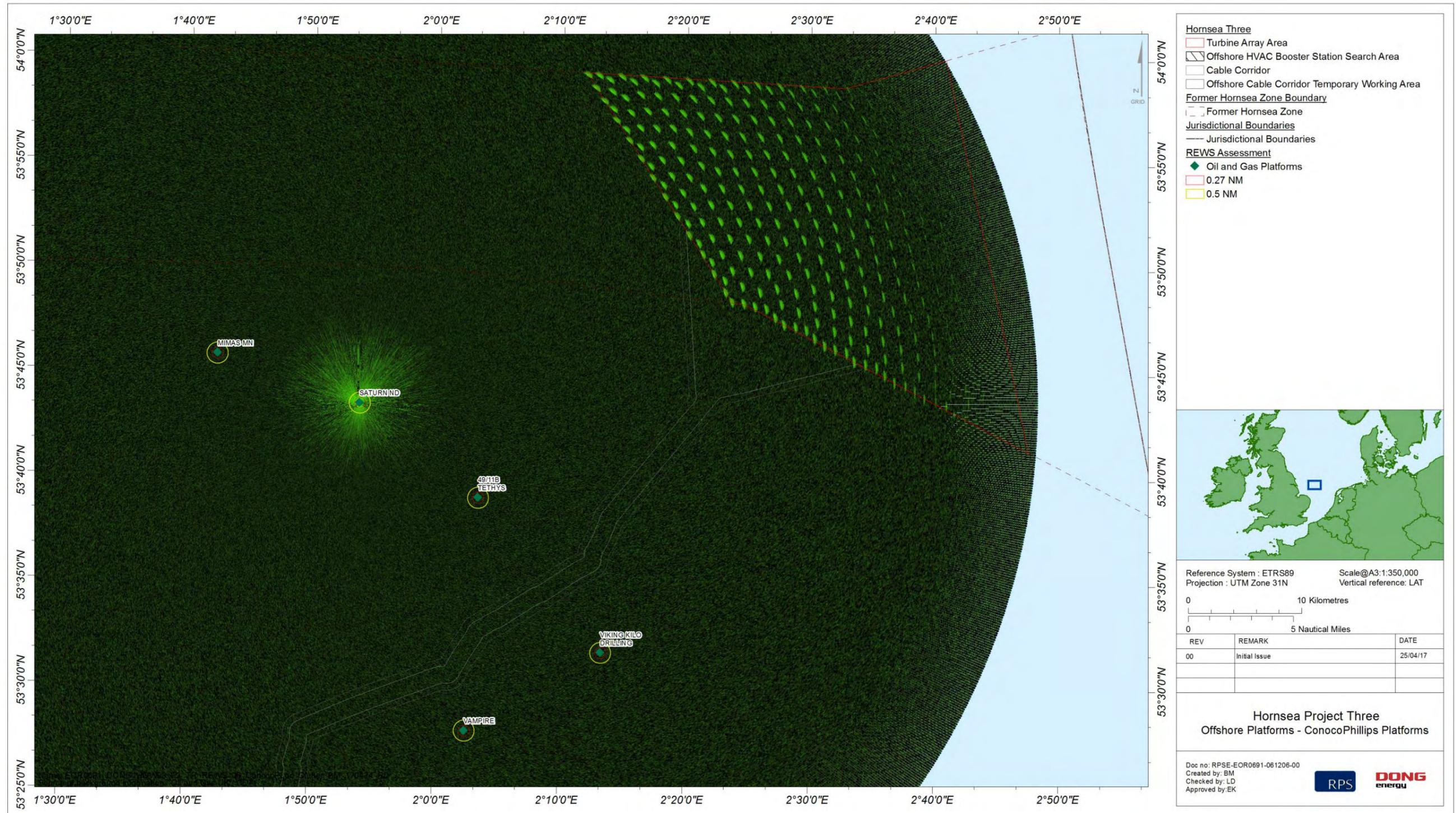
Figure 5.2: Saturn platform REWS clutter map showing returns from Hornsea Three and sea clutter.
