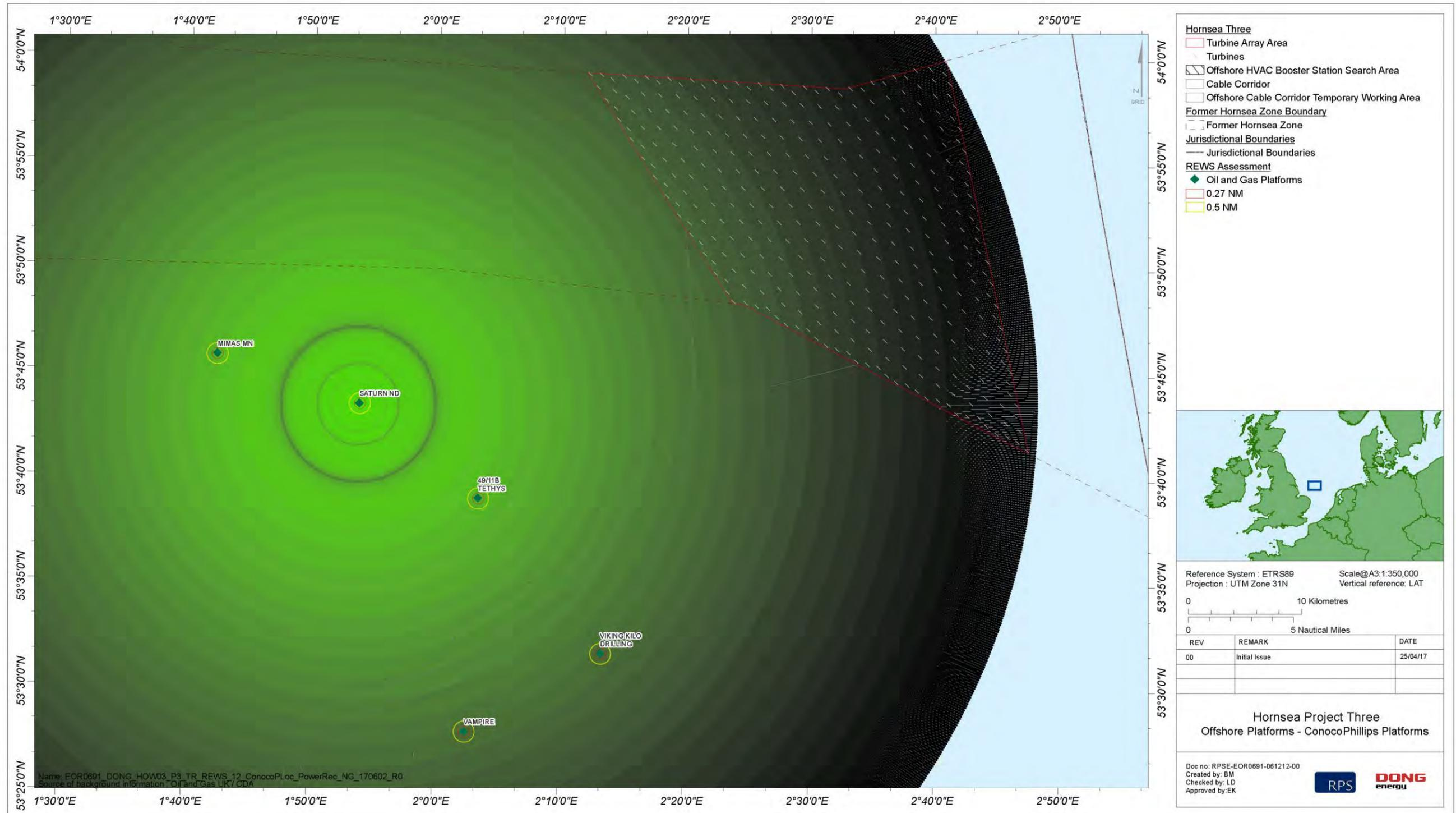
Figure 5.4: Modelled power received from 100 m² target (coverage).
