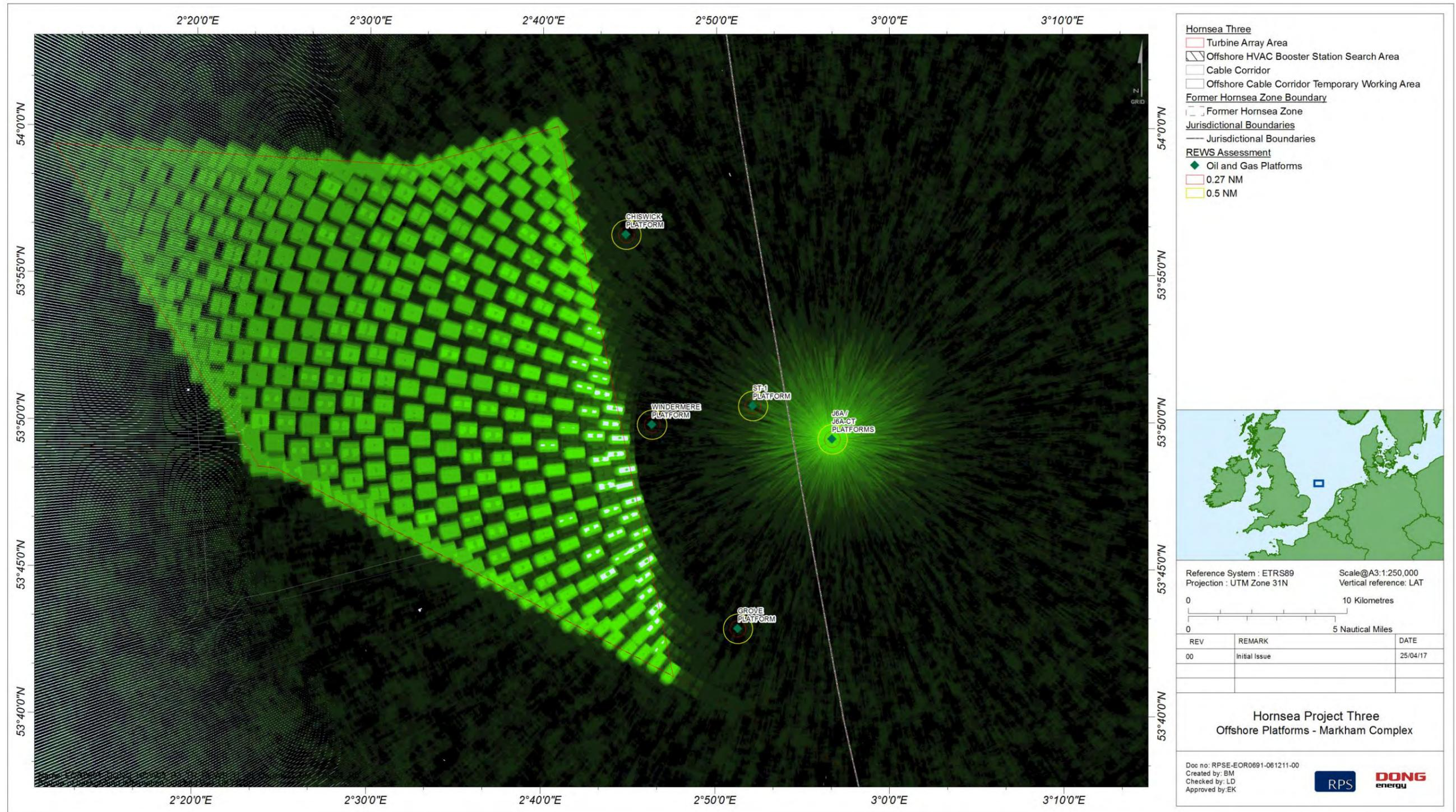
Figure 4.3: J6A platform REWS detection threshold over the Hornsea Three.
