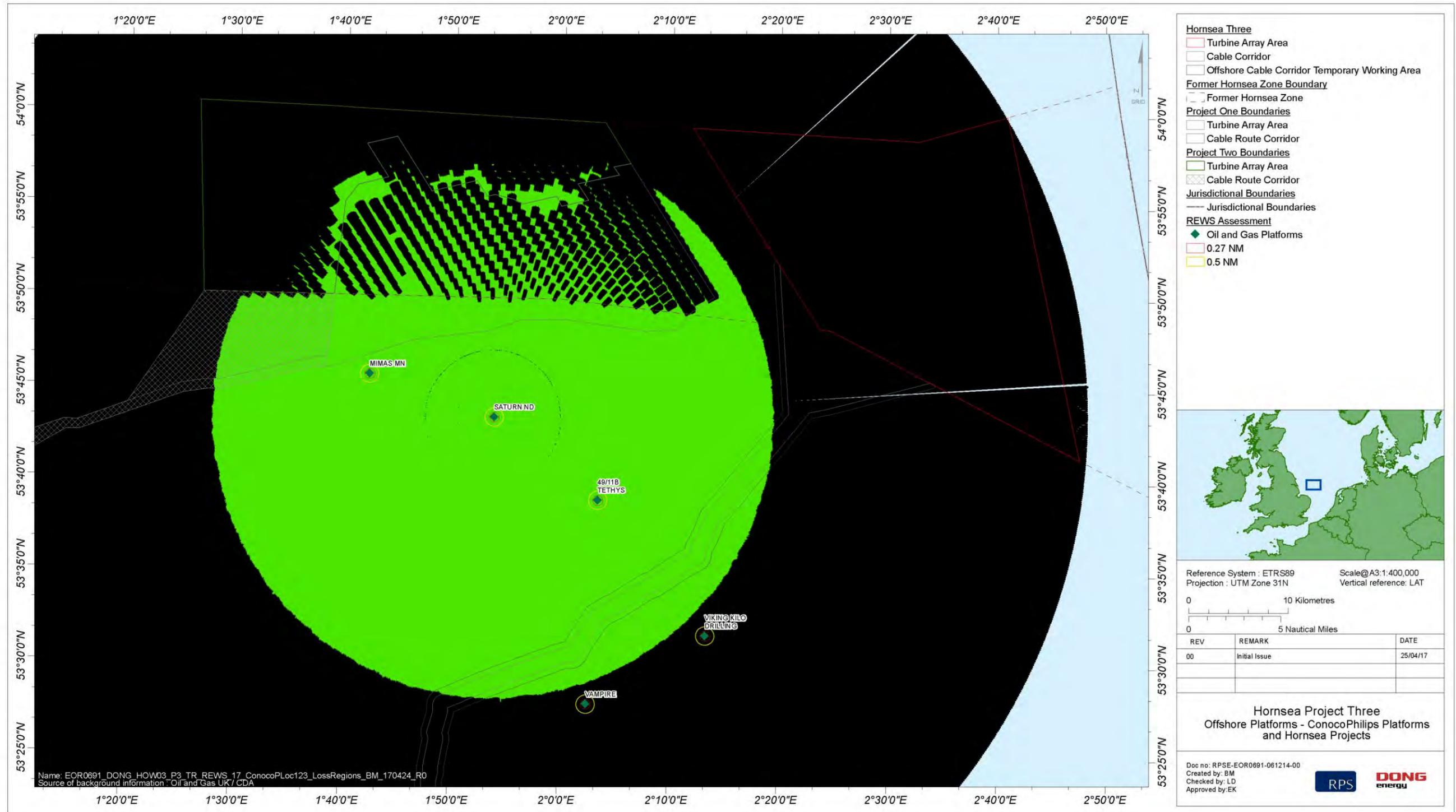
Figure 5.11: Saturn platform REWS detection plot showing loss regions for a 100 m<sup>2</sup> target over the combined Hornsea Project One, Hornsea Project Two and Hornsea Three.
