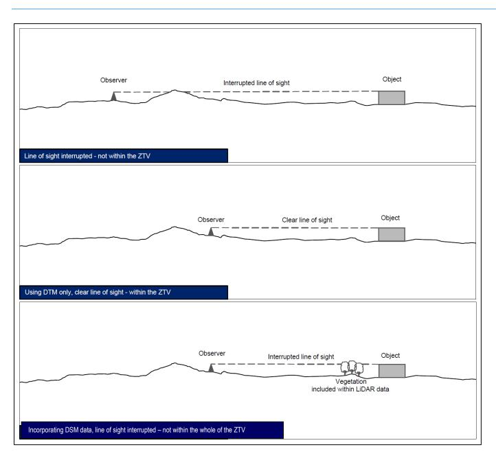
Figure D.1 Zone of Theoretical Visibility – Methodology and Assumptions.
