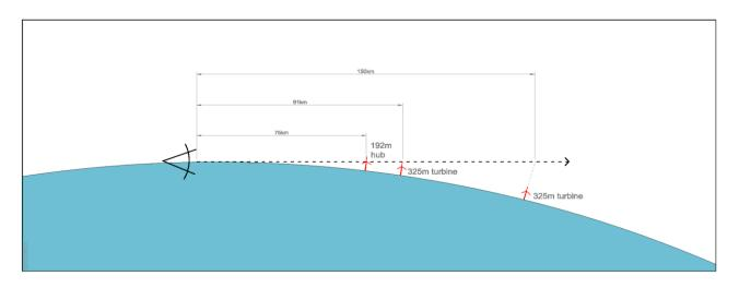
Figure 4.10: Illustration of the effects of curvature of the earth on visibility (not to scale).
