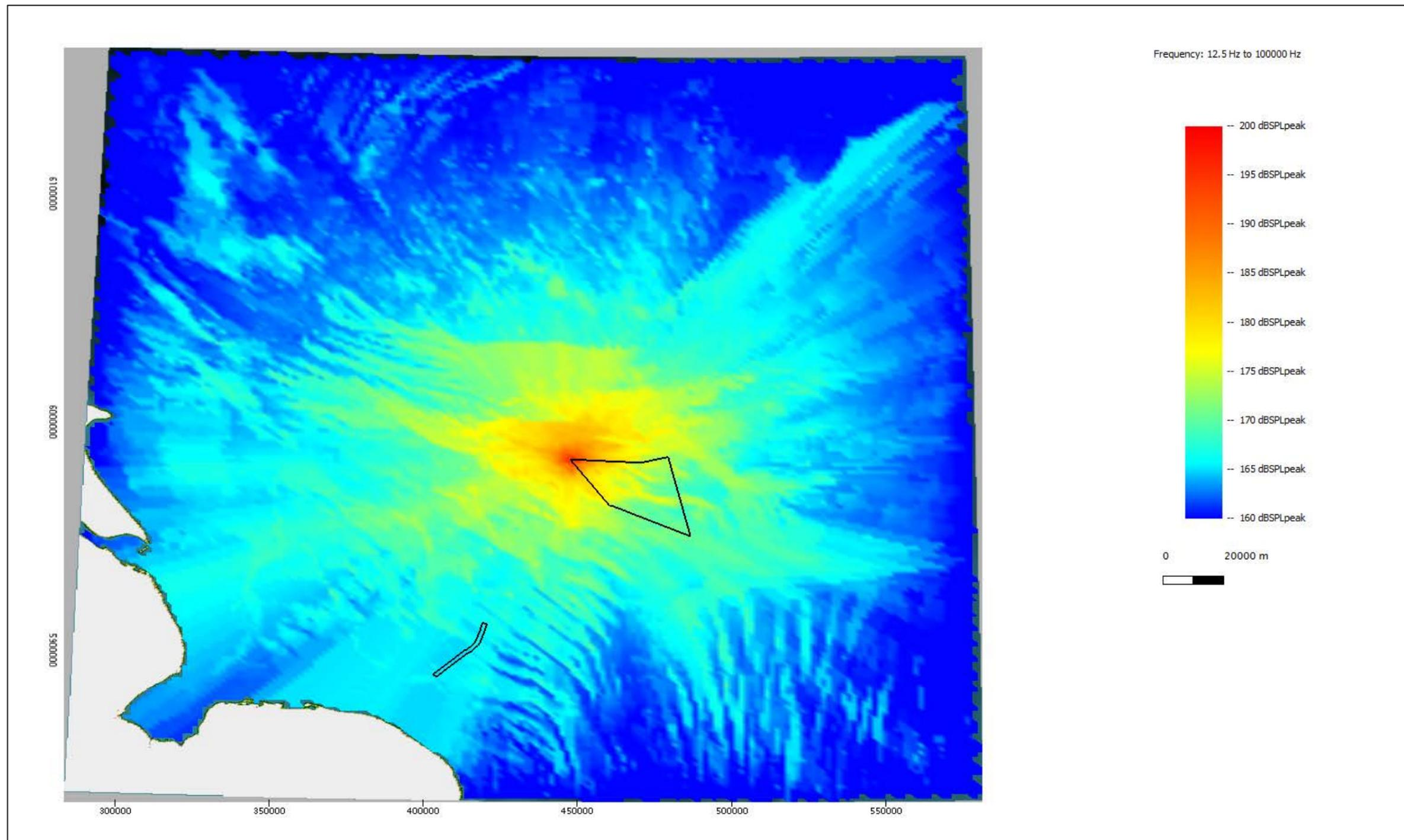
Figure A.6: Noise level plot showing the modelled unweighted  $SPL_{peak}$  noise levels at the Northwest location of Hornsea Three for installing a pin pile with a maximum blow energy of 2500 kJ.
