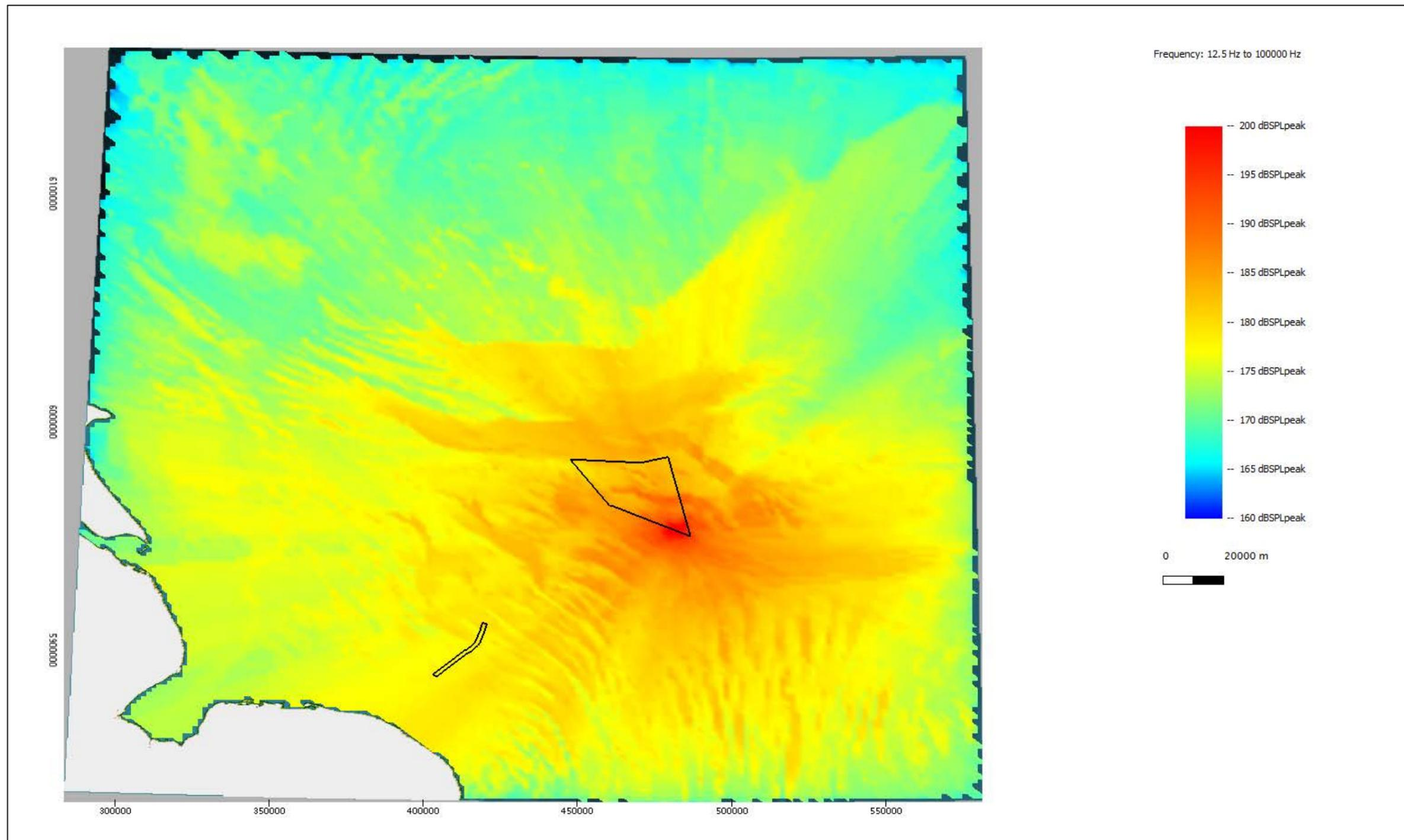
Figure A.3: Noise level plot showing the modelled unweighted  $SPL_{peak}$  noise levels at the South location of Hornsea Three for installing a monopile with a maximum blow energy of 5000 kJ.
