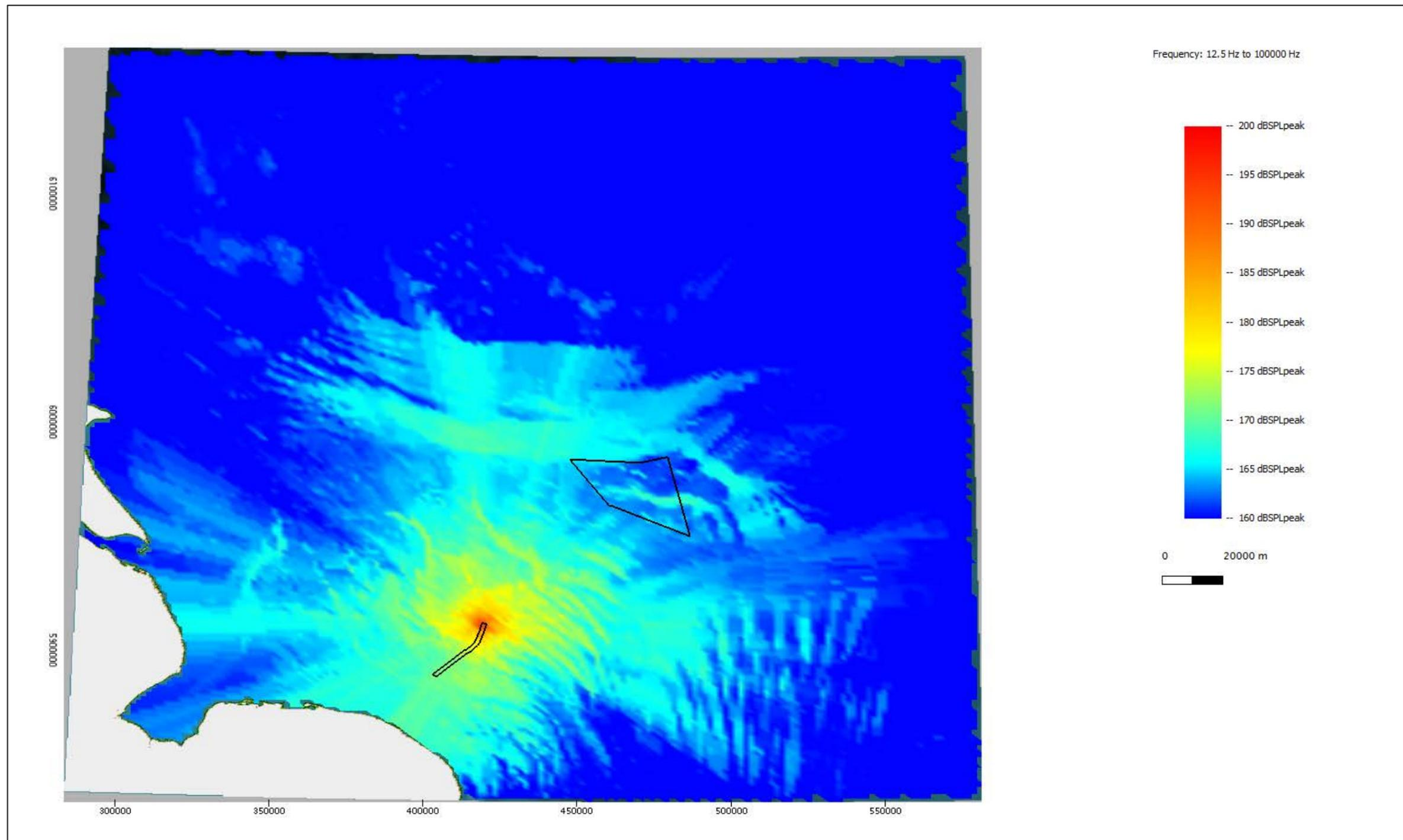
Figure A.9: Noise level plot showing the modelled unweighted SPL<sub>peak</sub> noise levels at the HVAC North location for installing a pin pile with a maximum blow energy of 2500 kJ.
