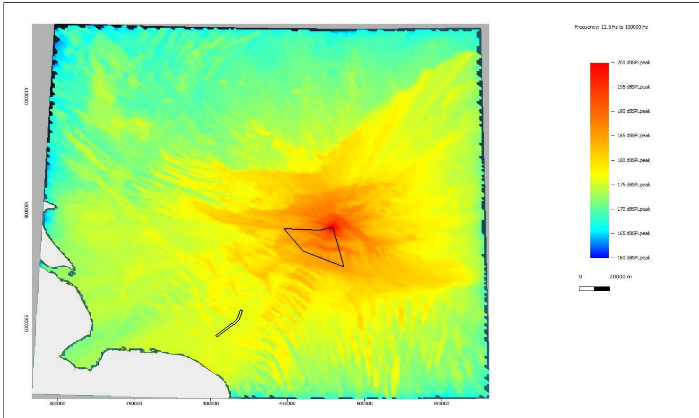
Figure A.2: Noise level plot showing the modelled unweighted SPL<sub>peak</sub> noise levels at the Northeast location of Hornsea Three for installing a monopile with a maximum blow energy of 5000 kJ.
