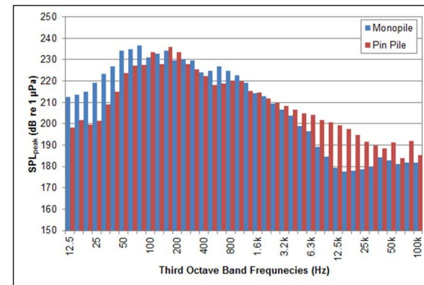
Figure 5.2: Third octave source level frequency spectra for the Northwest location, maximum blow energy.
