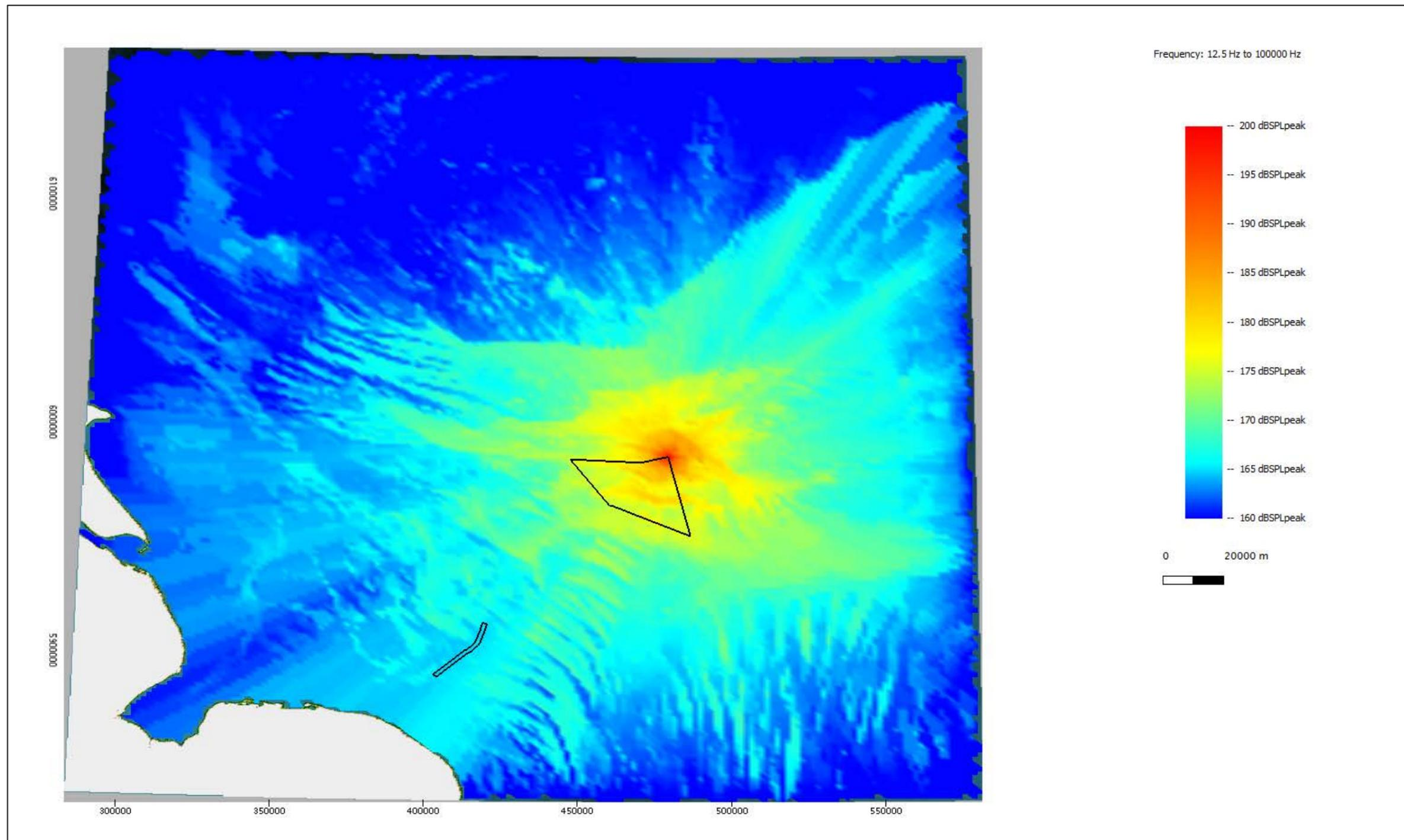
Figure A.7: Noise level plot showing the modelled unweighted  $SPL_{peak}$  noise levels at the Northeast location of Hornsea Three for installing a pin pile with a maximum blow energy of 2500 kJ.
