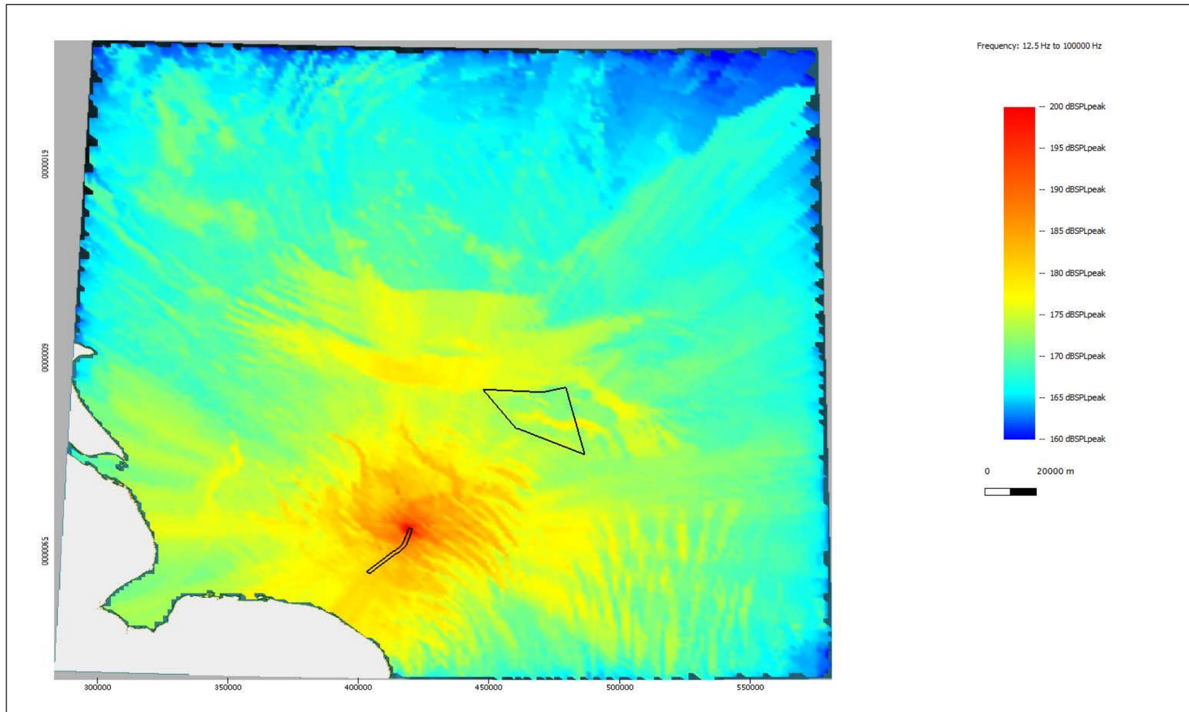
Figure A.4: Noise level plot showing the modelled unweighted  $SPL_{peak}$  noise levels at the HVAC North location for installing a monopile with a maximum blow energy of 5000 kJ.
