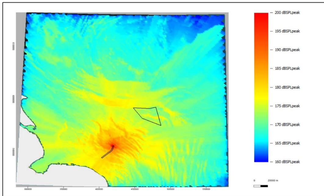
Figure 5.4: Noise level plot showing the modelled unweighted  $SPL_{peak}$  noise levels at the HVAC North location for installing a monopile with a maximum blow energy of 5000 kJ.
