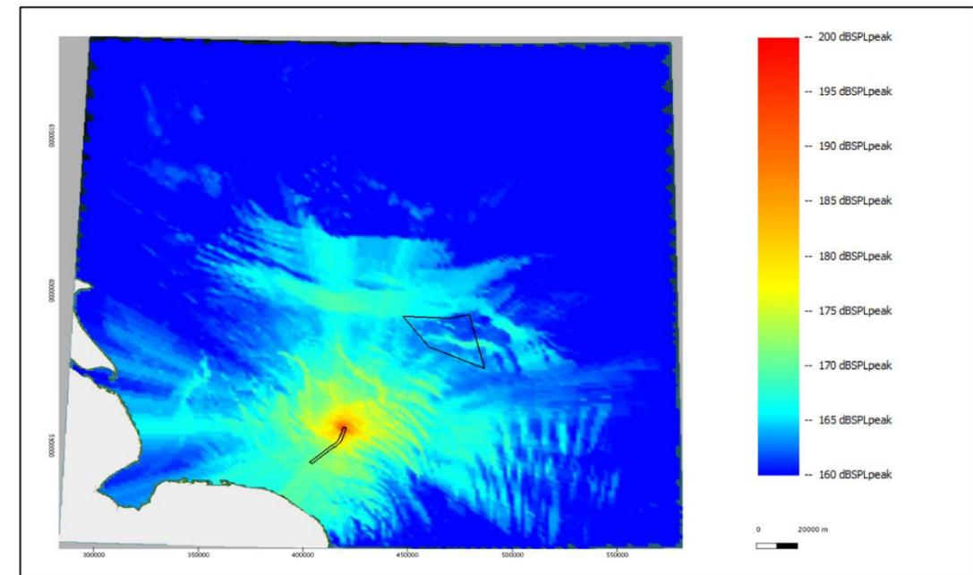
Figure 5.6: Noise level plot showing the modelled unweighted  $SPL_{peak}$  noise levels at the HVAC North location for installing a pin pile with a maximum blow energy of 2500 kJ.
