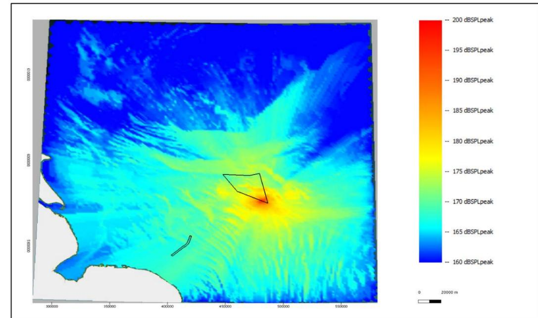
Figure 5.5: Noise level plot showing the modelled unweighted  $SPL_{peak}$  noise levels at the South location of Hornsea Three for installing a pin pile with a maximum blow energy of 2500 kJ.
