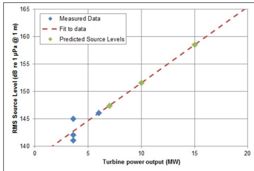
Figure 6.1: Extrapolated source levels from operational turbines plotted with a linear fit to estimate source levels for larger turbines.
