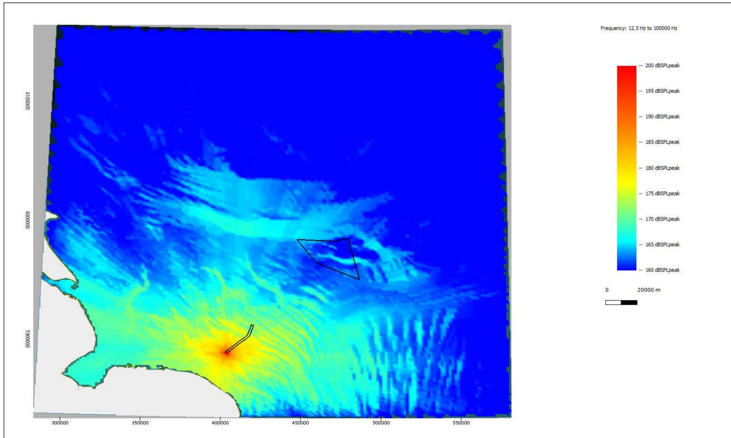
Figure A.10: Noise level plot showing the modelled unweighted  $SPL_{peak}$  noise levels at the HVAC South location for installing a pin pile with a maximum blow energy of 2500 kJ.
