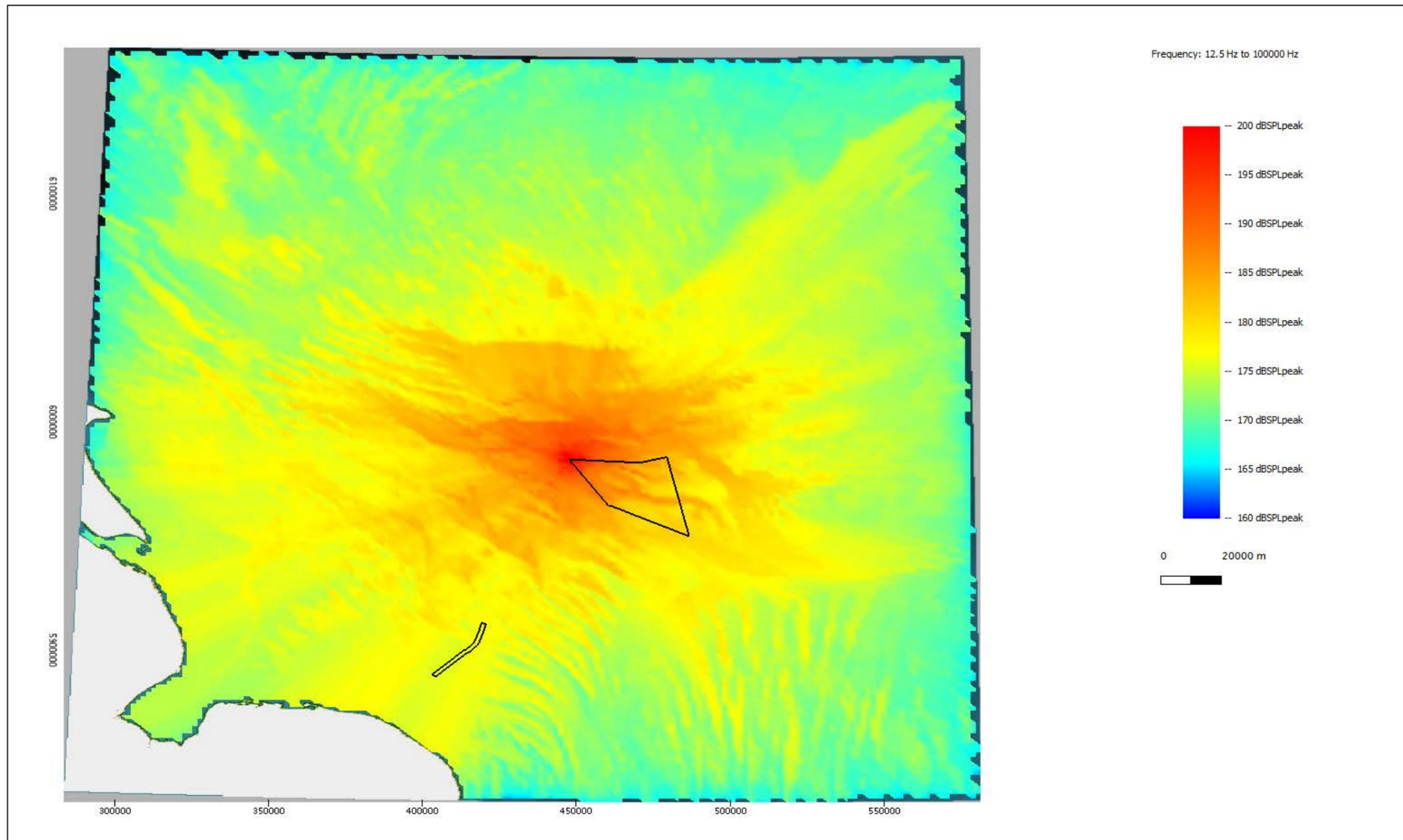
Figure A.1: Noise level plot showing the modelled unweighted SPL<sub>peak</sub> noise levels at the Northwest location of Hornsea Three for installing a monopile with a maximum blow energy of 5000 kJ.
