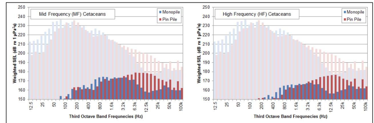
Figure 5.9: Filtered noise inputs for monopiles and pin piles using the MF cetacean and HF cetacean filters from NMFS (2016). The translucent bars show the unweighted third octave levels.
