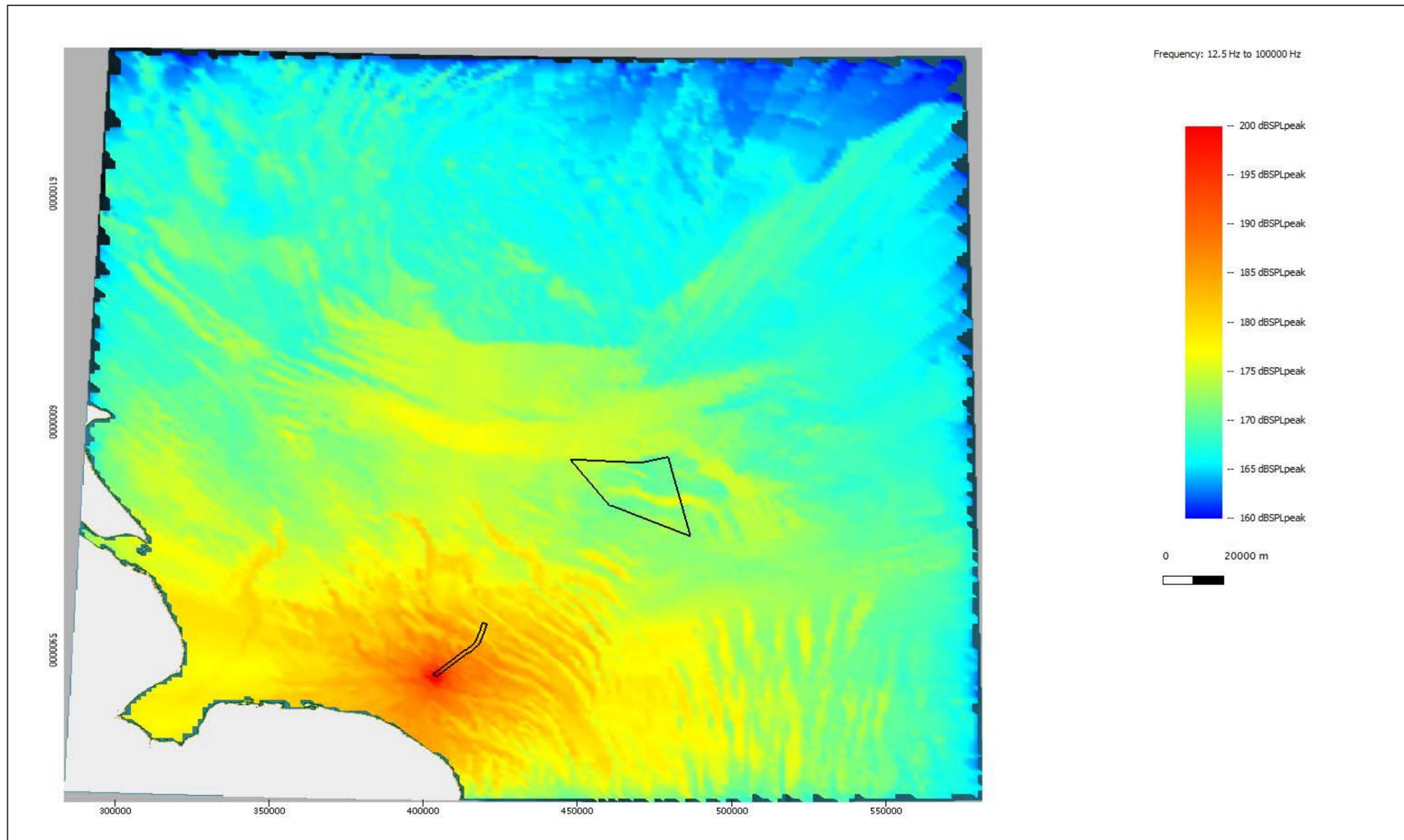
Figure A.5: Noise level plot showing the modelled unweighted SPL<sub>peak</sub> noise levels at the HVAC South location for installing a monopile with a maximum blow energy of 5000 kJ.
