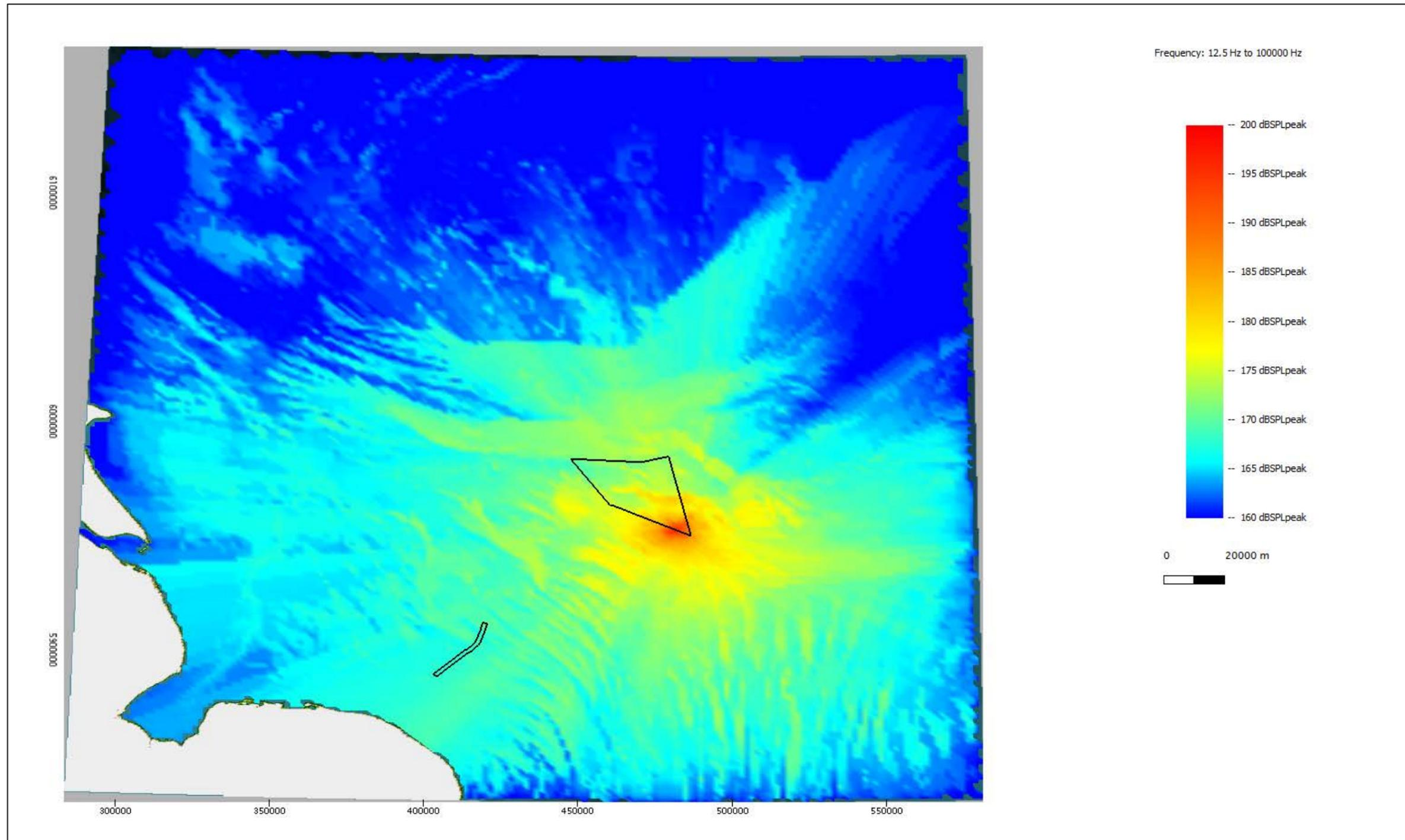
Figure A.8: Noise level plot showing the modelled unweighted SPL<sub>peak</sub> noise levels at the South location of Hornsea Three for installing a pin pile with a maximum blow energy of 2500 kJ.
