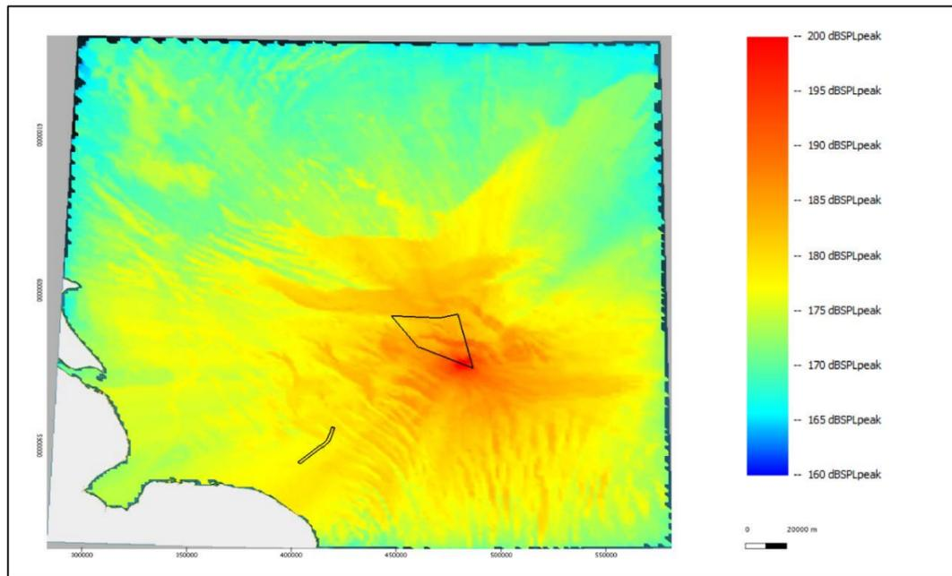
Figure 5.3: Noise level plot showing the modelled unweighted  $SPL_{peak}$  noise levels at the South location of Hornsea Three for installing a monopile with a maximum blow energy of 5000 kJ.
