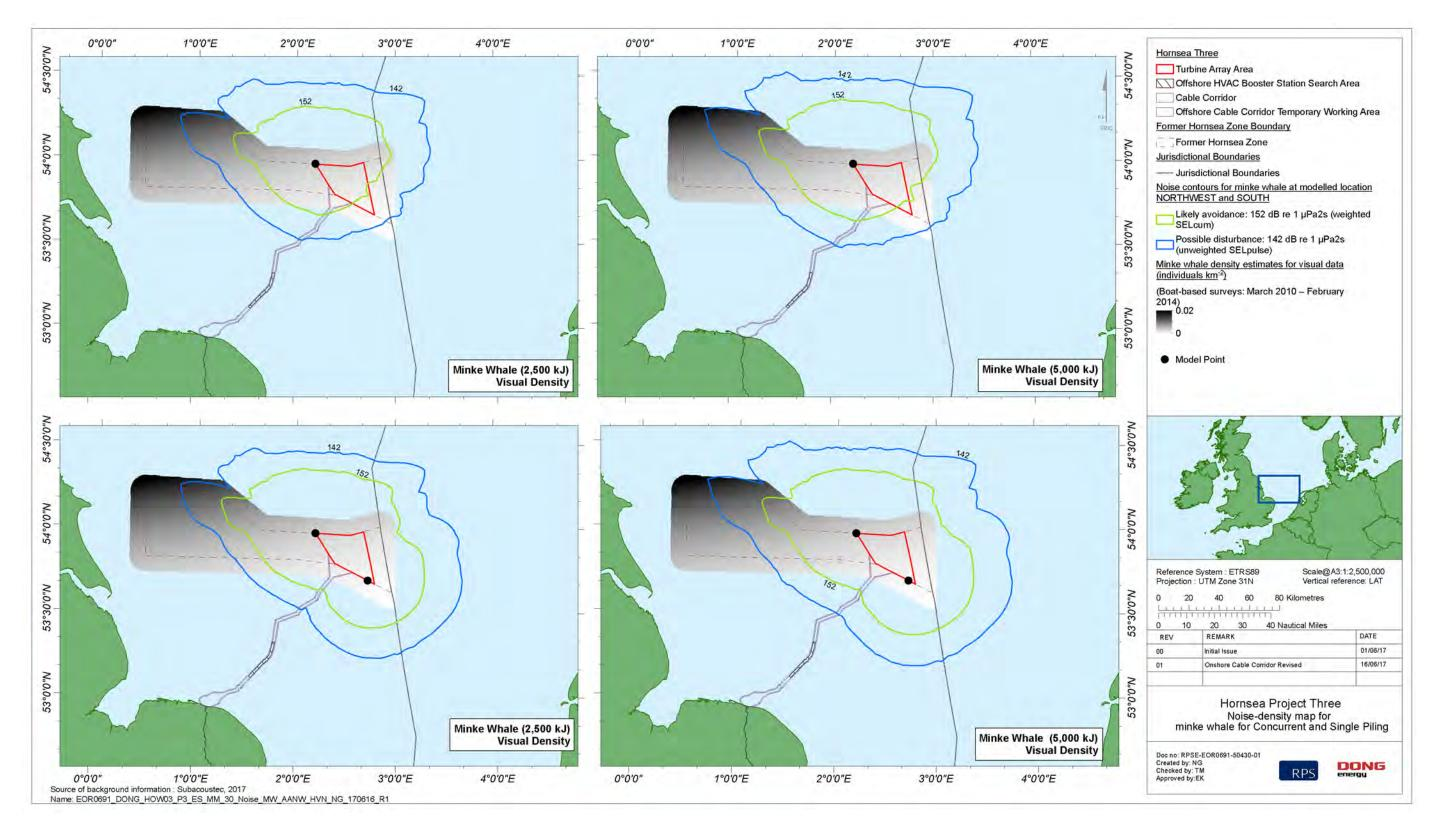
Figure 4.16: Noise density map for minke whale for concurrent and single piling in the Hornsea Three array area.
