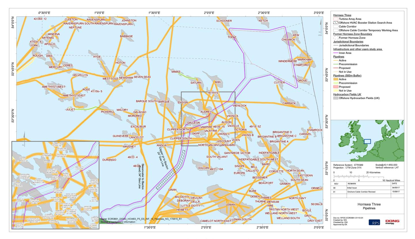
Figure 11.9: Pipelines located in the vicinity of Hornsea Three.
