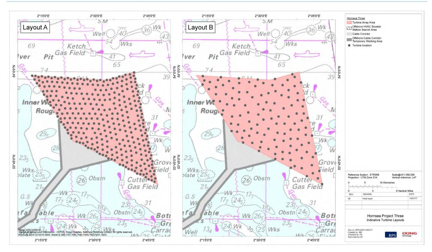
Figure 10.5: Indicative turbine layouts for the Hornsea Three array area.
