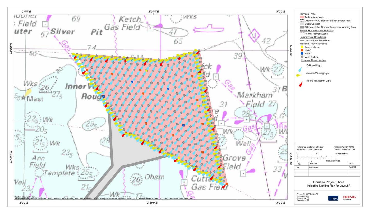
Figure 10.6: Indicative lighting plan for Layout A.
