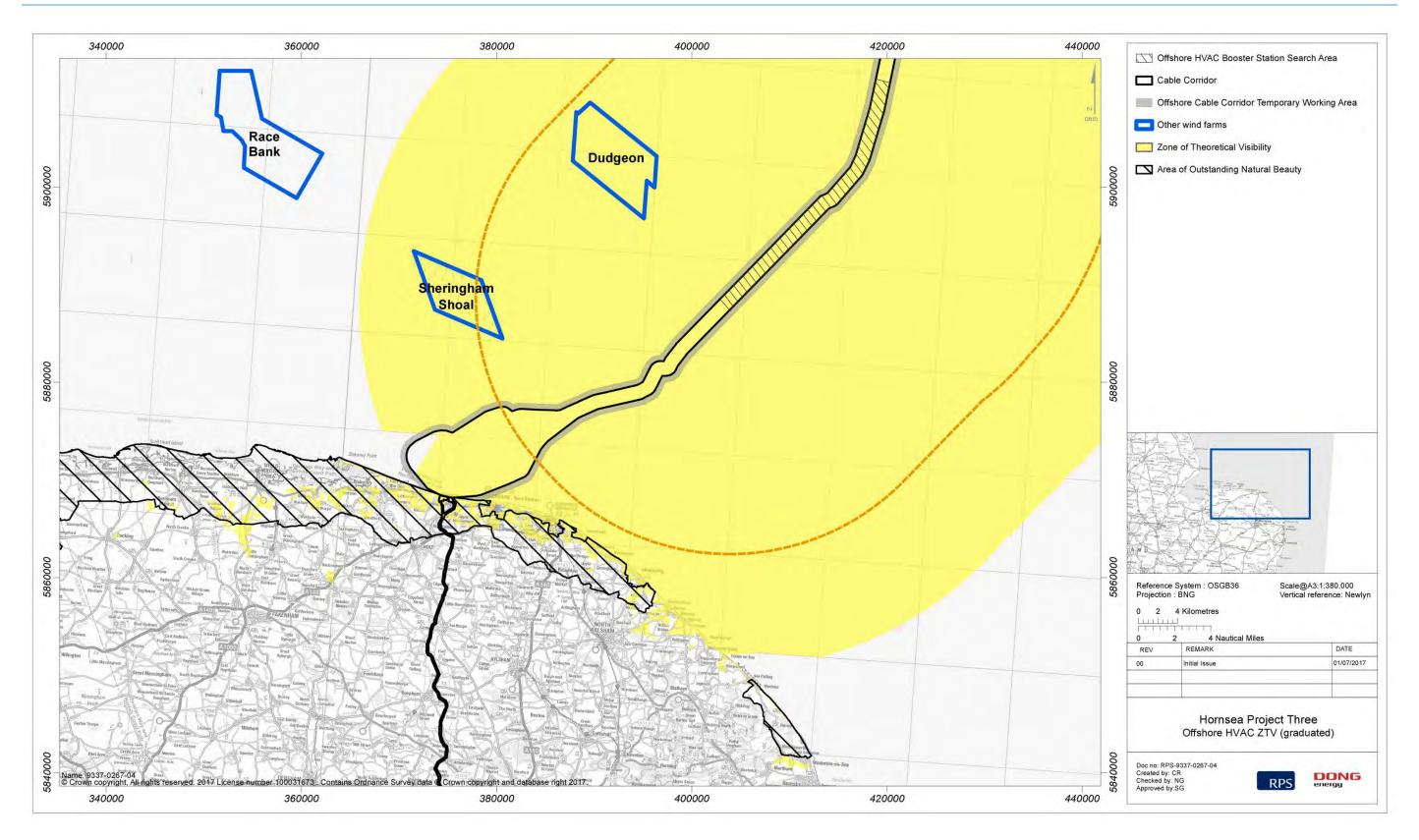
Figure 10.3: ZTV for the offshore HVAC booster stations.
