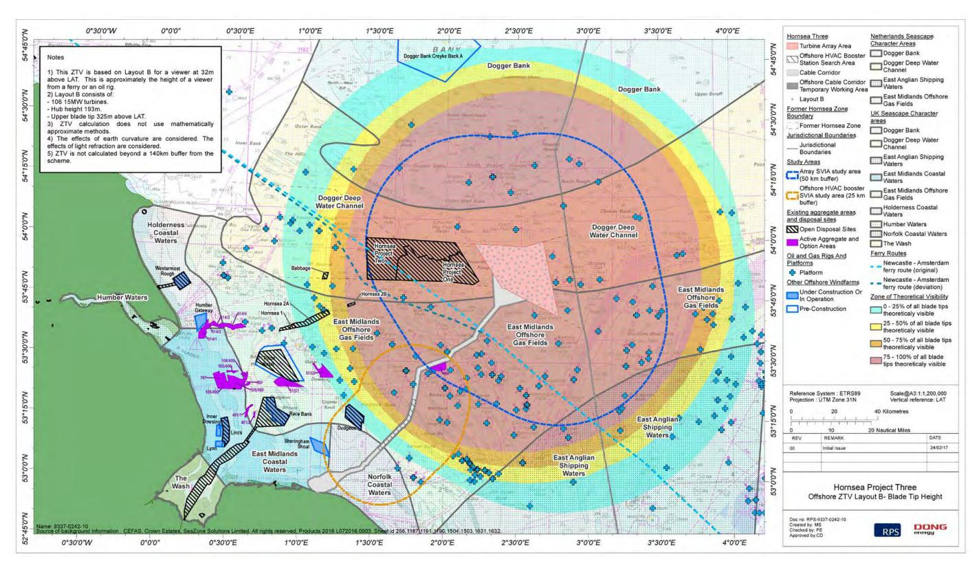
Figure 10.10: Offshore ZTV Layout B – blade tip height.
