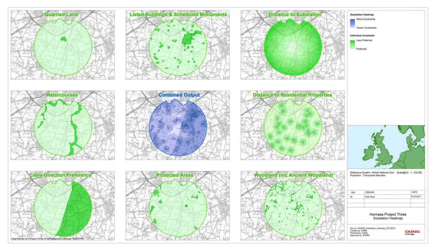
Figure 4.14: Constraints mapping of substation search area.
