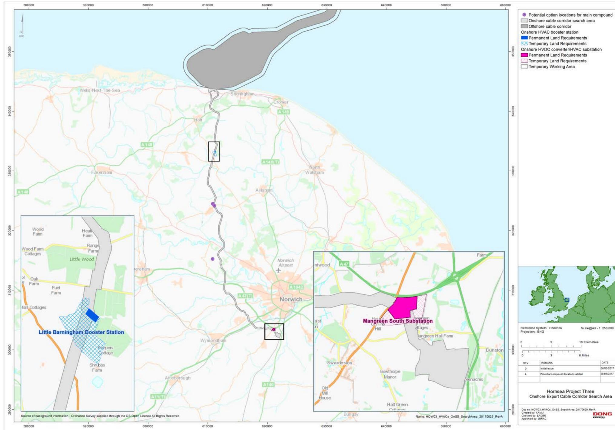
Figure 3.22: Onshore export cable route and locations for HVAC booster station and onshore HVDC converter/HVAC substation.
