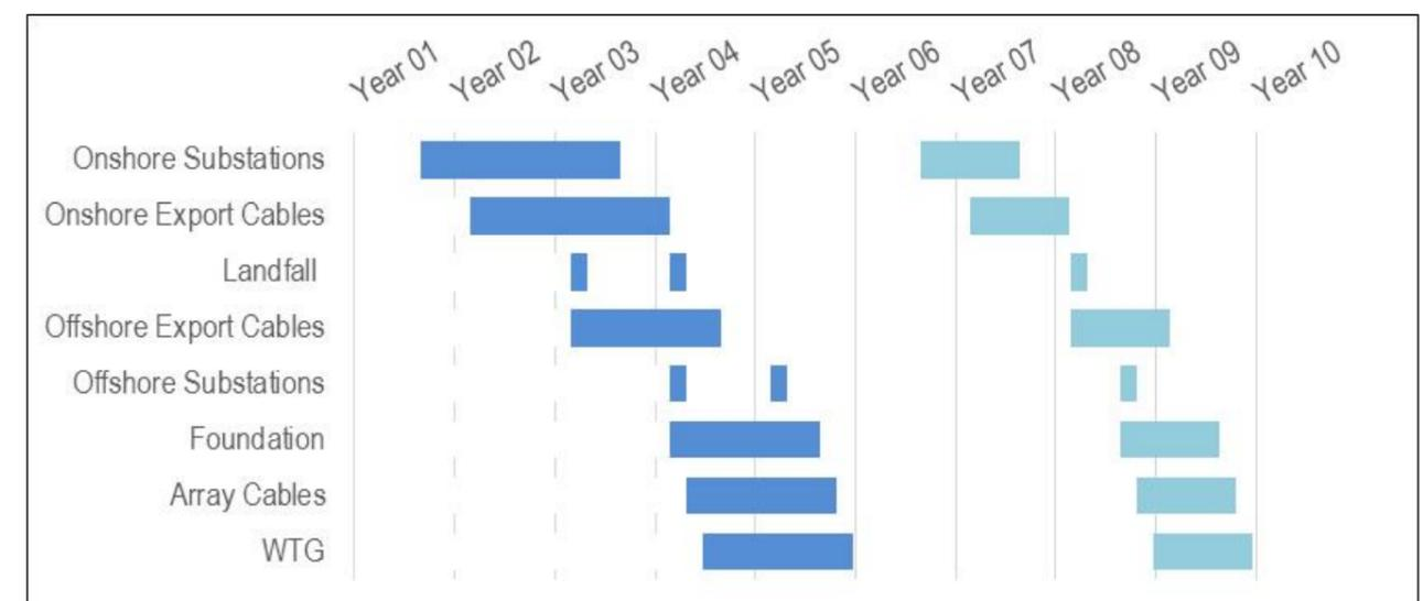
Figure 3.29: Indicative construction programme if project built out in two fully sequential phases.
