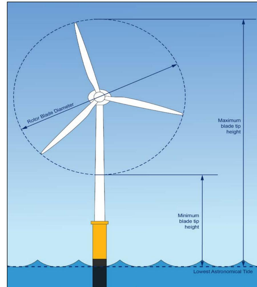
Figure 3.3: Schematic of an offshore wind turbine.
