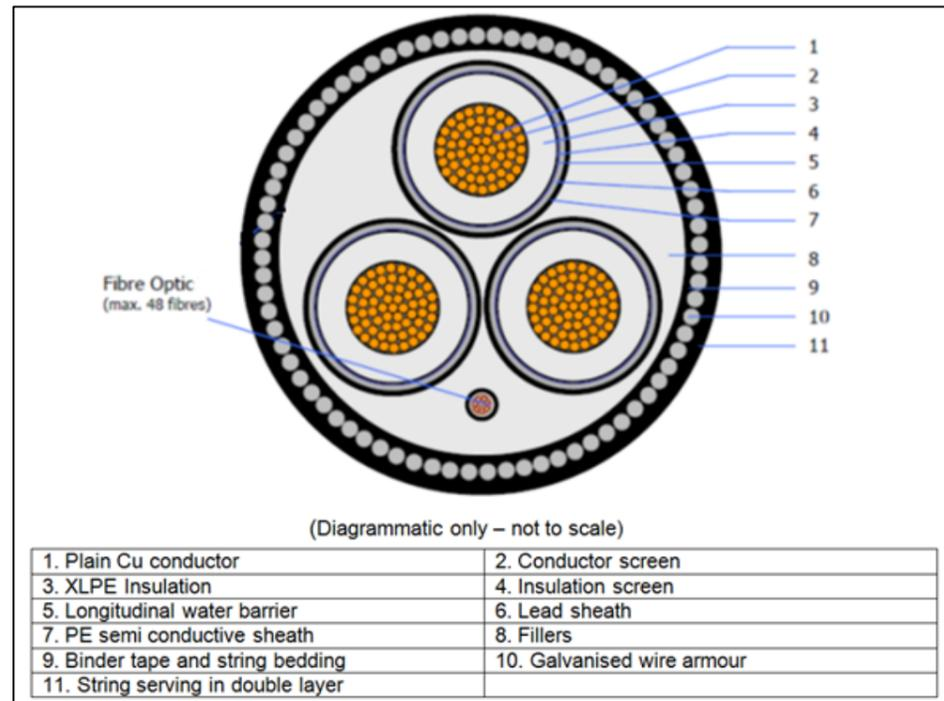
Figure 3.17: Cross section through a typical offshore alternating current (AC) (220 kV) export cable (Courtesy of Prysmian).
