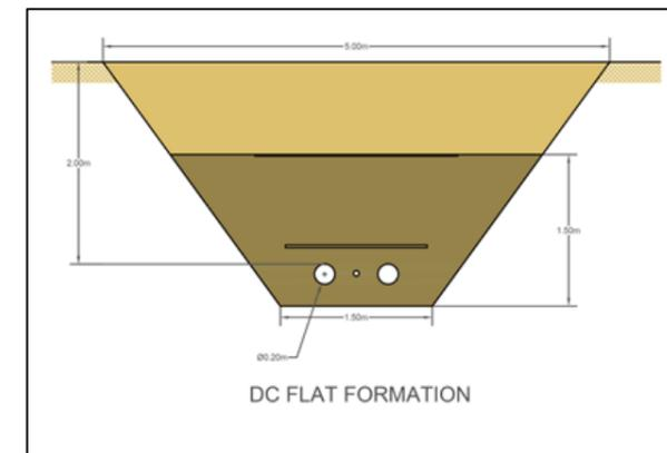
Figure 3.24: Onshore export cable HVDC trench layout.
