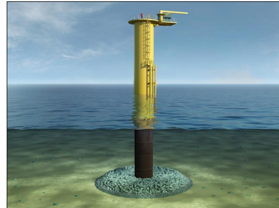
Figure 3.7: A monopile foundation and transition piece.
