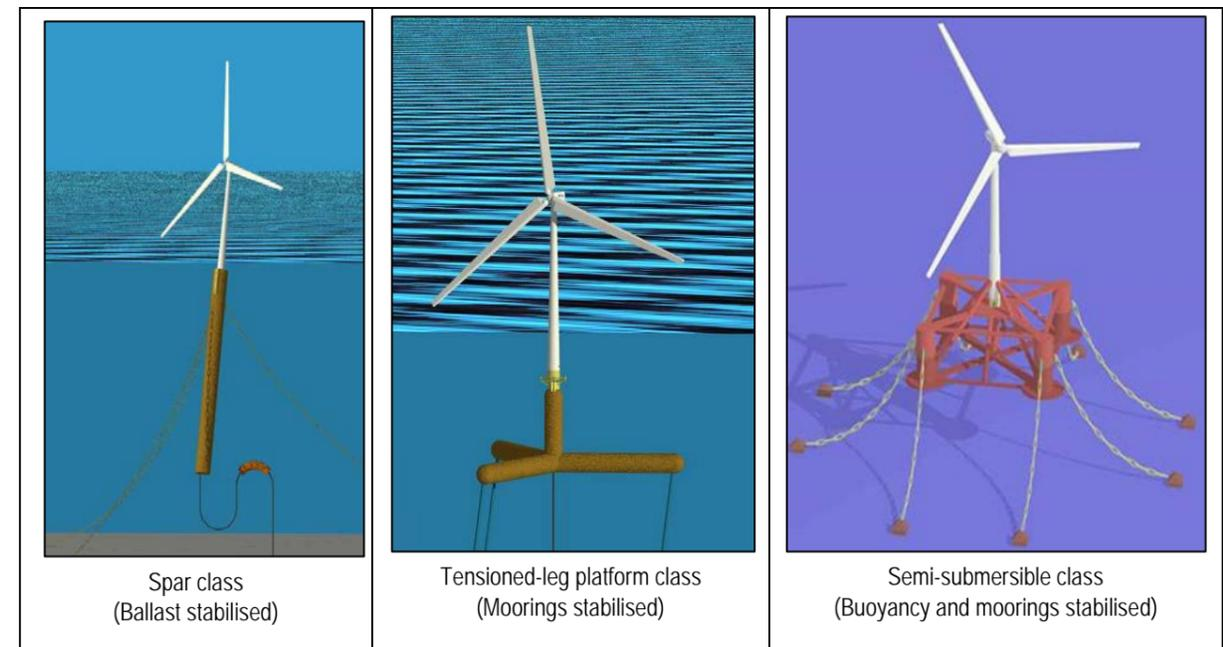
Figure 3.10: Examples of floating foundations.
