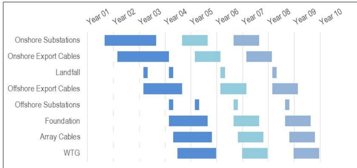
Figure 3.30: Indicative construction programme if project built out in three partially parallel phases.
