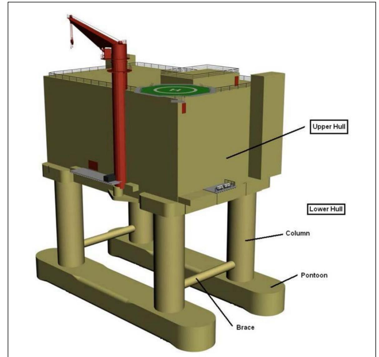
Figure 3.11: An example of a converter substation design supported by a Pontoon Gravity Base – pontoon gravity base – type 1.
