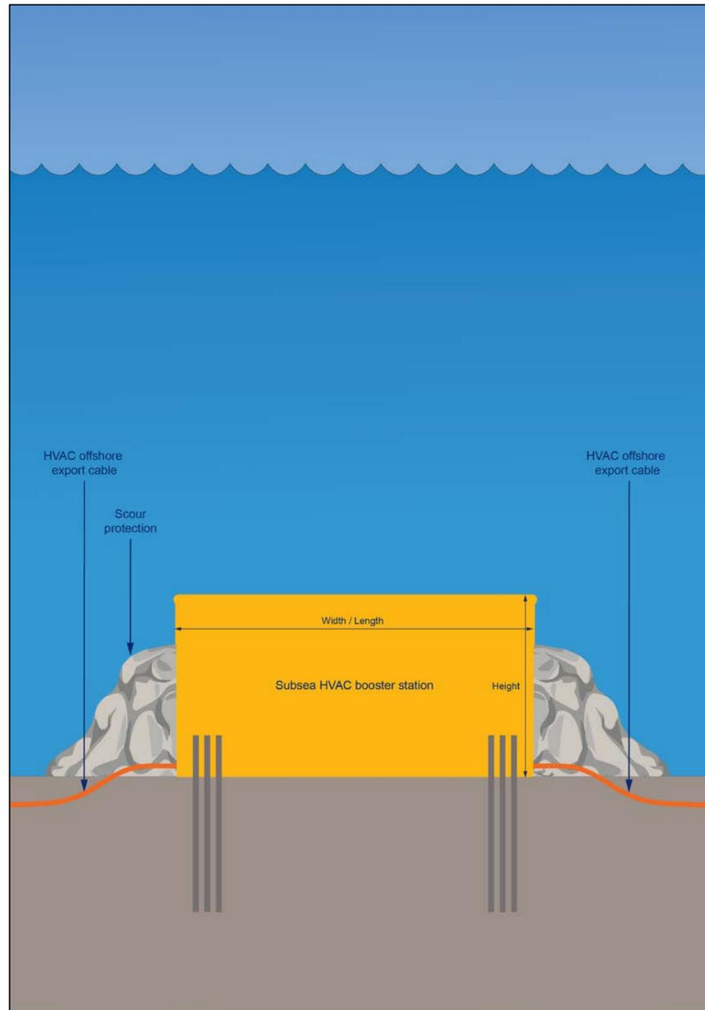
Figure 3.16: Illustration of subsea offshore HVAC booster station.
