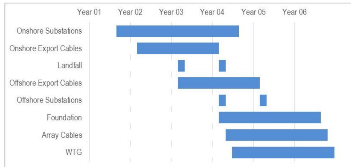
Figure 3.28: Indicative construction programme if project built out in a single phase.
