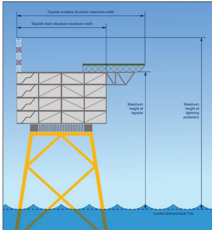
Figure 3.15: Schematic of an offshore transformer substation.
