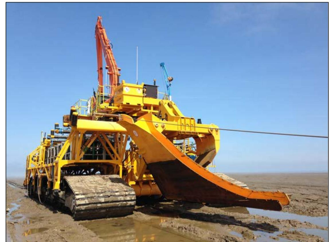
Figure 3.21: The 'sunfish' installation tool as used for cable installation at the Race Bank offshore wind farm.
