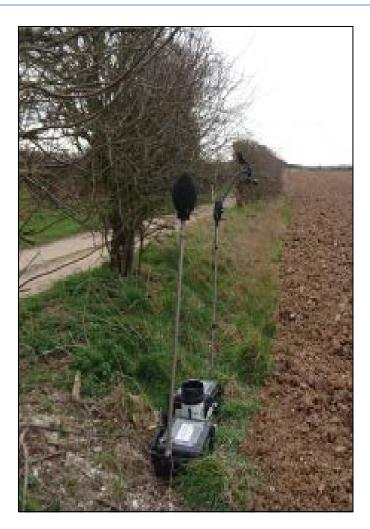
Figure 7.4: Noise monitoring equipment
