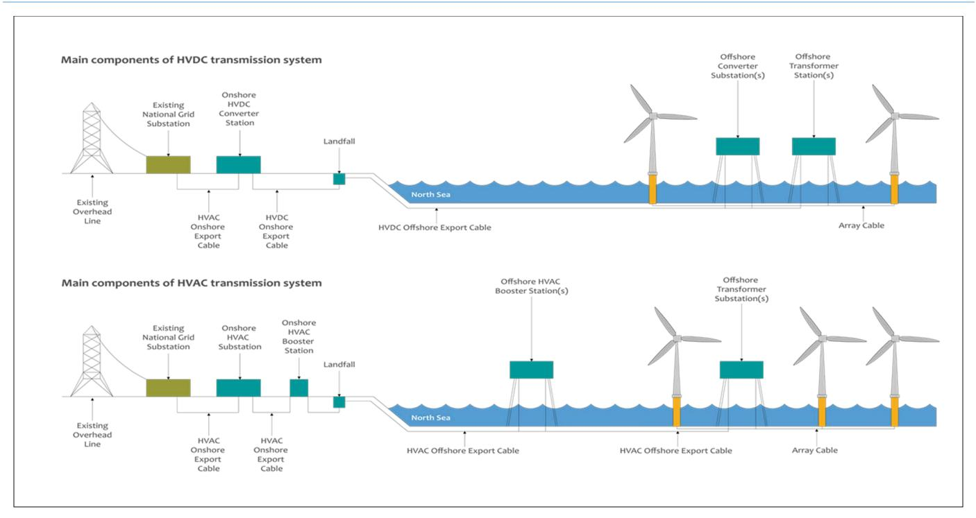
Figure 3.2: Main components of HVDC and HVAC transmission options for Hornsea Three.
