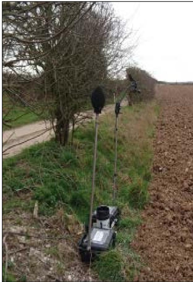
Figure 7.4: Noise monitoring equipment.
