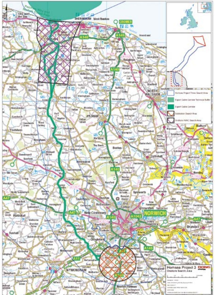
Figure 7: Map showing the original onshore export cable route search area with the indicative 200 m cable corridor (plus 100 m technical buffer either side) and substation/onshore HVAC booster station search areas.
