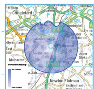
Figure 2: Heat map of the onshore substation search area. The darker shades indicate the more constrained areas.
