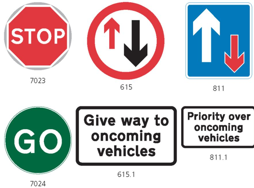
Figure 3.5: Manually Operated Stop/Go Signs and Priority Signs.
