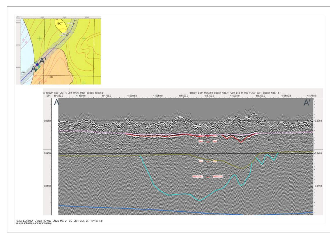
Figure 3.6: Sample section through channel on Hornsea Three offshore cable corridor.
