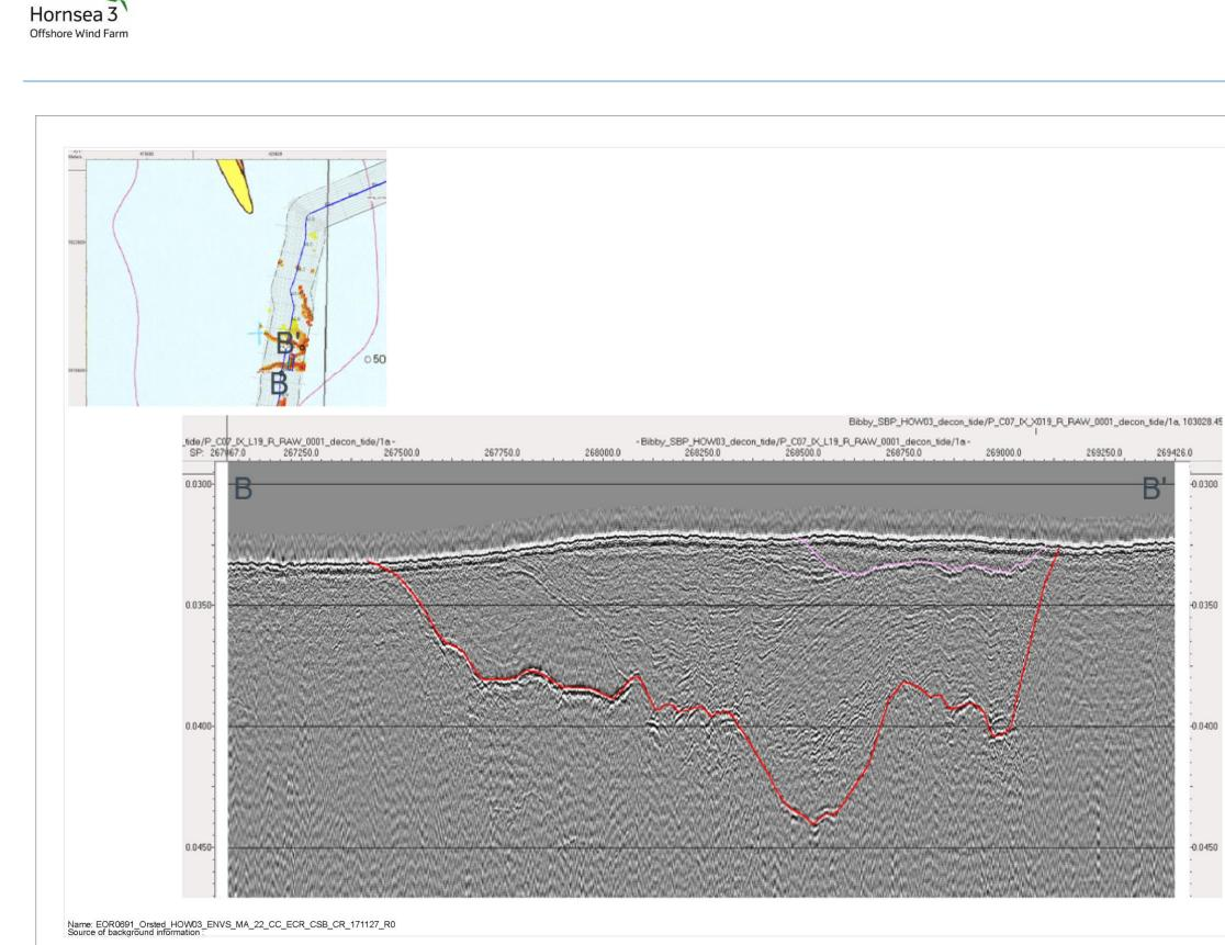
Figure 3.7: Sample section through channel on Hornsea Three offshore cable corridor.
