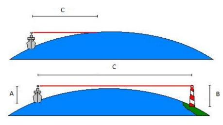
Figure 19.1: Determining Radar range
