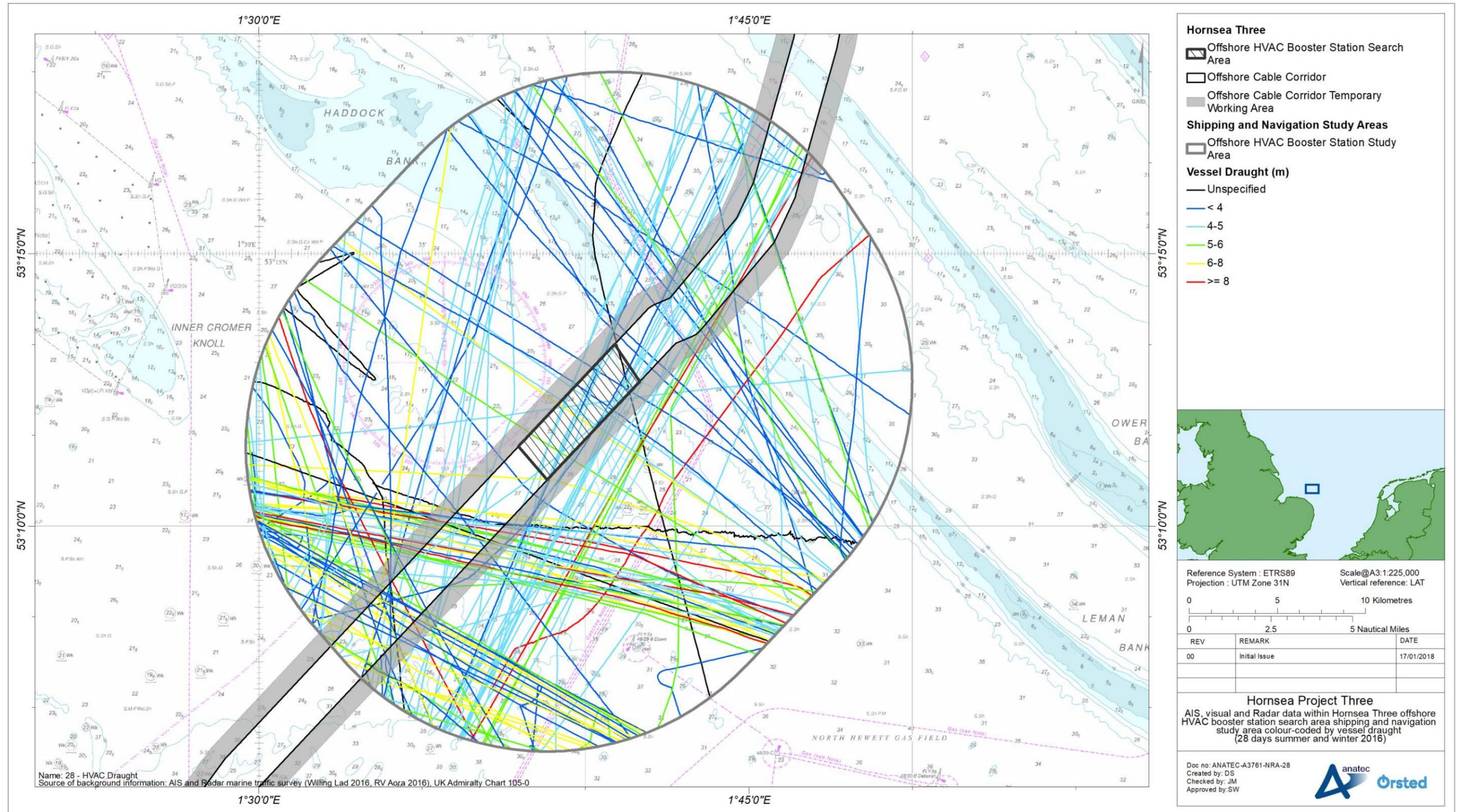
Figure 15.37: AIS, visual and Radar data within the Hornsea Three offshore HVAC booster station search area shipping and navigation study area colour-coded by vessel draught (28 days summer and winter 2016).
