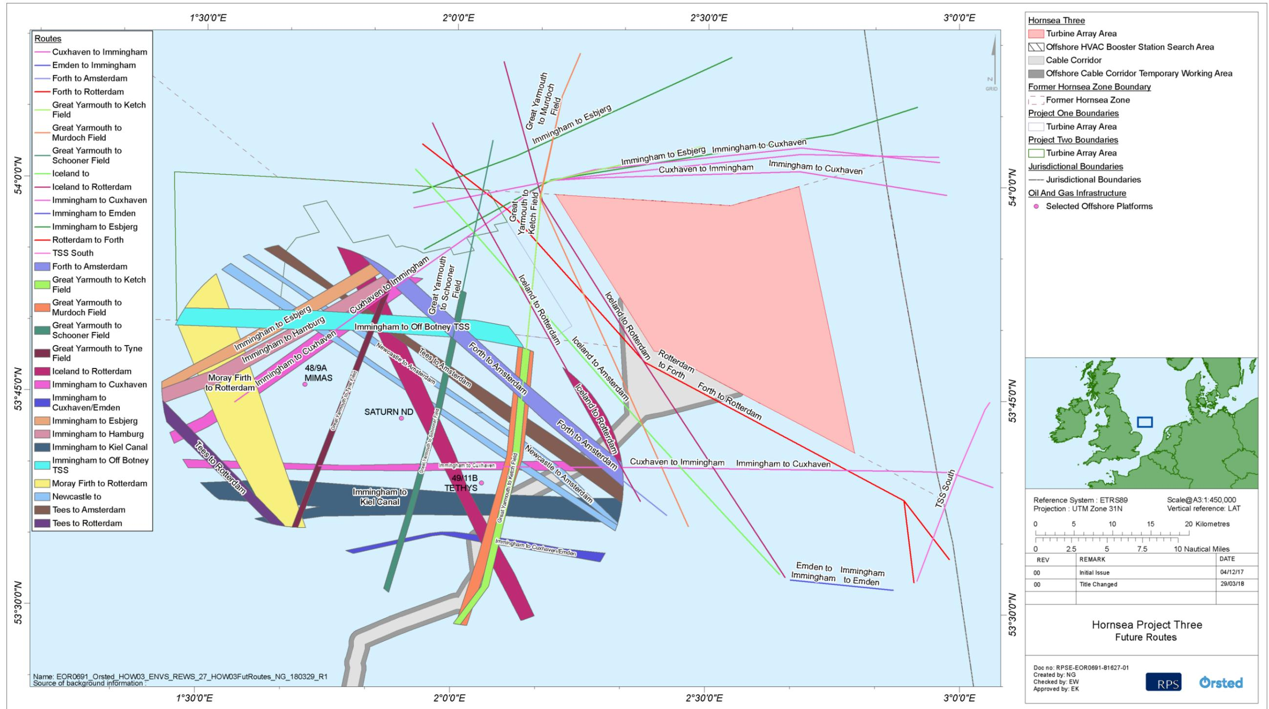
Figure 6.3 Predicted rerouted traffic around Hornsea Three in isolation.
