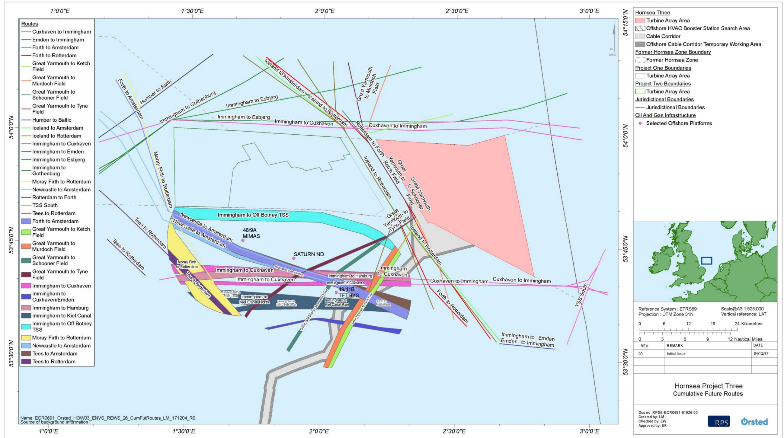
Figure 6.5: Predicted shipping re-routes around Hornsea Three considered cumulatively with Hornsea Projects One and Hornsea Project Two.
