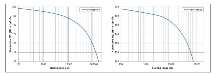
Figure 5.22: Total received cumulative SEL for species of fish (Popper *et al.* (2014) unweighted criteria) when fleeing from impact piling noise at NW location for a monopile installed with a maximum hammer energy of 5,000 kJ (Left plot = WNW transect (290°), Right plot = SSW transect (190°)).
