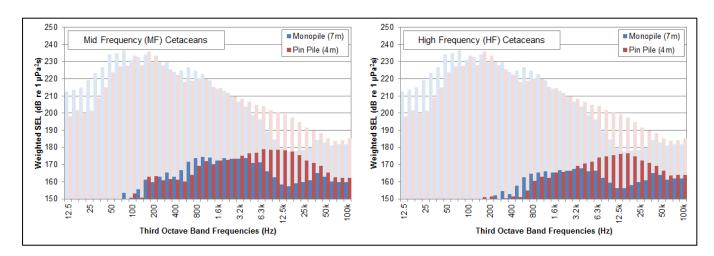
Figure 5.18: Filtered noise inputs for monopiles and pin piles using the MF cetacean and HF cetacean filters from NMFS (2016).
