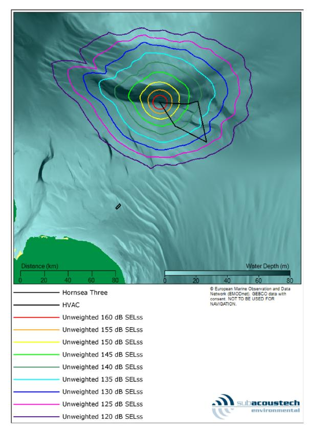
Figure 5.8: Contour plot showing the modelled unweighted SEL<sub>ss</sub> noise levels at the NW location for installing a pin pile with a maximum blow energy of 2500 kJ.
