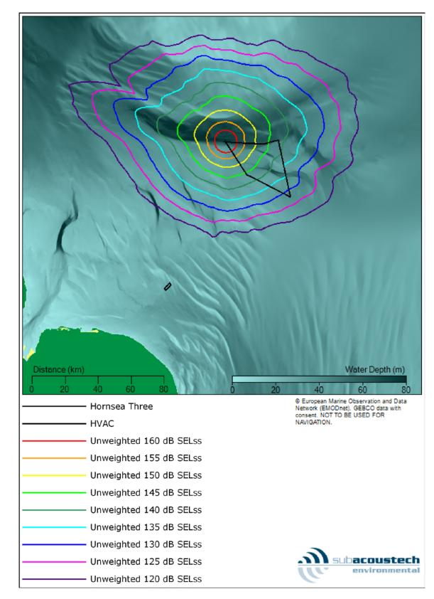
Figure 5.9: Contour plot showing the modelled unweighted SELss noise levels at the NW location for installing a monopile with a maximum blow energy of 3500 kJ.
