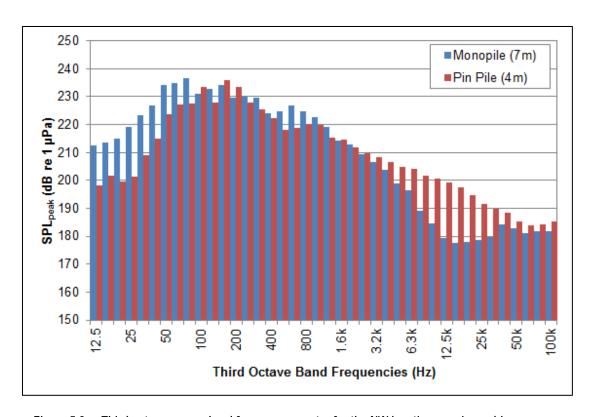
Figure 5.2: Third octave source level frequency spectra for the NW location, maximum blow energy.
