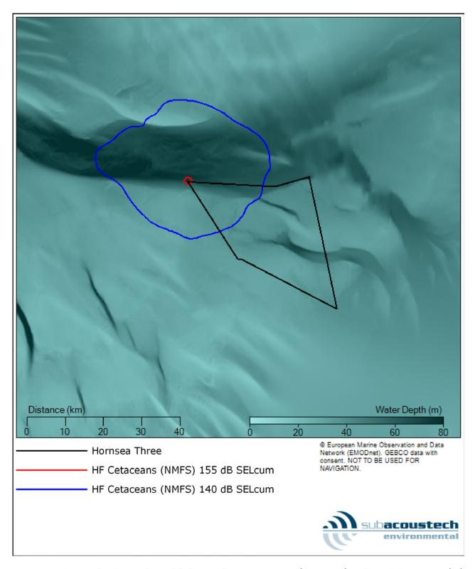
Figure 5.15: Contour plot showing the modelled PTS and TTS impact ranges (NMFS, 2016) for fleeing high frequency (HF) cetaceans at the NW location for installing a pin pile with a maximum blow energy of 2500 kJ.
