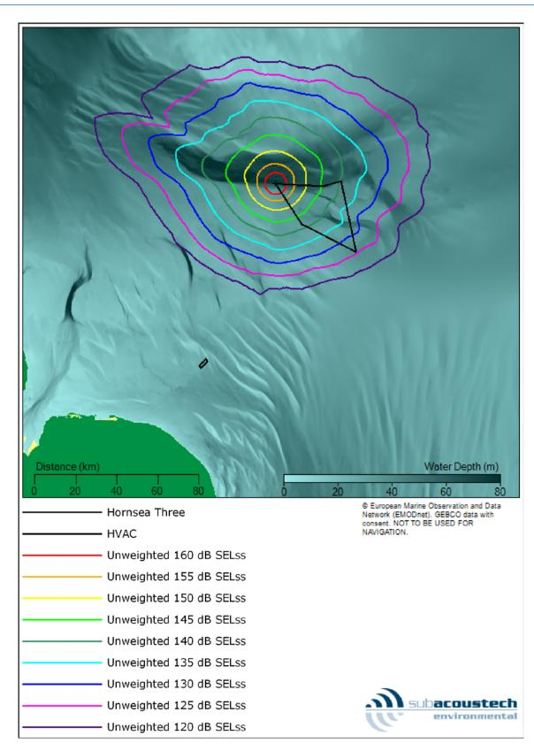
Figure 5.10: Contour plot showing the modelled unweighted SEL<sub>ss</sub> noise levels at the NW location for installing a monopile with a maximum blow energy of 2000 kJ.
