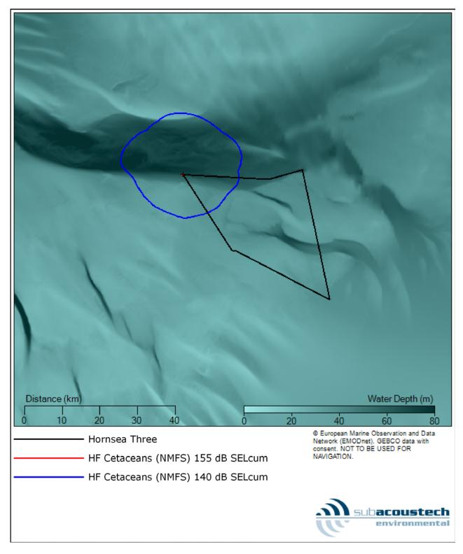
Figure 5.17: Contour plot showing the modelled PTS and TTS impact ranges (NMFS, 2016) for fleeing high frequency (HF) cetaceans at the NW location for installing a pin pile with a Most Likely maximum blow energy of 1750 kJ.
