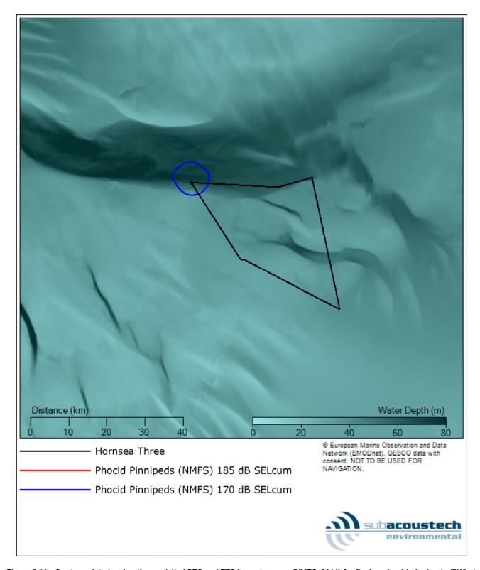
Figure 5.16: Contour plot showing the modelled PTS and TTS impact ranges (NMFS, 2016) for fleeing phocid pinnipeds (PW) at the NW location for installing a pin pile with a maximum blow energy of 2500 kJ. Note the 185 dB contour is too small to be visible at this scale.
