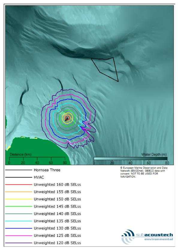
Figure 5.6: Contour plot showing the modelled unweighted SELss noise levels at the HVAC N location for installing a monopile with a maximum blow energy of 5000 kJ.
