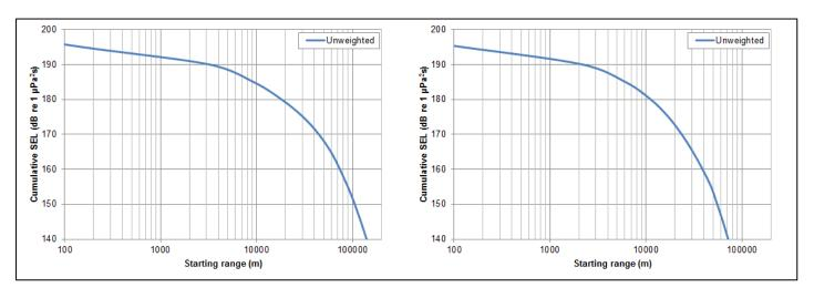
Figure 5.23: Total received cumulative SEL for species of fish (Popper *et al.* (2014) unweighted criteria) when fleeing from impact piling noise at NW location for a monopile installed with a maximum hammer energy of 3500 kJ (Left plot = WNW transect (290°), Right plot = SSW transect (190°)).
