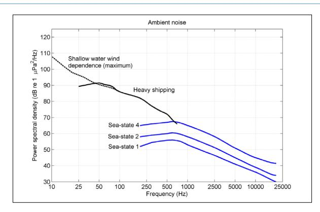
Figure 4.1: Ambient underwater noise as shown in Wenz (1962) showing frequency dependency from different noise sources.
