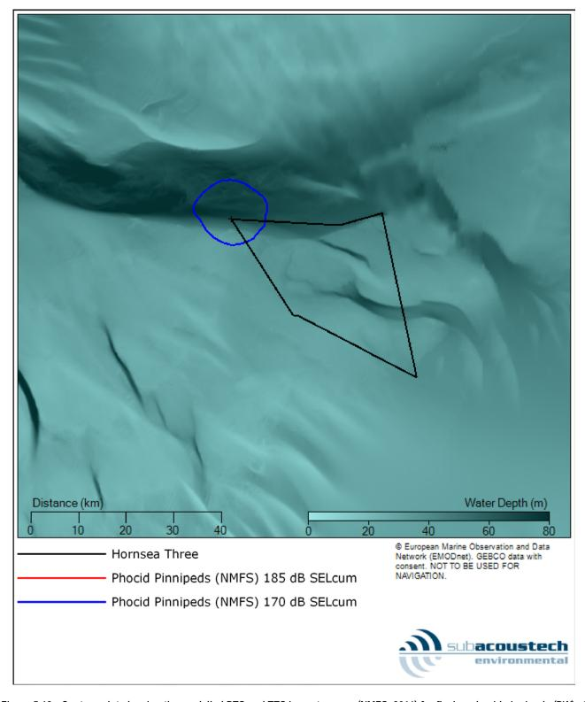
Figure 5.13: Contour plot showing the modelled PTS and TTS impact ranges (NMFS, 2016) for fleeing phocid pinnipeds (PW) at the NW location for installing a monopile with a maximum blow energy of 5000 kJ. Note the 185 dB contour is too small to be visible at this scale.
