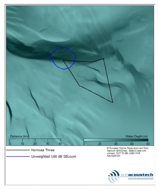
Figure 5.19: Contour plot showing the unweighted SEL<sub>cum</sub> TTS impact ranges (Popper et al. 2014) for fleeing fish at the NW location for installing a monopile with a maximum blow energy of 5000 kJ.
