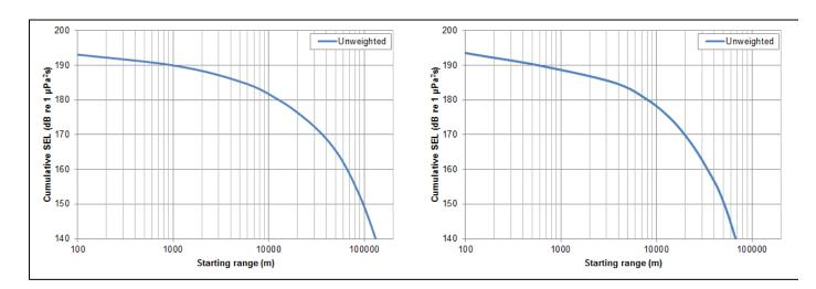
Figure 5.25: Total received cumulative SEL for species of fish (Popper *et al.* (2014) unweighted criteria) when fleeing from impact piling noise at NW location for a pin pile installed with a maximum hammer energy of 1,750 kJ (Left plot = WNW transect (290°), Right plot = SSW transect (190°)).
