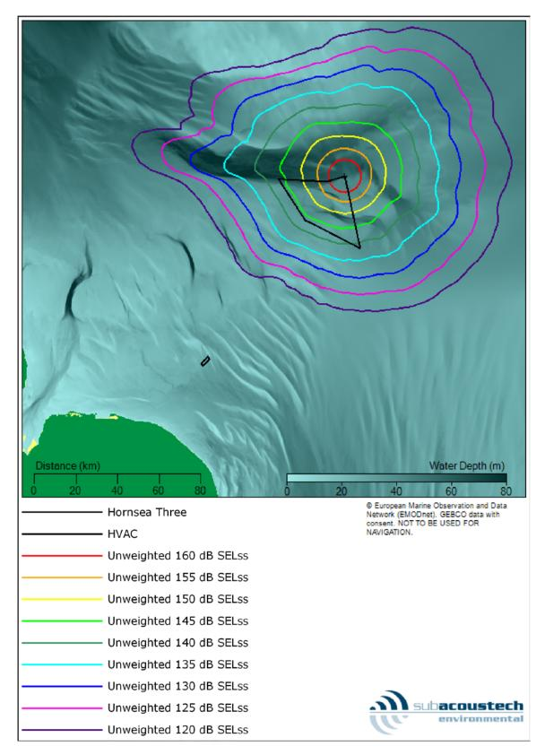
Figure 5.4: Contour plot showing the modelled unweighted SELss noise levels at the NE location for installing a monopile with a maximum blow energy of 5000 kJ.
