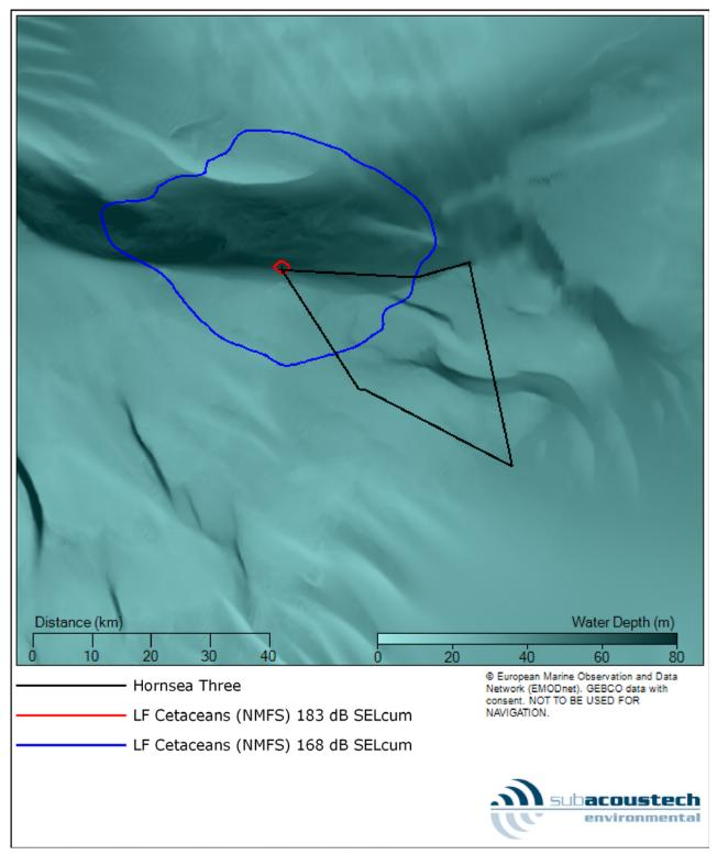
Figure 5.11: Contour plot showing the modelled PTS and TTS impact ranges (NMFS, 2016) for fleeing low frequency (LF) cetaceans at the NW location for installing a monopile with a maximum blow energy of 5000 kJ.
