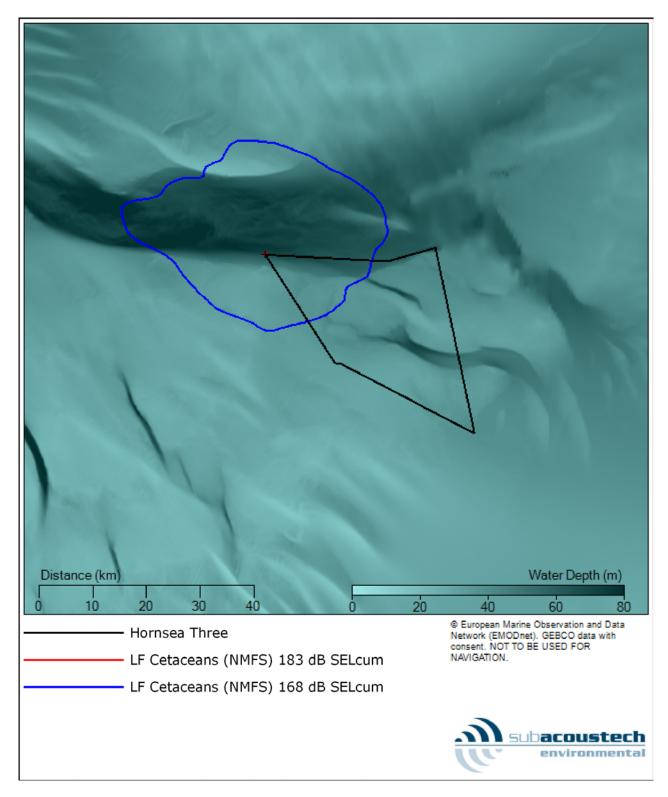
Figure 5.14: Contour plot showing the modelled PTS and TTS impact ranges (NMFS, 2016) for fleeing low frequency (LF) cetaceans at the NW location for installing a pin pile with a maximum blow energy of 2500 kJ.
