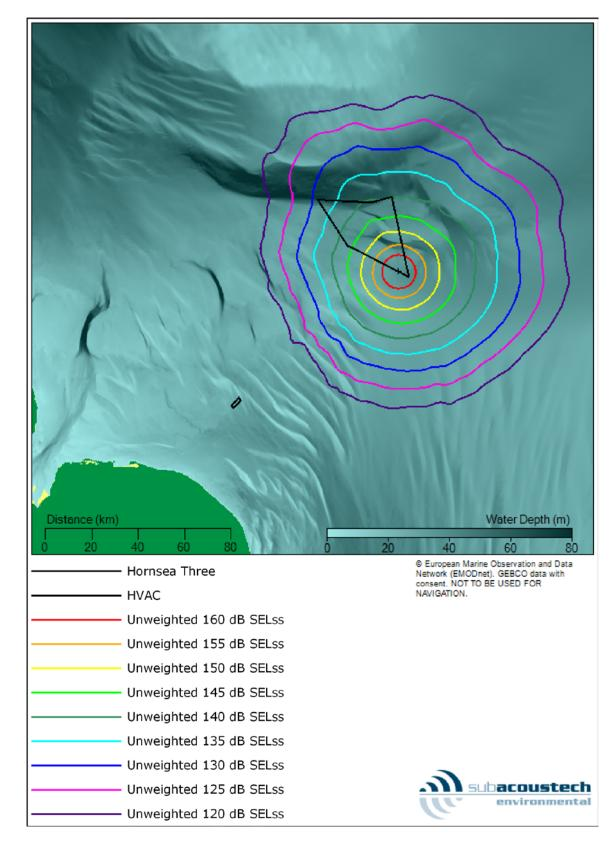
Figure 5.5: Contour plot showing the modelled unweighted SELss noise levels at the S location for installing a monopile with a maximum blow energy of 5000 kJ.
