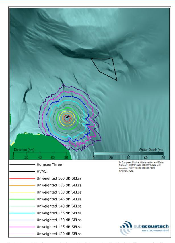
Figure 5.7: Contour plot showing the modelled unweighted SELss noise levels at the HVAC S location for installing a monopile with a maximum blow energy of 5000 kJ.
