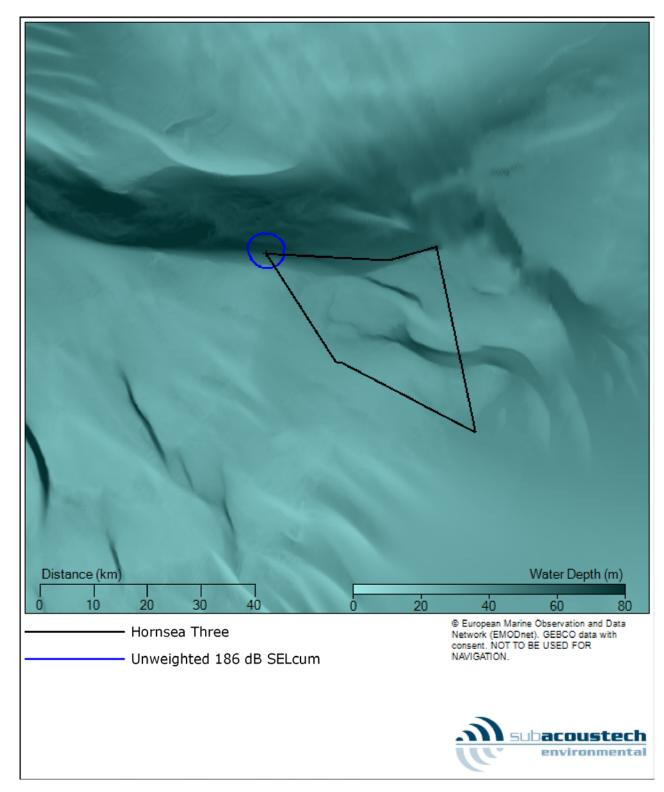
Figure 5.21: Contour plot showing the unweighted SEL<sub>cum</sub> TTS impact ranges (Popper et al. 2014) for fleeing fish at the NW location for installing a pin pile with a maximum blow energy of 1750 kJ.
