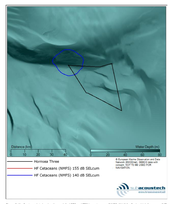
Figure 5.12: Contour plot showing the modelled PTS and TTS impact ranges (NMFS, 2016) for fleeing high frequency (HF) cetaceans at the NW location for installing a monopile with a maximum blow energy of 5000 kJ. Note the 155 dB contour is too small to be visible at this scale.
