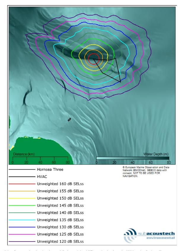
Figure 5.3: Contour plot showing the modelled unweighted SELss noise levels at the NW location for installing a monopile with a maximum blow energy of 5000 kJ.
