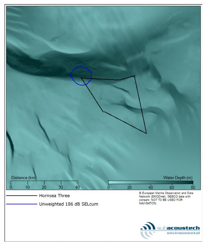
Figure 5.20: Contour plot showing the unweighted SEL<sub>cum</sub> TTS impact ranges (Popper et al. 2014) for fleeing fish at the NW location for installing a pin pile with a maximum blow energy of 2500 kJ.
