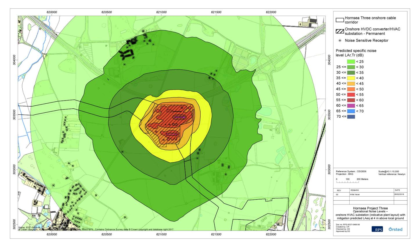
Figure 8.2: Operational noise levels - onshore HVAC substation (indicative plant layout) with mitigation predicted LAr, Tr at 4m above local ground.
