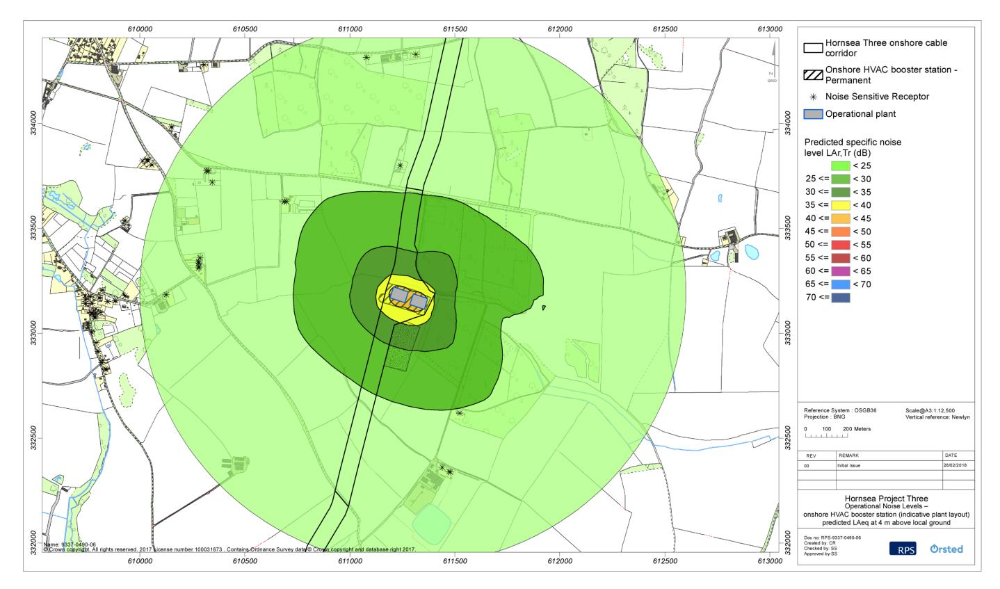
Figure 8.3: Operational noise levels – onshore HVAC booster station (indicative plant layout) predicted LAeq at 4 m above local ground.
