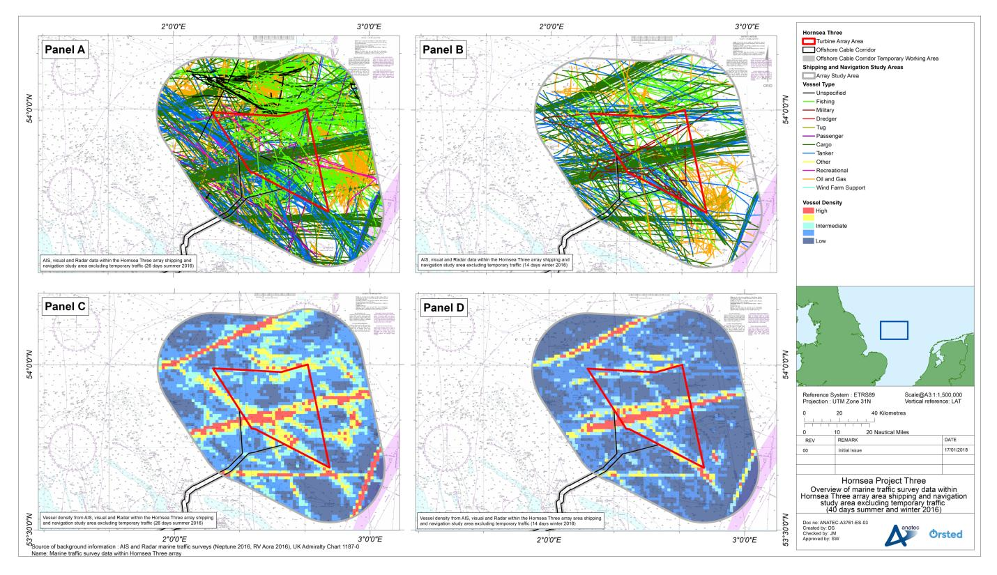
Figure 7.3: Overview of marine traffic survey data within the Hornsea Three array area shipping and navigation study area excluding temporary traffic (40 days summer and winter 2016).
