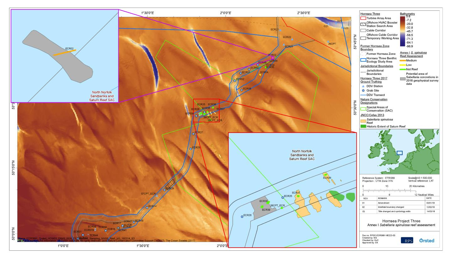
Figure 2.6: The Hornsea Three offshore cable corridor and historic extents of Annex I S. spinulosa reefs within the North Norfolk Sandbanks and Saturn Reef SAC, together with the results of the Hornsea Three site specific survey S. spinulosa reefiness assessments.
