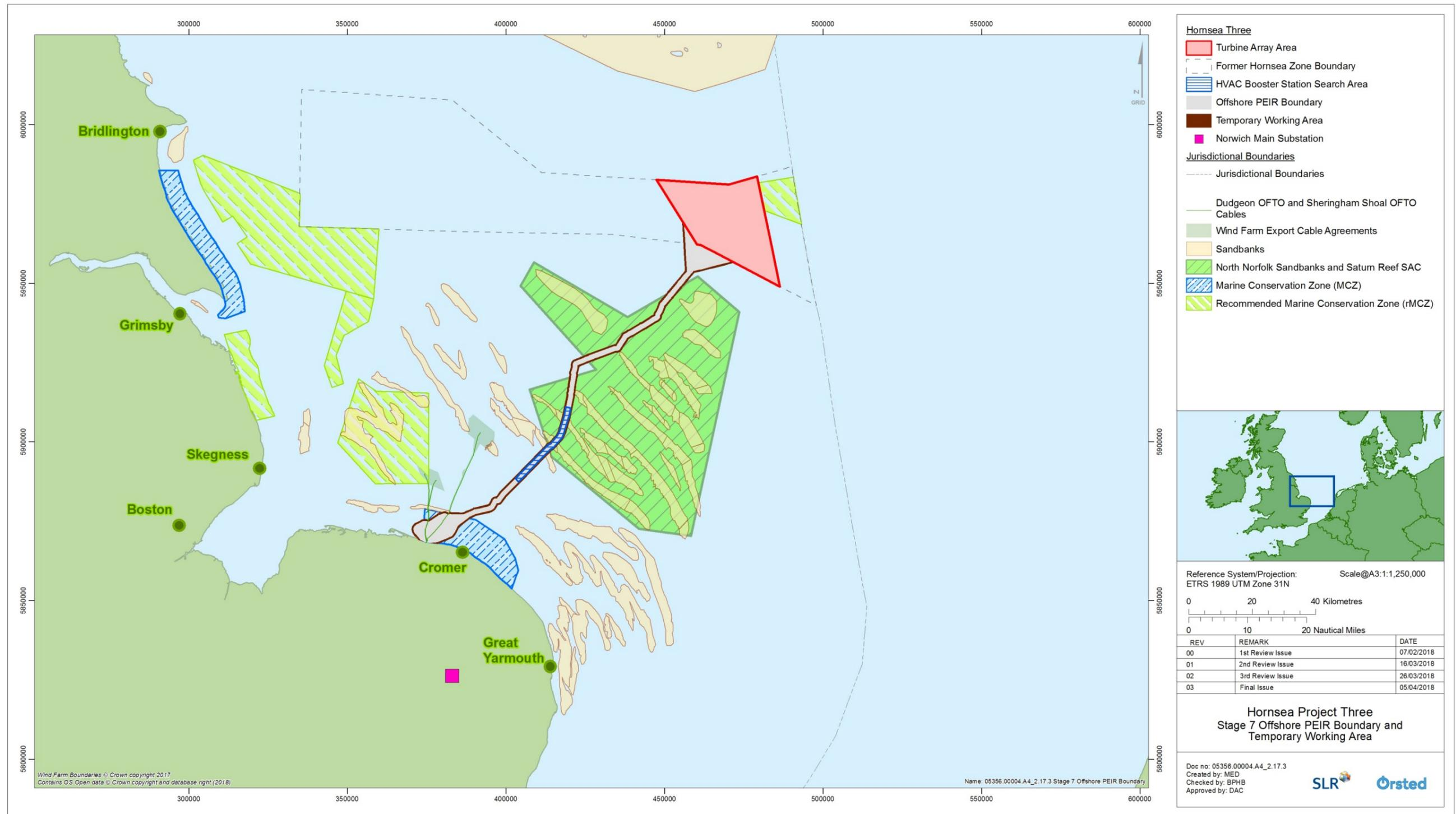
Figure 4.8: Refined offshore cable corridor and offshore HVAC booster station search area.
