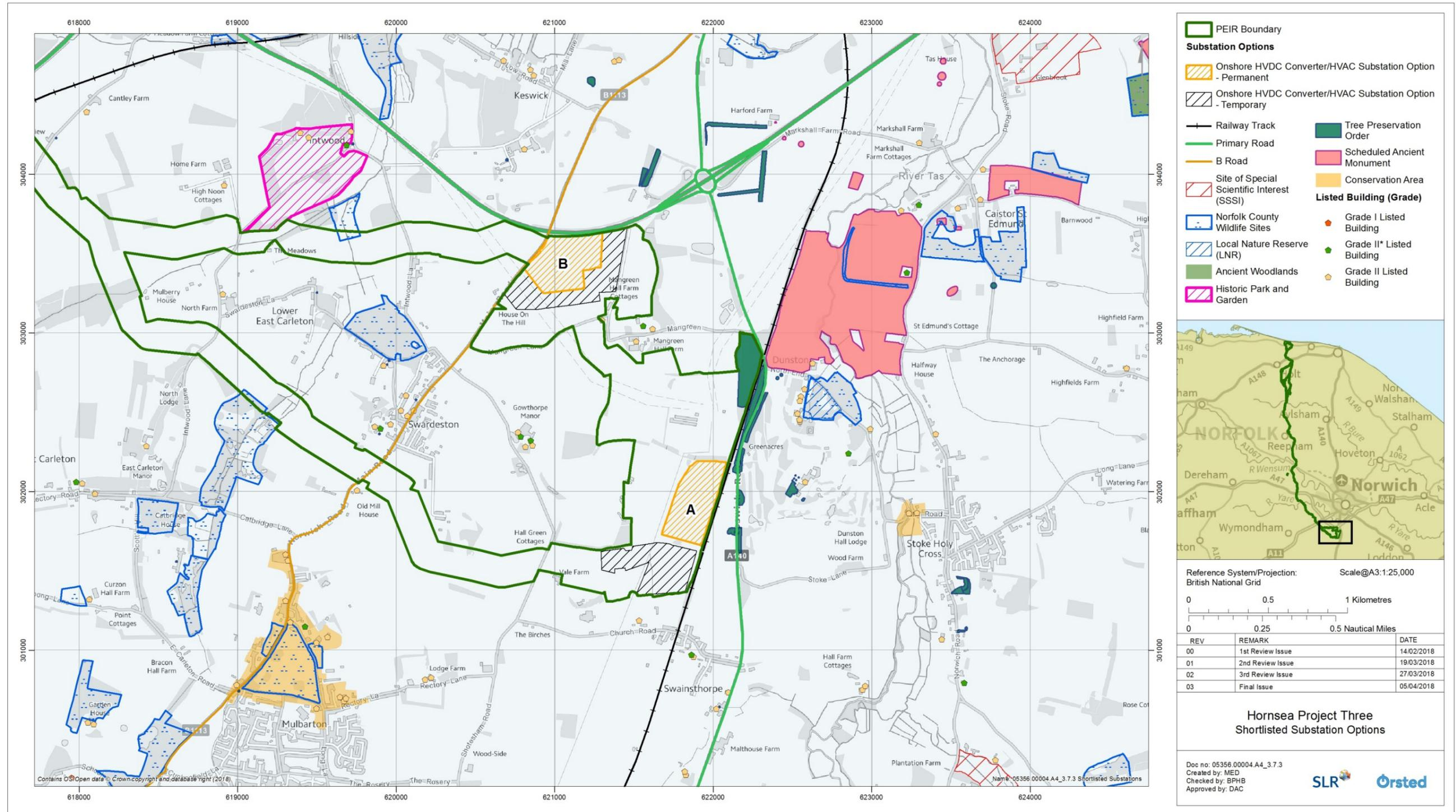
Figure 4.16: Overview of onshore HVDC converter/HVAC substation options.
