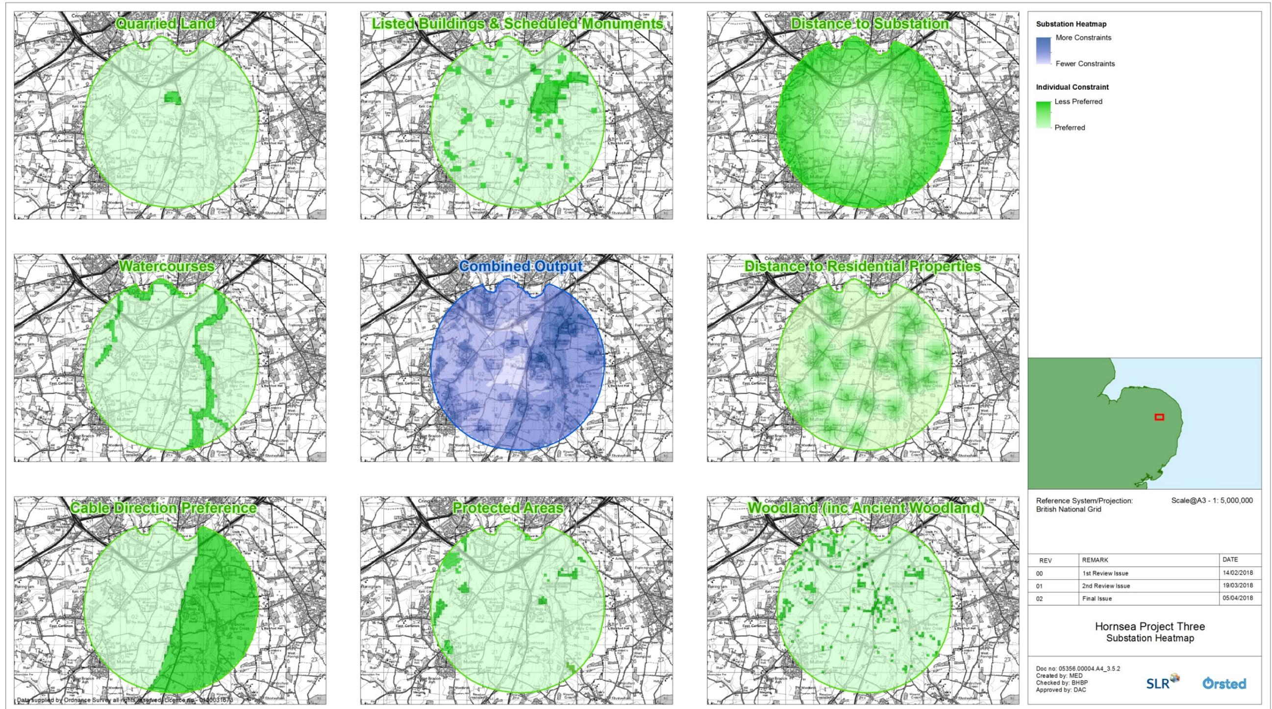
Figure 4.15: Constraints mapping of onshore HVDC converter/HVAC substation search area.
