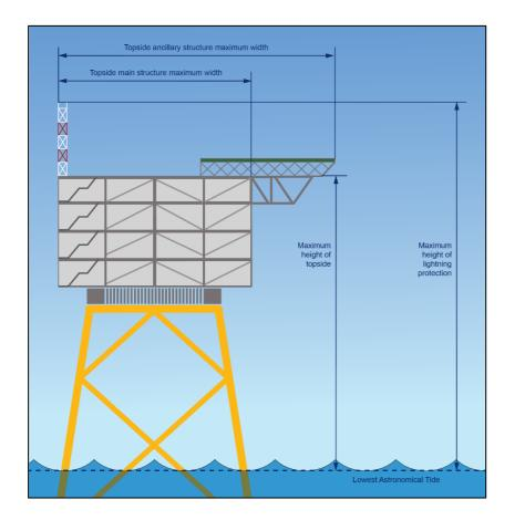
Figure 3.18: Schematic of an offshore transformer substation.
