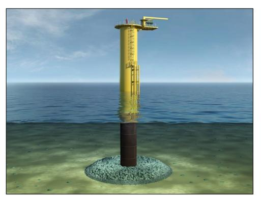
Figure 3.11: A monopile foundation and transition piece.
