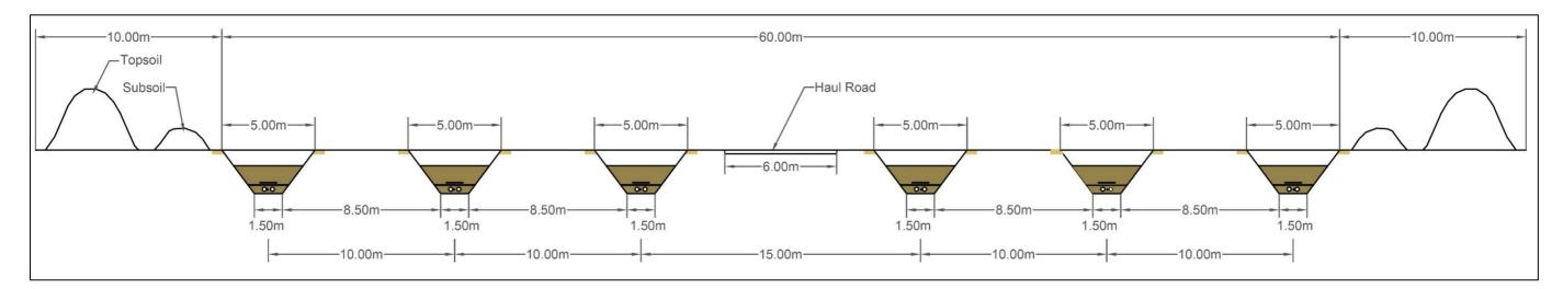
Figure 3.32: Onshore export cable corridor indicative layout showing the maximum of 6 onshore circuits.
