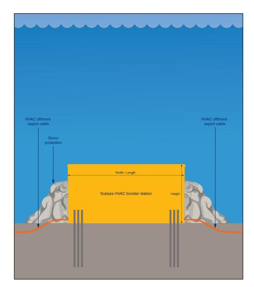
Figure 3.19: Illustration of an offshore subsea HVAC booster station.
