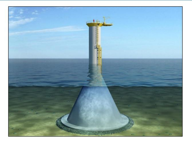
Figure 3.13: A gravity base foundation.
