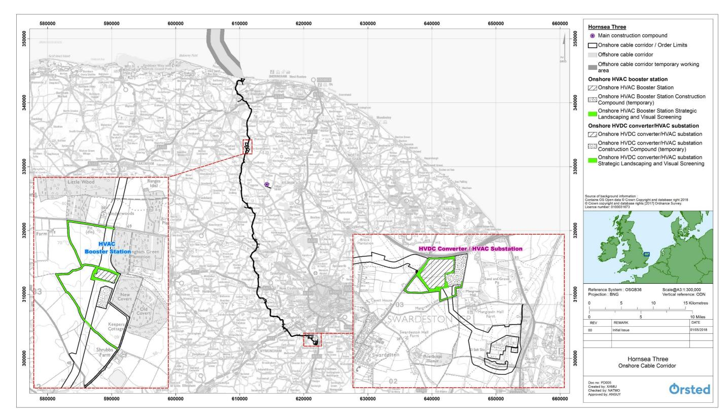
Figure 3.29: Hornsea Three onshore cable corridor and locations for onshore HVAC booster station and onshore HVDC converter/HVAC substation.
