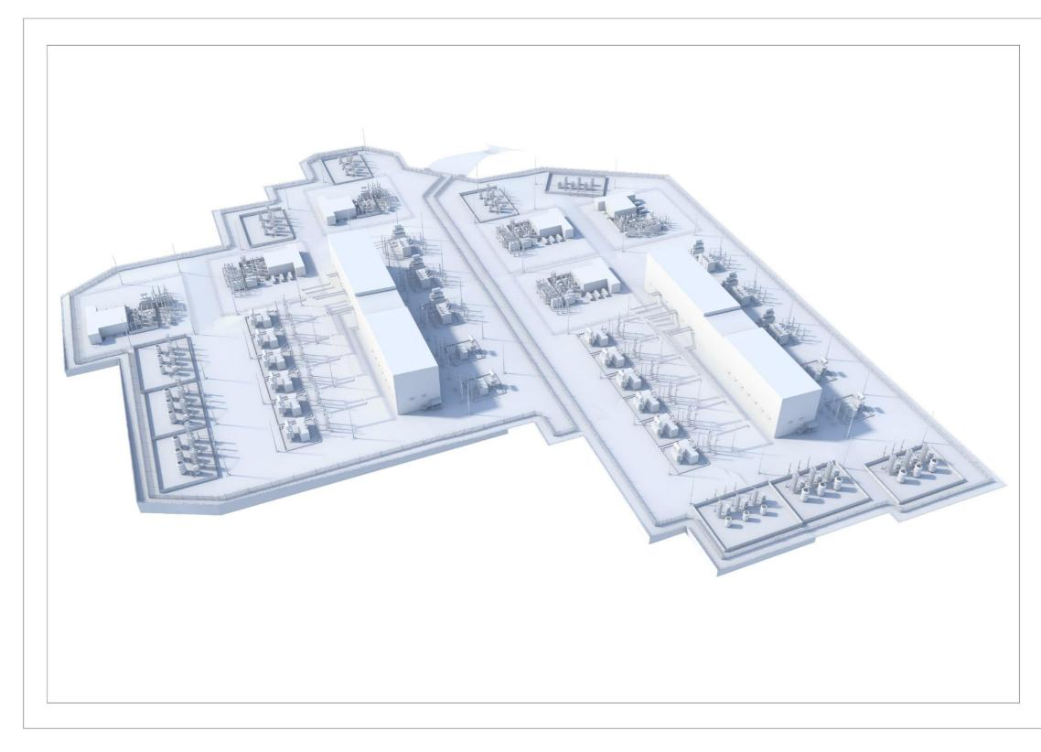
Figure 3.37: Indicative onshore HVDC converter/HVAC substation layout.
