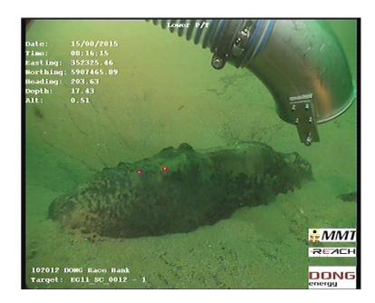
Figure 3.3: An example of a UXO following excavation.
