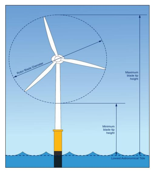
Figure 3.7: Schematic of an offshore wind turbine.
