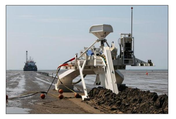
Figure 3.24: Example of a cable plough pulled from an installation vessel. (source: http://www.4coffshore.com/s/about/equipmentTypes.aspx)
