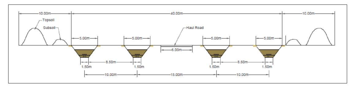
Figure 3.36: Grid connection export cable corridor indicative layout.
