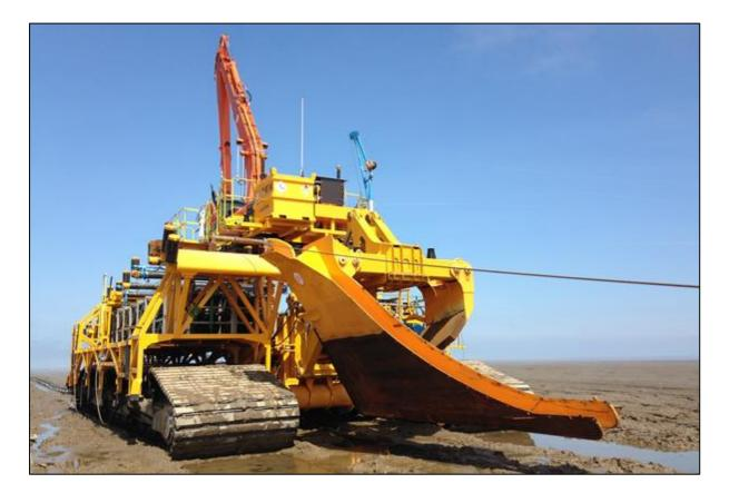
Figure 3.25: The 'sunfish' installation tool as used for cable installation at the Race Bank offshore wind farm.
