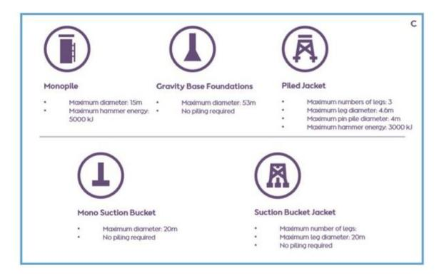
NOTE: Foundation dimensions are dependent on topside dimensions. Which in turn are dependent upon the design of the final topside, which is dependent upon the number of kittiwakes to be compensated
