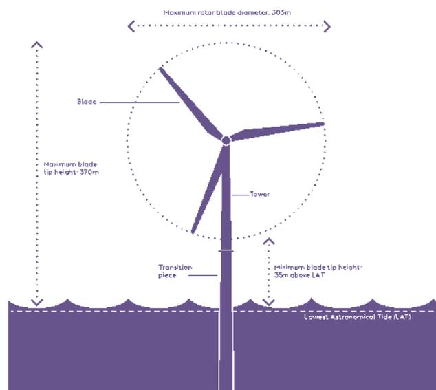
Figure 4: Typical Offshore Wind Turbine
