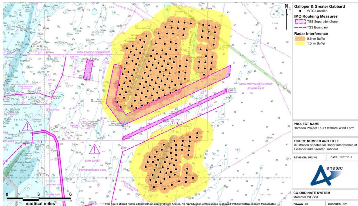
**Figure 18.3 Illustration of potential Radar interference at Greater Gabbard and Galloper Offshore Wind Farms**
