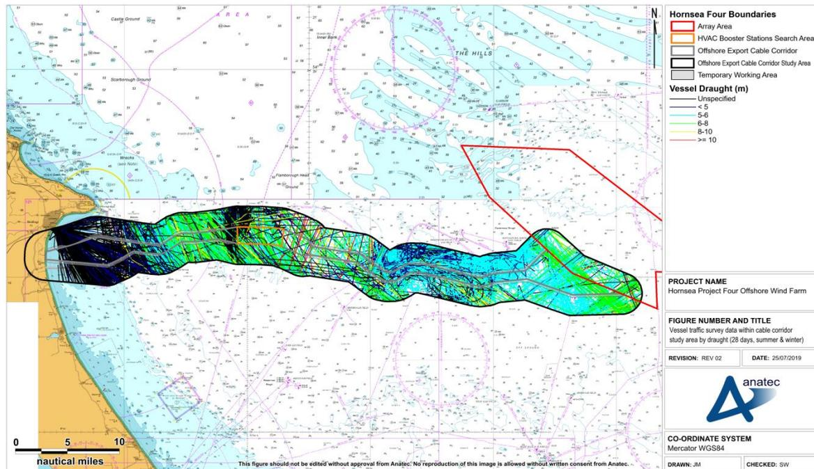
**Figure 15.30 Vessel traffic survey data within Hornsea Four offshore ECC shipping and navigation study area colour-coded by vessel draught (28 days summer 2018 and winter 2019)**
