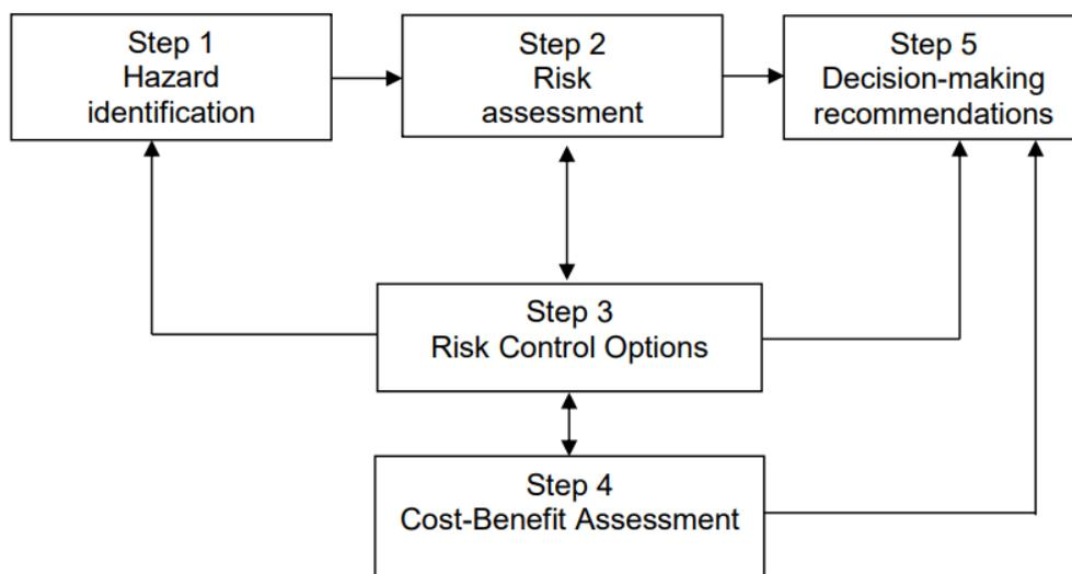
**Figure 3.1** Flow chart of the FSA methodology (IMO, 2018)
