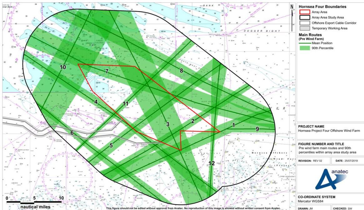
**Figure 15.16 Pre-wind farm main routes and 90<sup>th</sup> percentiles within Hornsea Four array area shipping and navigation study area**
