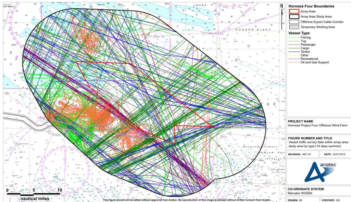
**Figure 15.1** Vessel traffic survey data within Hornsea Four array area shipping and navigation study area colour-coded by vessel type (14 days summer 2018)
