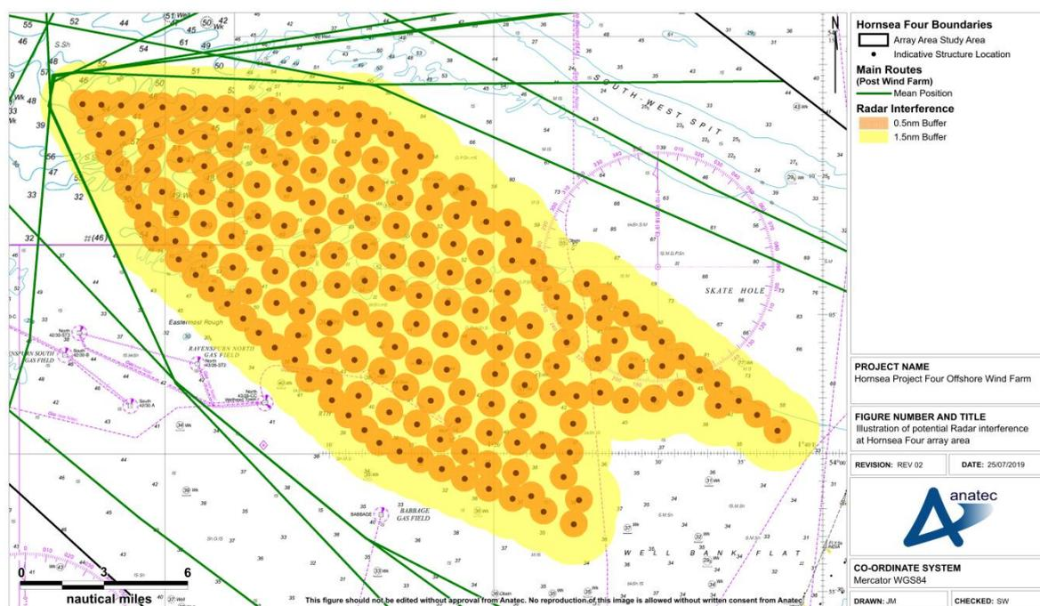
**Figure 18.4 Illustration of potential Radar interference at Hornsea Four array area**
