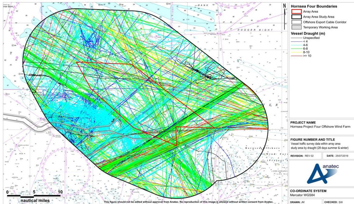
**Figure 15.14 Vessel traffic survey data within Hornsea Four array area shipping and navigation study area colour-coded by vessel draught (28 days summer 2018 and winter 2019)**
