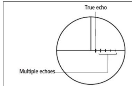
**Figure 18.2** Illustration of multiple reflected echoes on Radar screen
