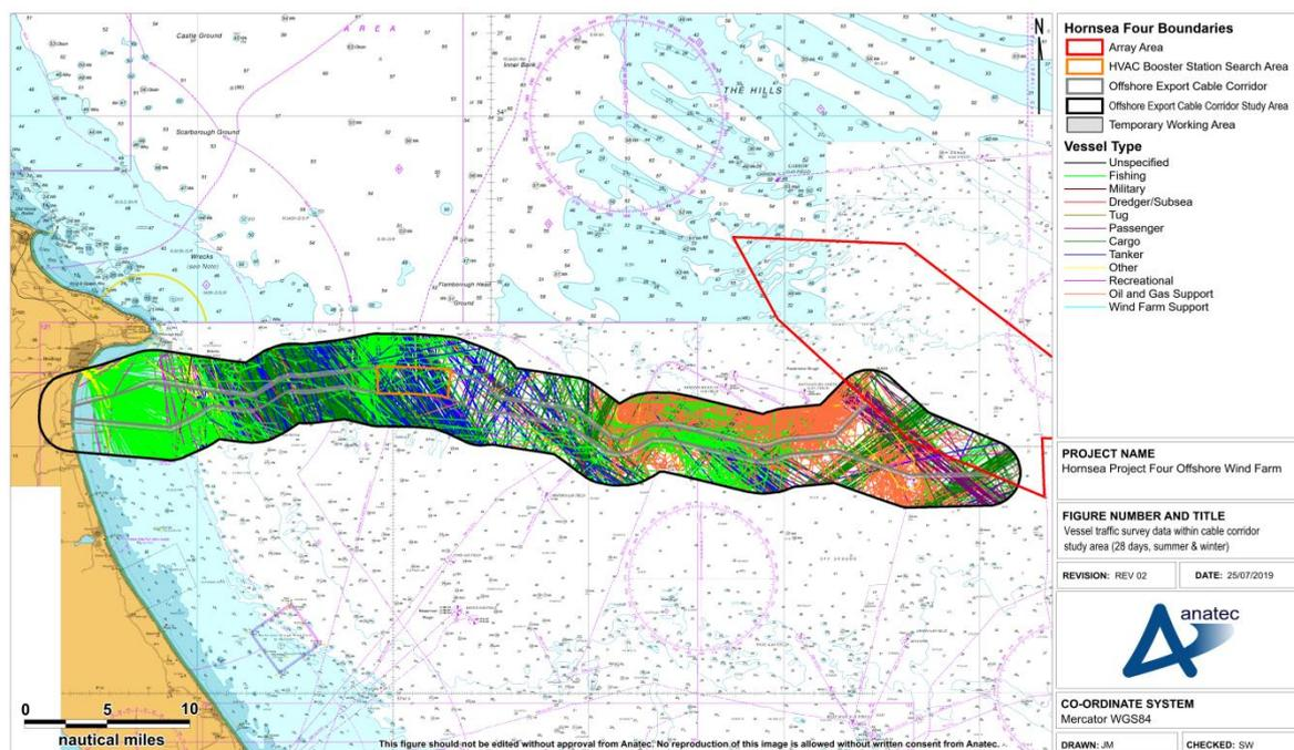
**Figure 15.20 Vessel traffic survey data within Hornsea Four offshore ECC shipping and navigation study area colour-coded by vessel type (28 days summer 2018 and winter 2019)**
