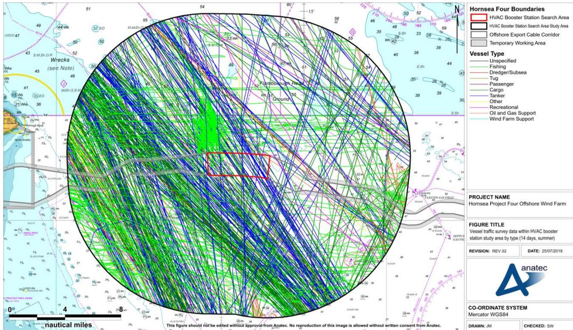
**Figure 15.34** Vessel traffic survey data within Hornsea Four HVAC booster station search area shipping and navigation study area colour-coded by vessel type (14 days summer 2018)
