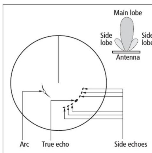
**Figure 18.1** Illustration of side lobes on Radar screen
