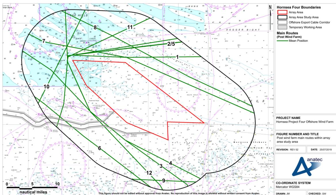
**Figure 17.1 Post wind farm main routes within Hornsea Four array area shipping and navigation study area**
