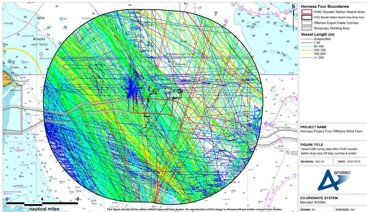
Figure 15.44 Vessel traffic survey data within Hornsea Four HVAC booster station search area shipping and navigation study area colour-coded by vessel length (28 days summer 2018 and winter 2019)
