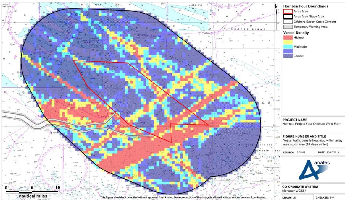
**Figure 15.4** Vessel traffic density heat map within Hornsea Four array area shipping and navigation study area excluding temporary traffic (14 days winter 2019)
