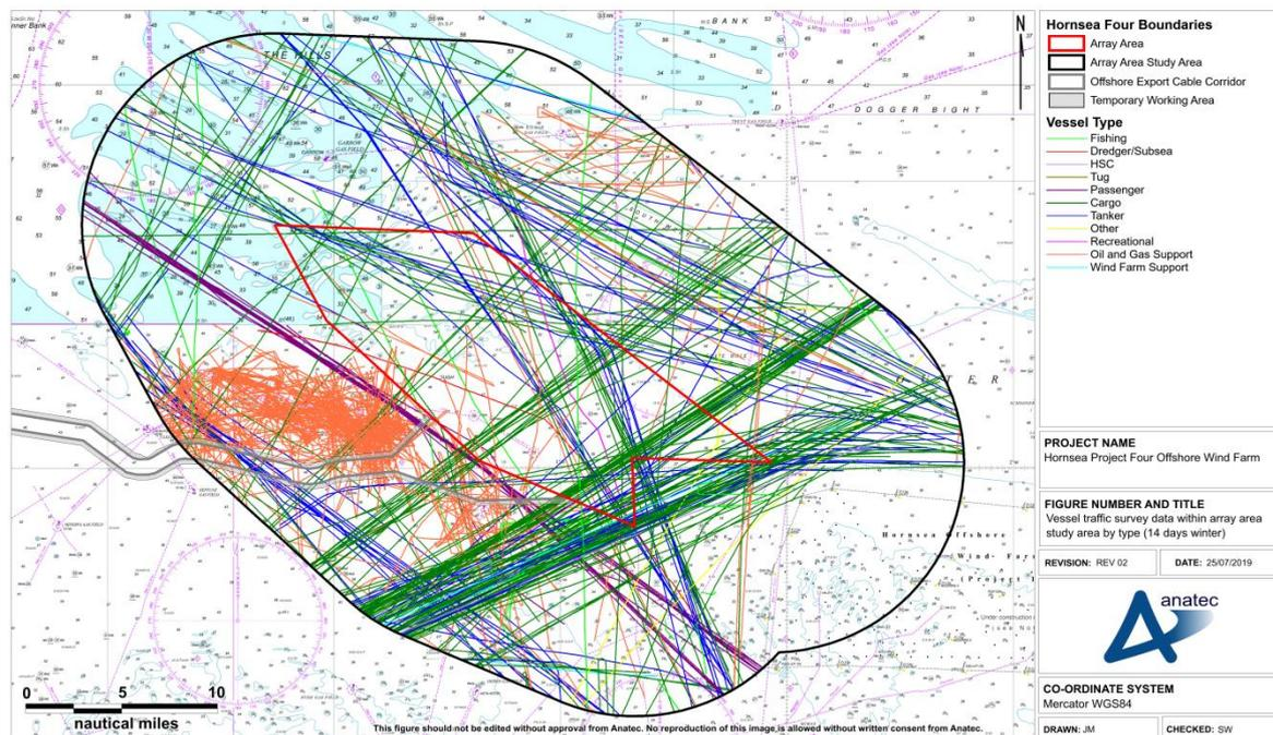
**Figure 15.2** Vessel traffic survey data within Hornsea Four array area shipping and navigation study area colour-coded by vessel type (14 days winter 2019)
