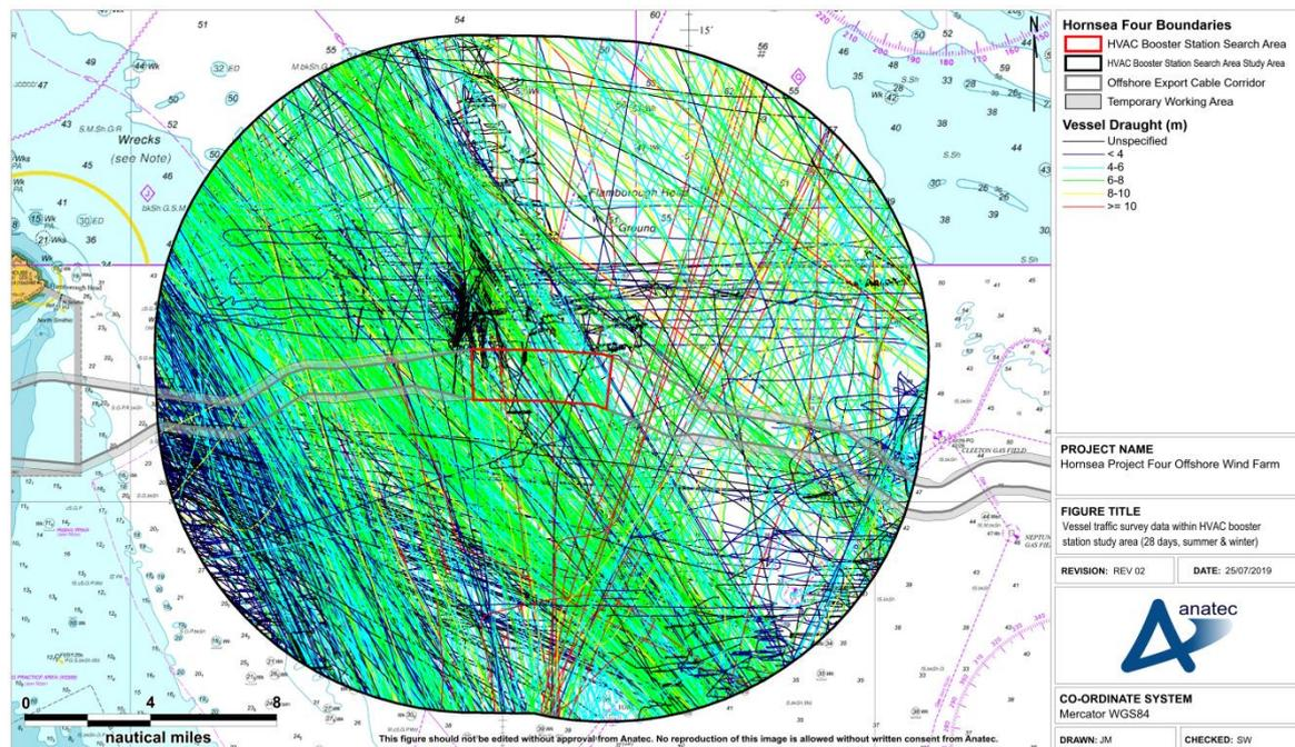
**Figure 15.46 Vessel traffic survey data within Hornsea Four HVAC booster station search area shipping and navigation study area colour-coded by vessel draught (28 days summer 2018 and winter 2019)**
