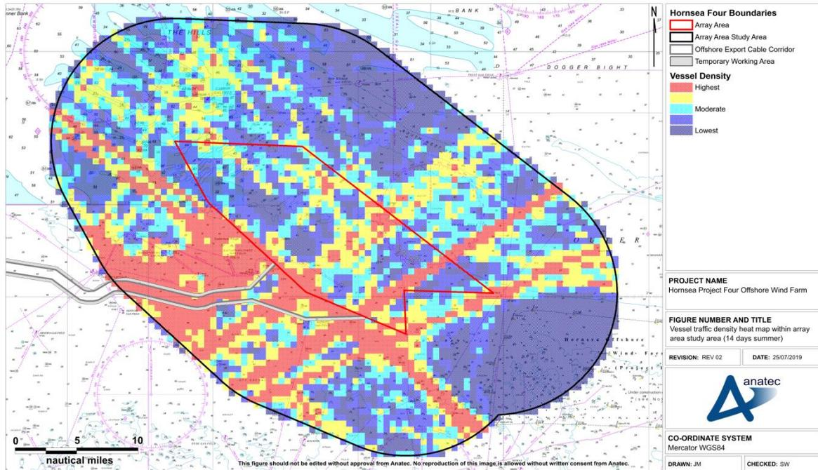
**Figure 15.3** Vessel traffic density heat map within Hornsea Four array area shipping and navigation study area excluding temporary traffic (14 days summer 2018)
