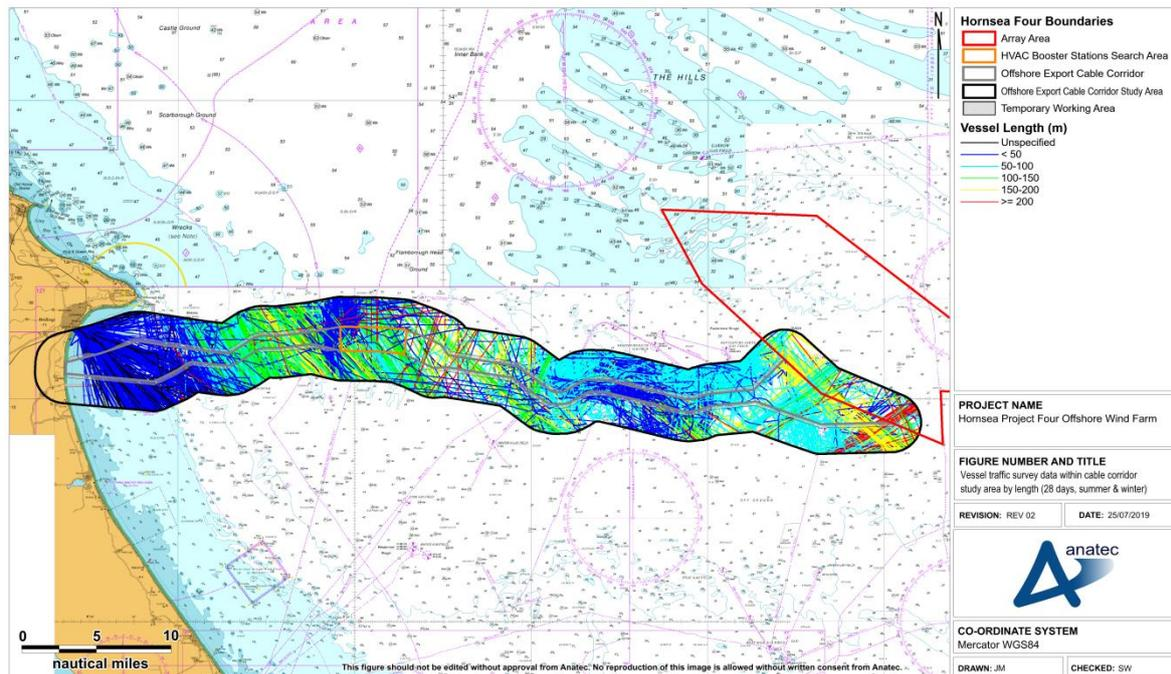
**Figure 15.28 Vessel traffic survey data within Hornsea Four offshore ECC shipping and navigation study area colour-coded by vessel length (28 days summer 2018 and winter 2019)**
