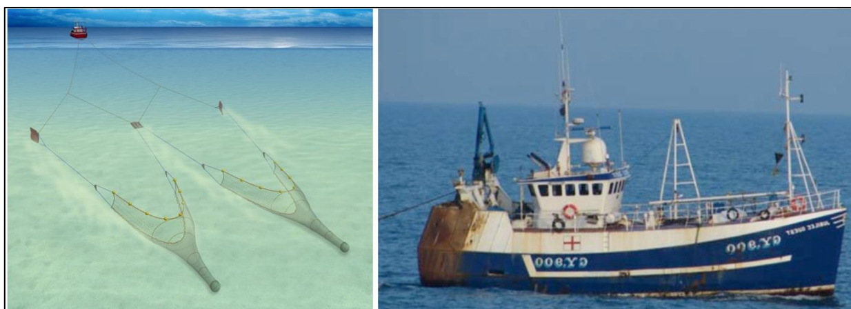
Figure 26: Typical demersal otter trawler vessel and gear diagram (Sources: Visserijnieuws, 2010; Seafish, 2019).
