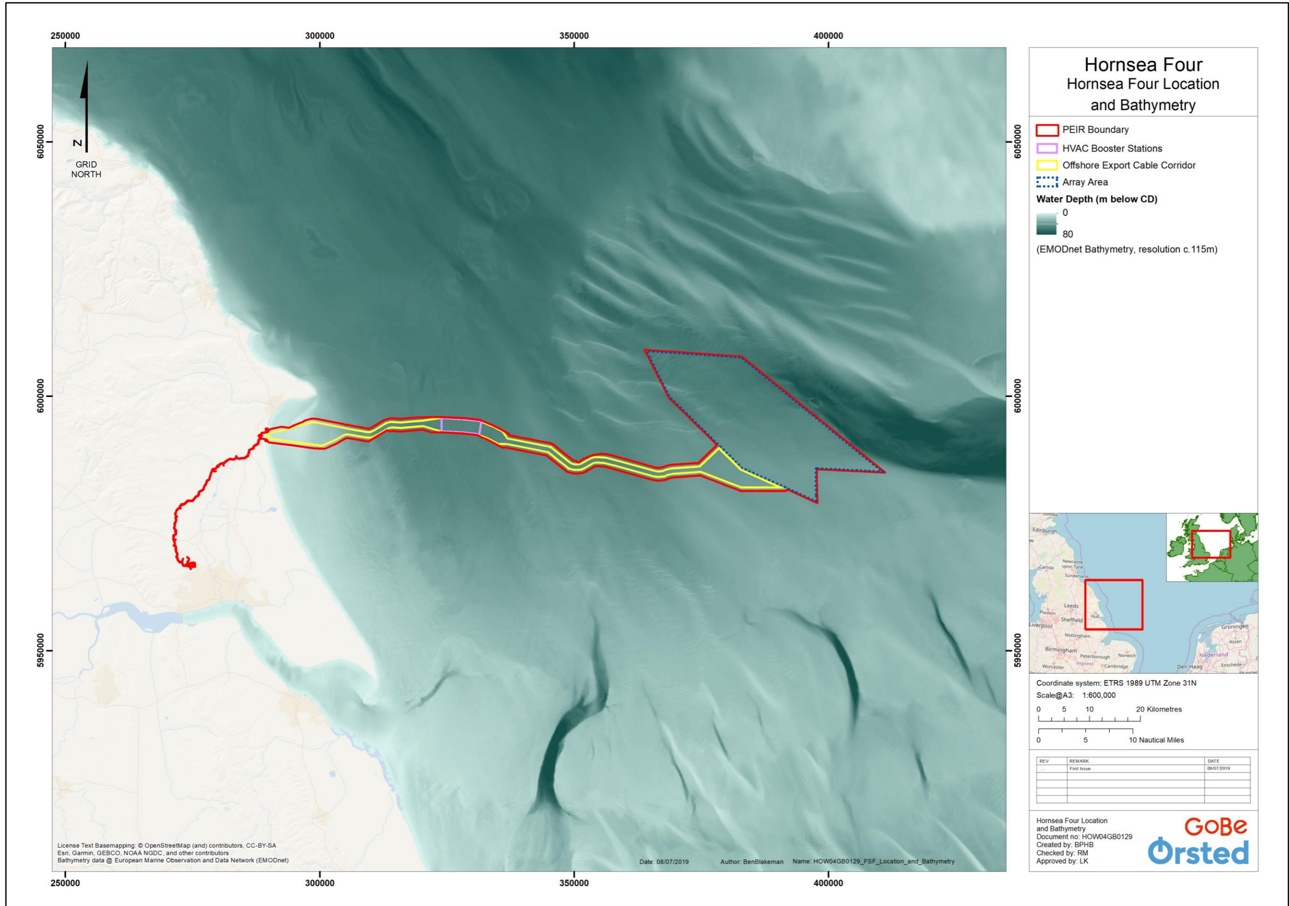
Figure 3.2: Bathymetry within the region of Hornsea Four (based on EMODnet bathymetry data) (not to scale).
