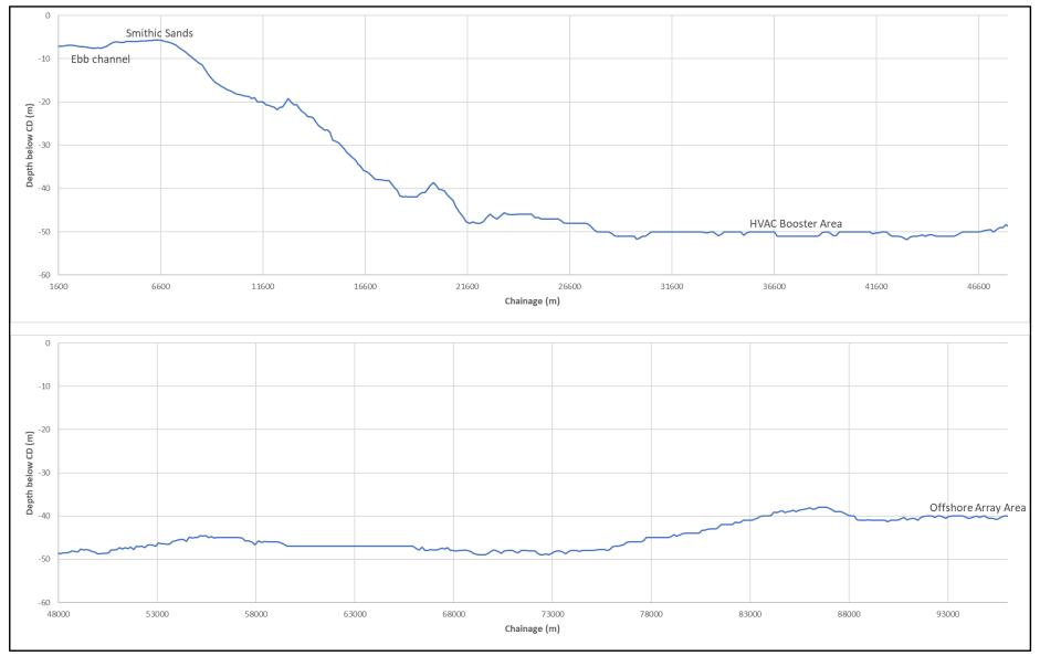
Figure 1.3: Seabed profile along offshore ECC, from landfall into offshore array.
