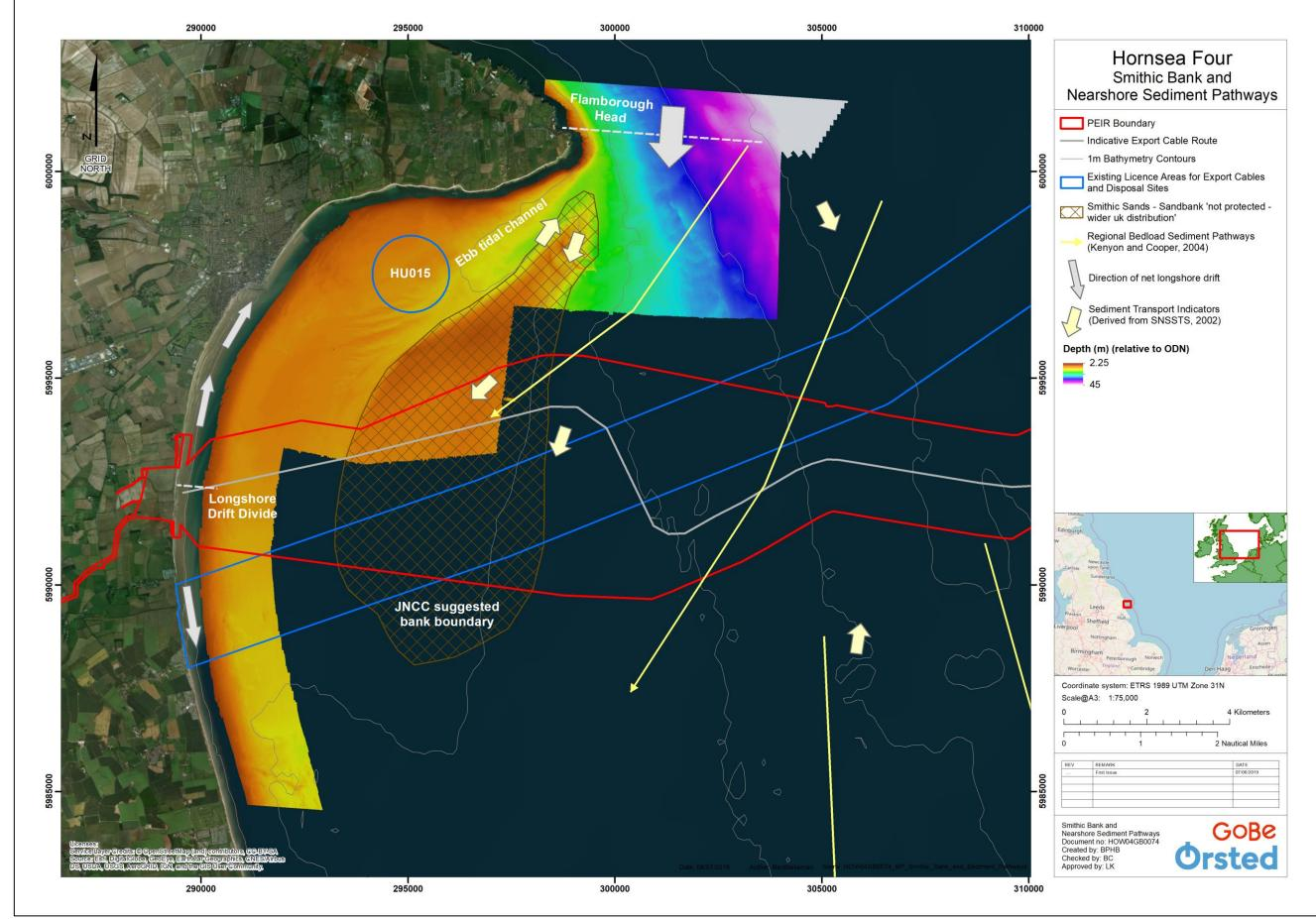
Figure 1.10: Smithic Sands and nearshore sediment pathways (not to scale).
