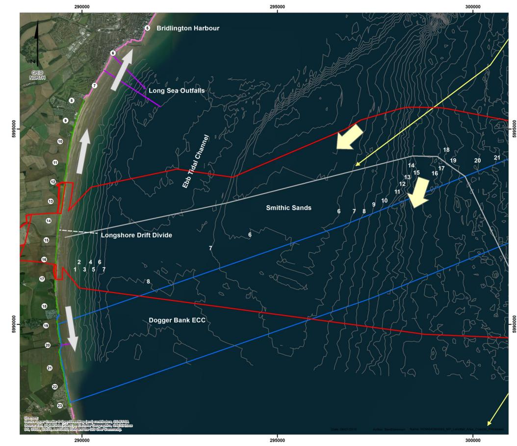
Figure 1.2: Landfall area coastal process (not to scale).
