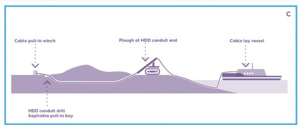
Figure 4.14: Indicative HDD and open cut arrangement (indicative only).
