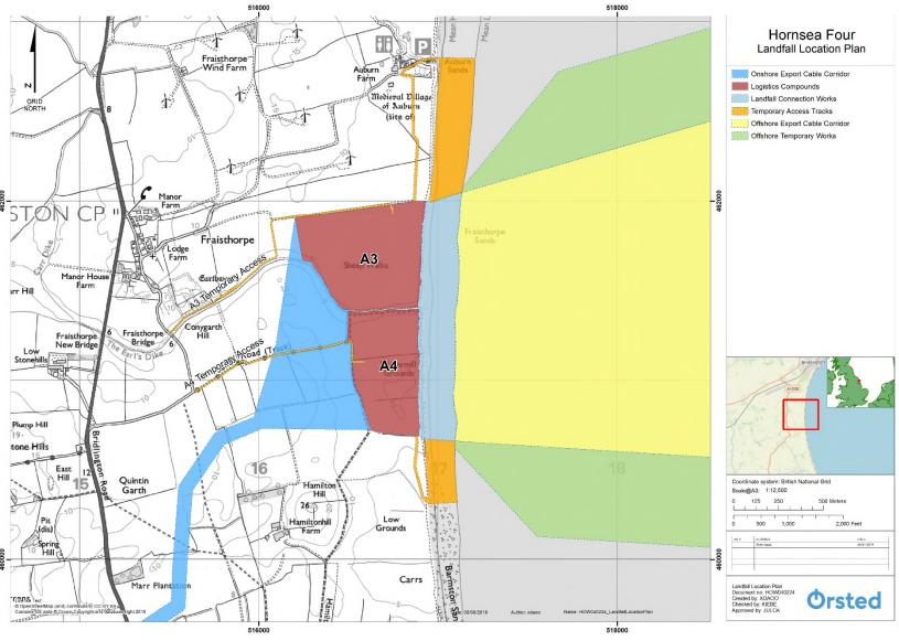
Figure 4.13: Hornsea Four Landfall Area. Two different options for the Export cable corridor through the landfall area (not to scale).
