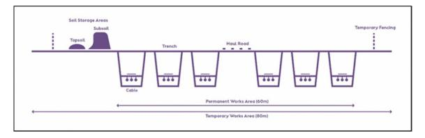
Figure 4.18: Onshore export cable corridor indicative layout showing the maximum of 6 onshore circuits (indicative only).
