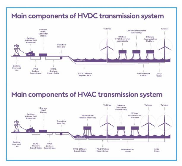
Figure 4.3: Main components of Hornsea Four (indicative only).
