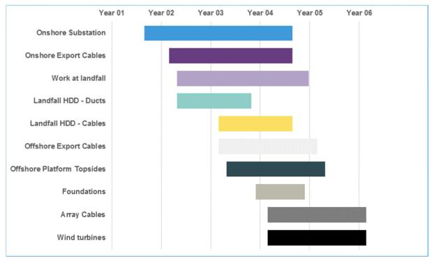
Figure 4.4: Indicative construction programme for Hornsea Four.
