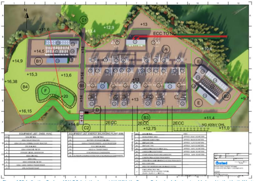
Figure 4.20: Indicative Onshore HVAC Substation layout (A). With the Energy Balancing Infrastructure(s) placed to the North-West (B1) and to the East (B2) on the figure (not to scale).
