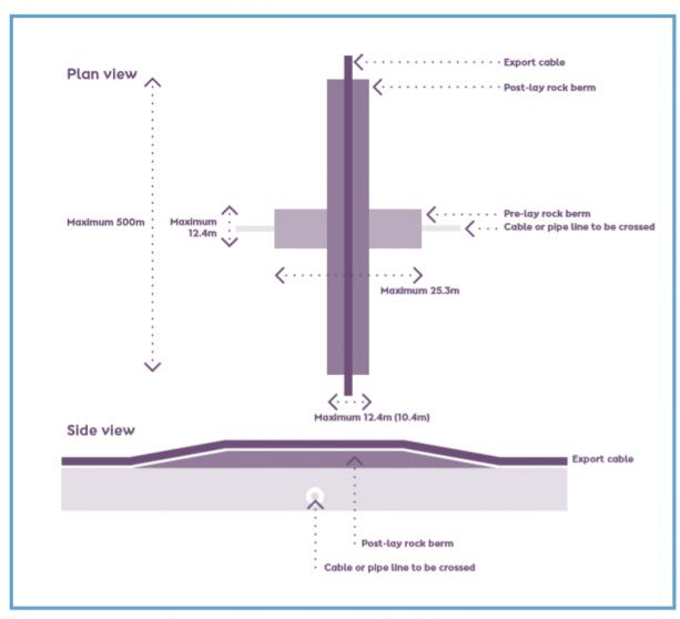
Figure 4.11: Offshore Cable Crossing (indicative only).
