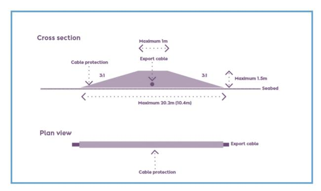
Figure 4.10: Cable protection via rock placement (indicative only).
