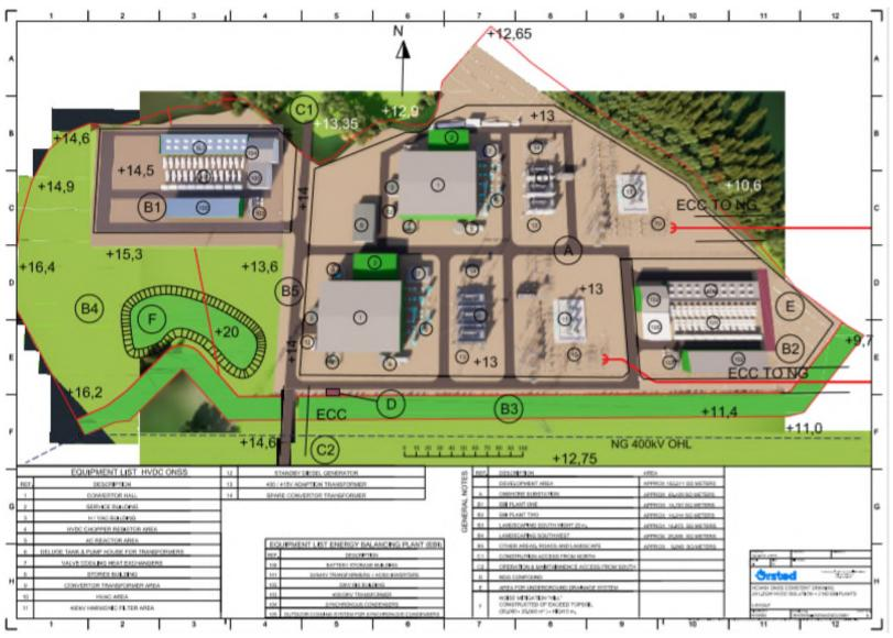
Figure 4.21: Indicative Onshore HVDC converter substation layout (A). With the Energy Balancing Infrastructure(s) placed to the North-West (B1) and to the East (B2) in the figure (not to scale).
