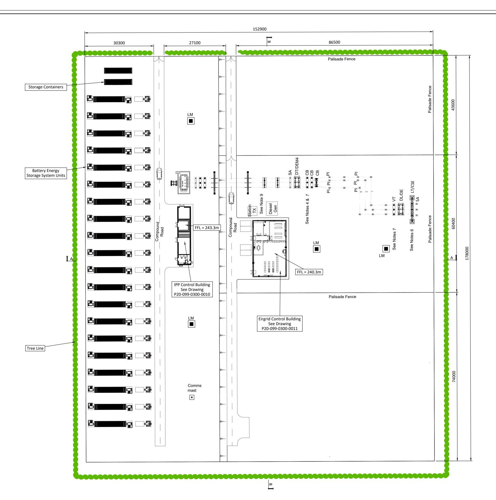
Legend LIGHTING MAST SURGE ARRESTER VOLTAGE TRANSFORMER CURRENT TRANSFORMER, SINGLE PHASE POST INSULATOR LINE TRAP (TYPICALLY R & T PHASES) LINE/EARTH DISCONNECT DL/DE DT/DEM4 TRAFO/EARTH DISCONNECT CIRCUIT BRAKER BUSBAR DISCONNECT DB SA1/SA2 SB1/SB2 SECTIONALISER DISCONNECT
