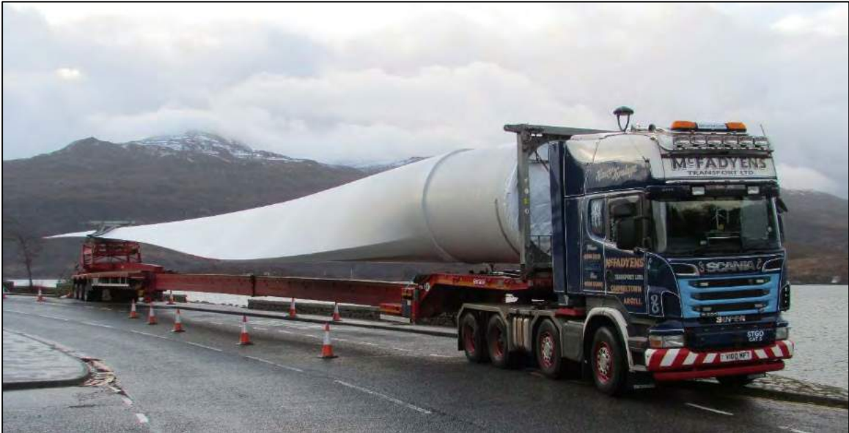
Figure 2: Superwing Carrier Trailer
