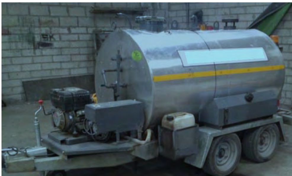
Plate 3-5: Towable Sprayer for Temporary Reinstatement
